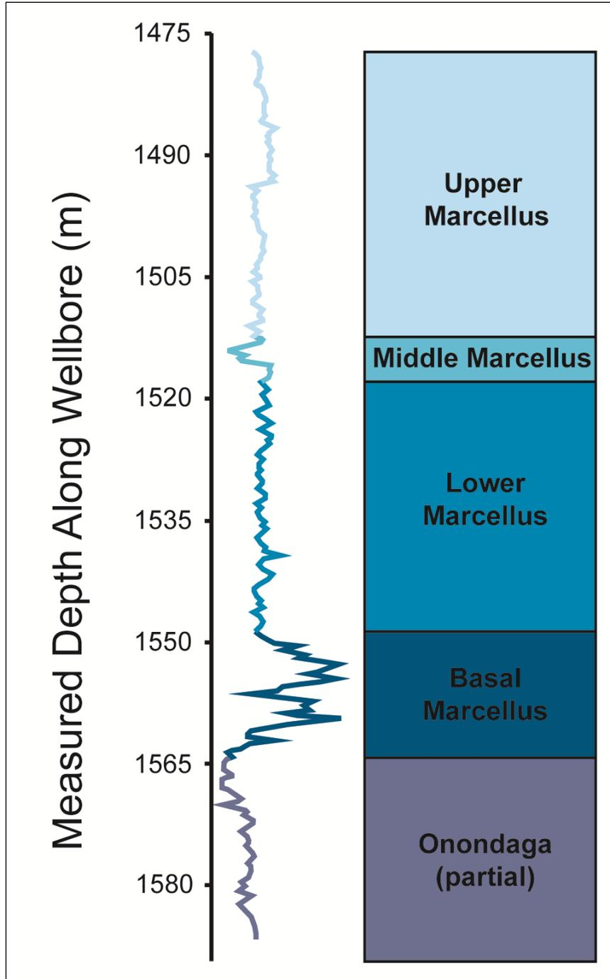
**Figure 6:** Vertical gamma type log for the Appalachian Plateau. This guide shows the gamma log signatures for specific units. The gamma log signature recorded while horizontally drilling is compared to this type log to understand what section the wellbore is currently in stratigraphically.
