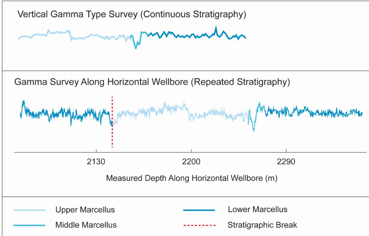
**Figure 9:** Comparing the vertical gamma type survey for the Appalachian Plateau (modified from Figure 6) to a horizontal well path. The horizontal well path passed through upper Marcellus shale into lower Marcellus shale with no record of middle Marcellus.
