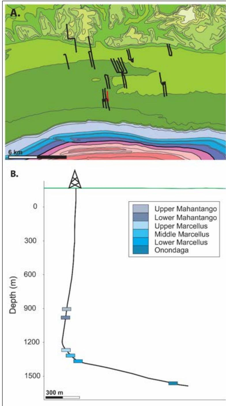
**Figure 5:** (A) The plan view extent of vertical and horizontal wells drilled by Inflection Energy, LLC. in Lycoming County, Pennsylvania. Refer to figure 4 for legend. (B) Horizon top data along one well path (represented by red well path in (A)) drilled by Inflection Energy, LLC. This data reveals the depth to horizons in the area of this specific well.
