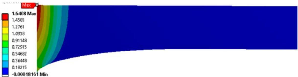
Figure 85: Normal radial stress (MPa) plot for minor radius 8mm
