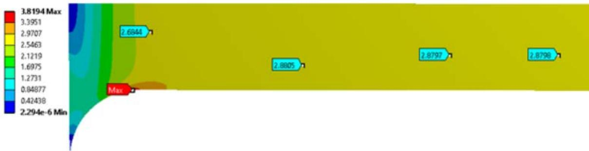
Figure 53: von Mises stress (MPa) plot for a fillet radius of 4mm
