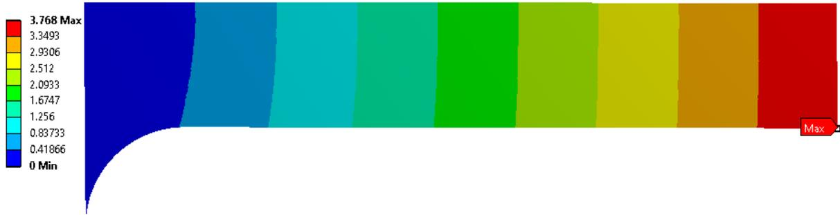
Figure 110: Displacement (mm) plot for mesh size 0.25
