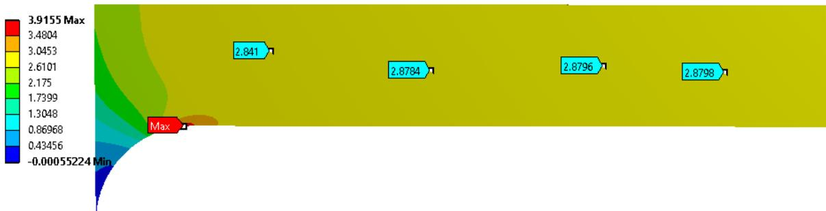
Figure 104: Normal axial stress (MPa) plot for mesh size 0.09
