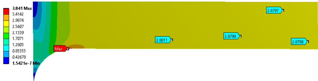
Figure 107: Equivalent stress (MPa) plot for mesh size 0.07
