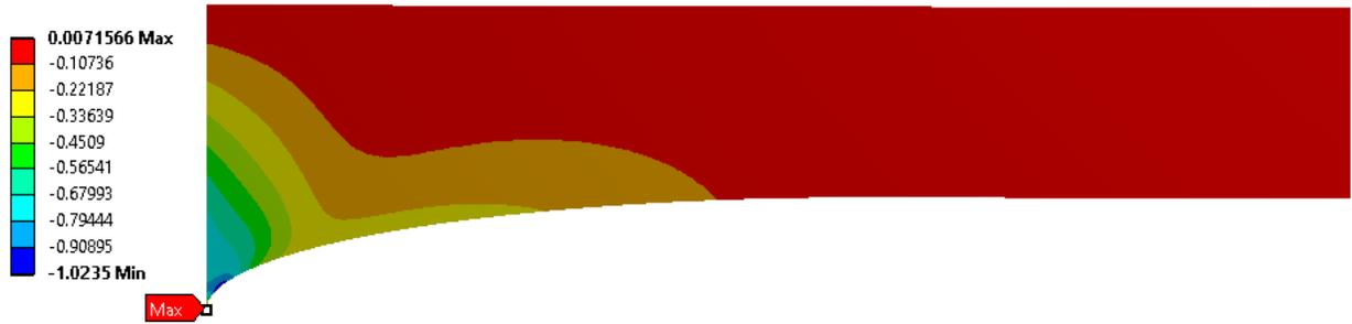
Figure 86: Shear stress (MPa) plot for minor radius 8mm
