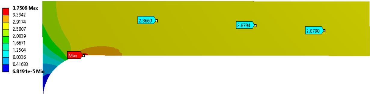
Figure 112: Normal axial stress (MPa) plot for mesh size 0.25
