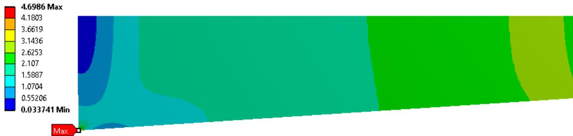
Figure 99: Equivalent stress (MPa) plot for mesh size 0.25
