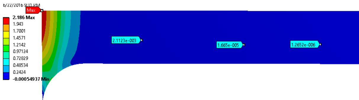
Figure 105: Normal radial stress (MPa) plot for mesh size 0.09
