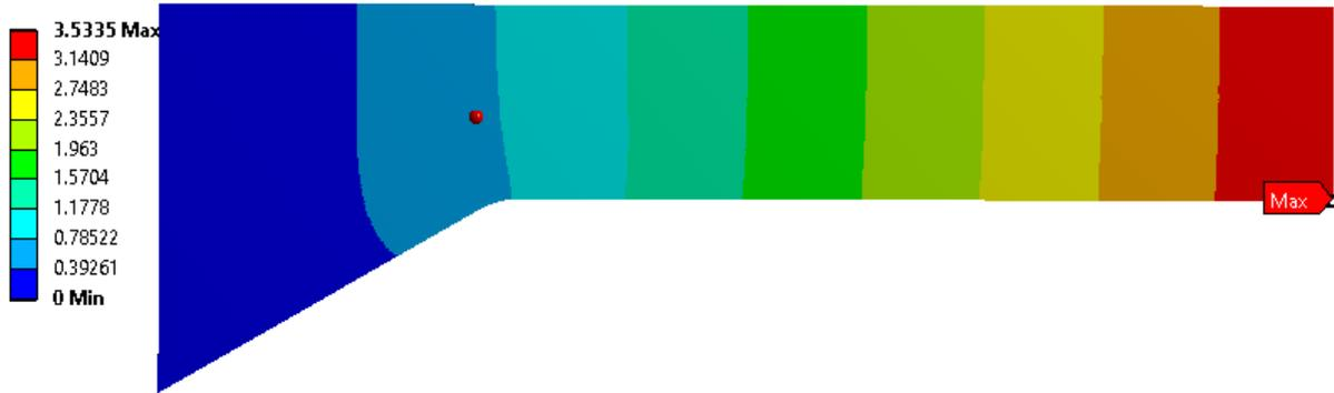
Figure 122: Displacement (mm) plot for mesh size 0.07
