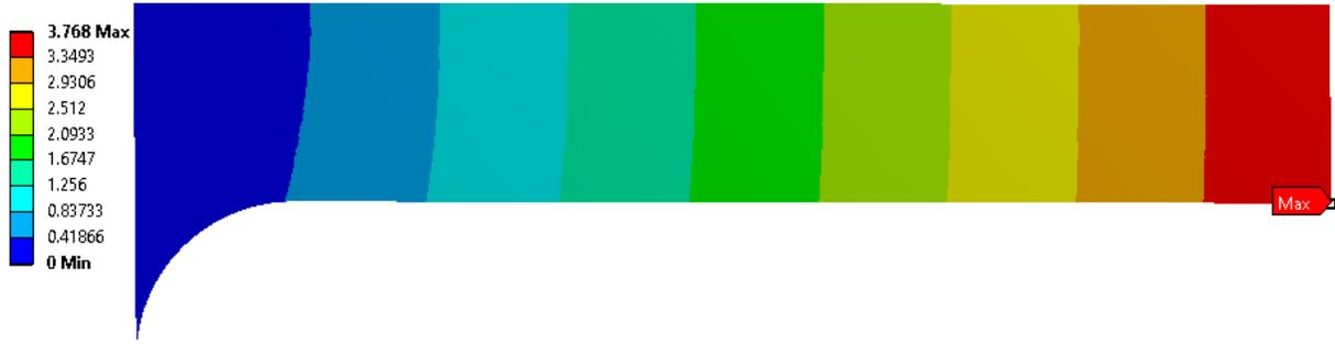
Figure 102 Displacement (mm) plot for mesh size 0.09
