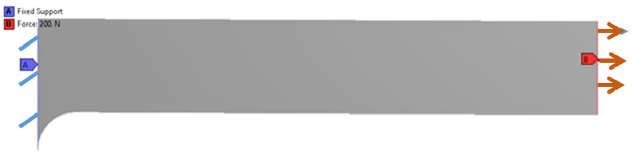
Figure 46: Case III with fillet radius 1mm
