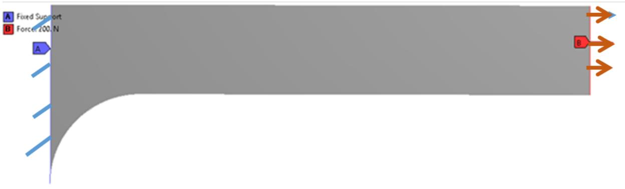
Figure 47: Case III with fillet radius 5mm
