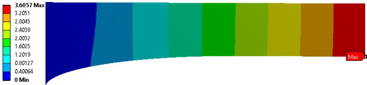
Figure 126 : Displacement (mm) plot for mesh size 0.09
