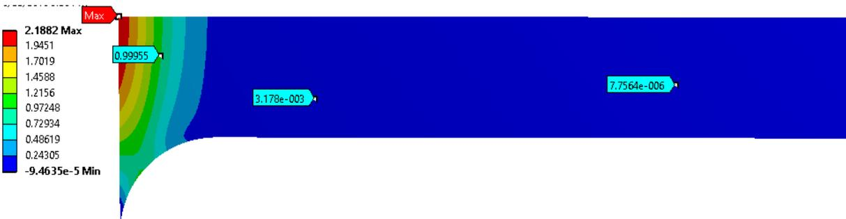
Figure 109: Normal radial stress (MPa) plot for mesh size 0.07
