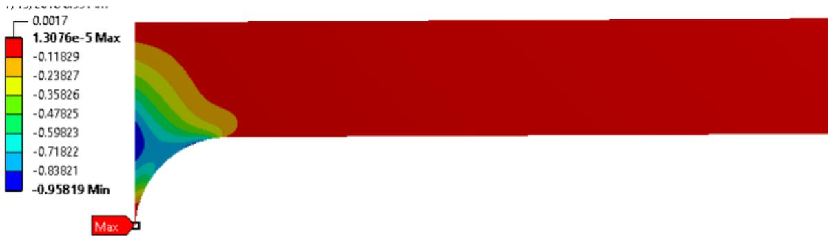
Figure 56: Shear stress (MPa) plot for a fillet radius of 4mm
