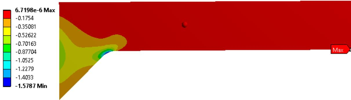
Figure 71: Shear stress (MPa) plot for case IV (angle 45 deg.)
