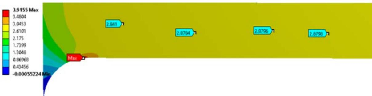
Figure 54: Normal axial stress (MPa) plot for a fillet radius of 4mm
