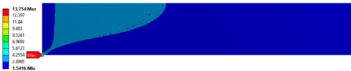
Figure 24: Normal axial stress (MPa) plot for Case I (Diameter 10mm)
