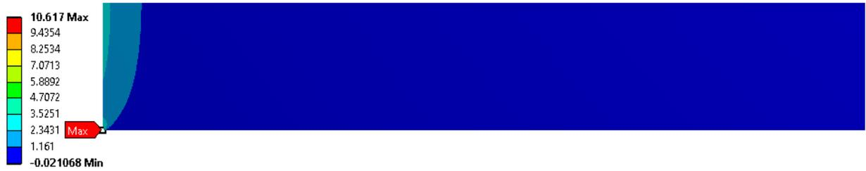
Figure 25: Normal radial stress (MPa) plot for Case I (Diameter 10mm)
