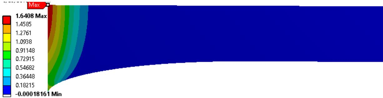
Figure 129: Normal radial stress (MPa) plot for mesh size 0.09
