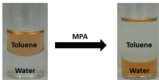
Figure 1.10 - ODPA capped CdTe nanoparticles soluble in toluene (left vial). Following ligand exchange to MPA, the nanoparticles change phases to become soluble in water (right vial). 51
