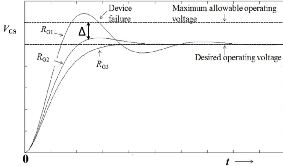
**Figure 10.** Commonly observed turn on characteristics for a generic device, where  $R_{G1} < R_{G2} < R_{G3}$
