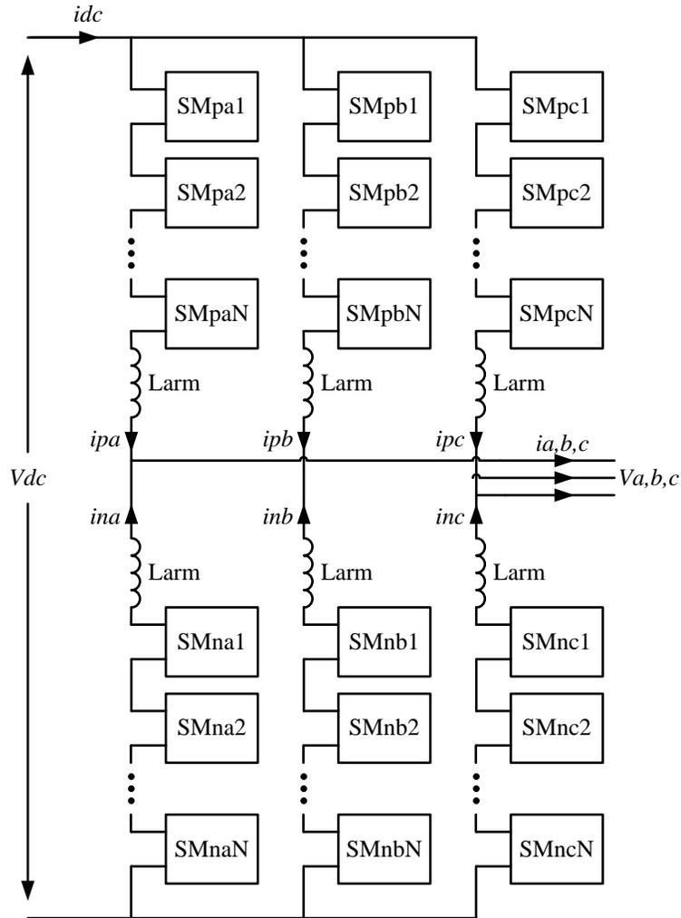
**Figure 4.** Three-phase modular multilevel converter topology
