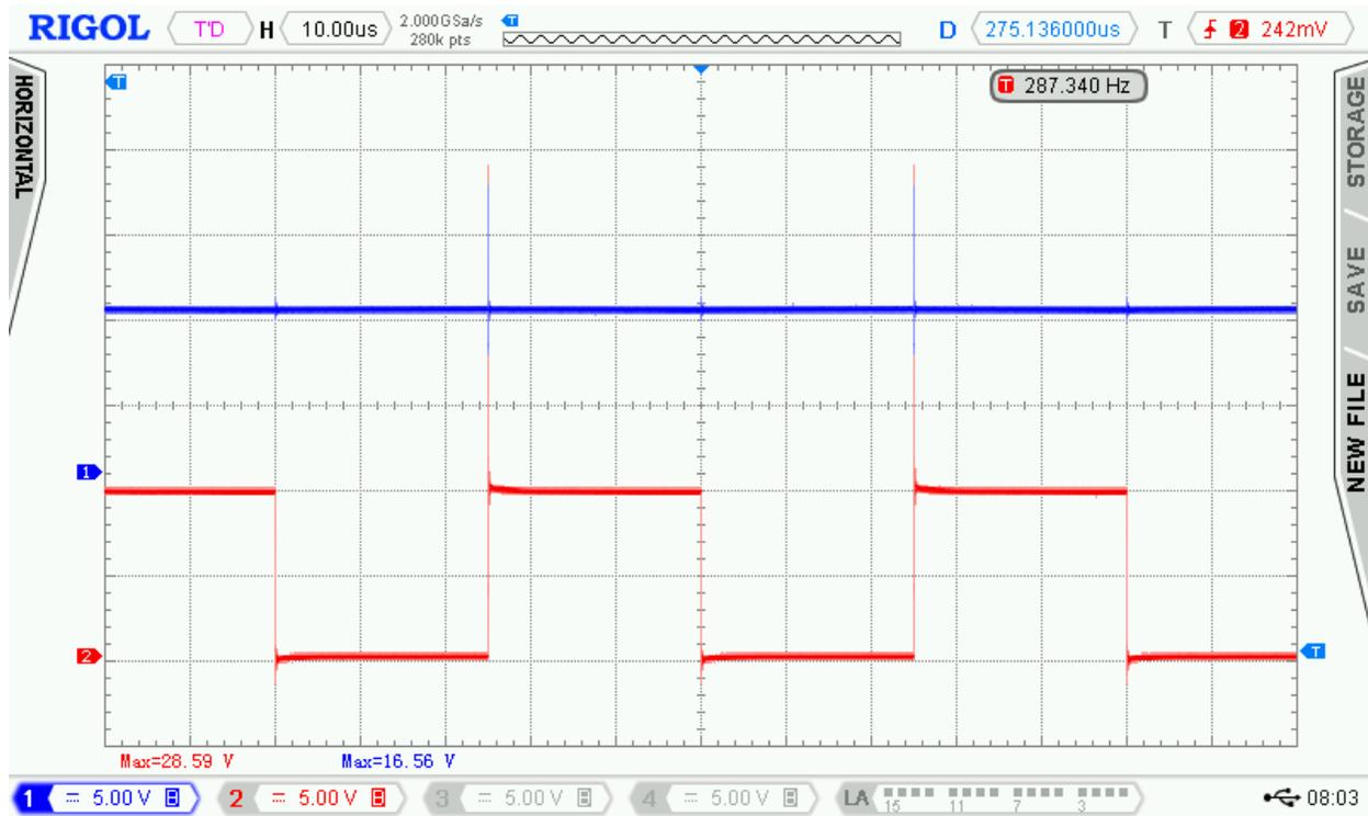
**Figure 81.** AC output of MHz range test converter at 10 V DC input
