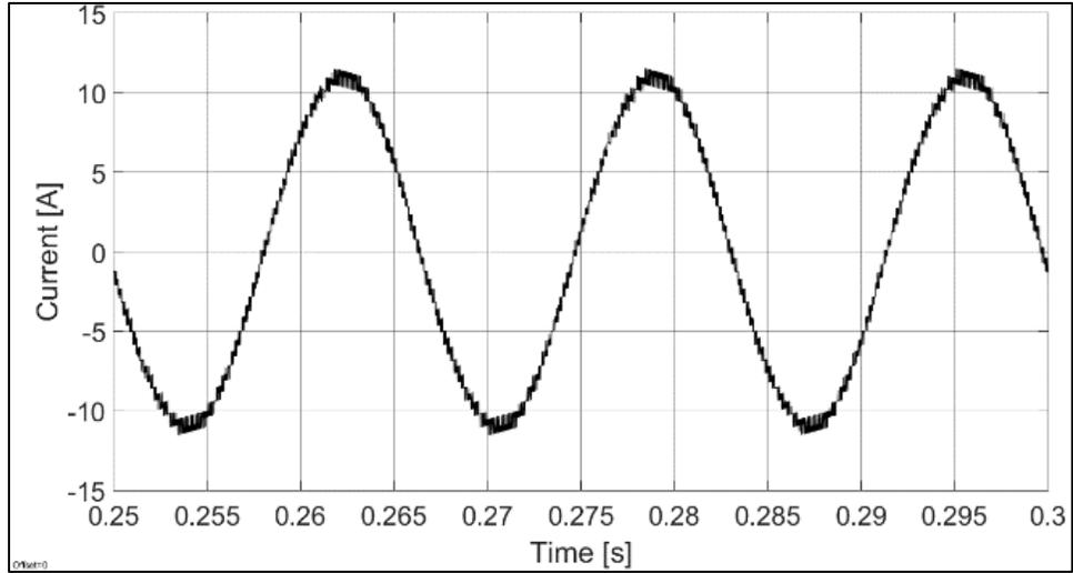
**Figure 43.** Simulated AC output current for 2 kW DC-AC MMC
