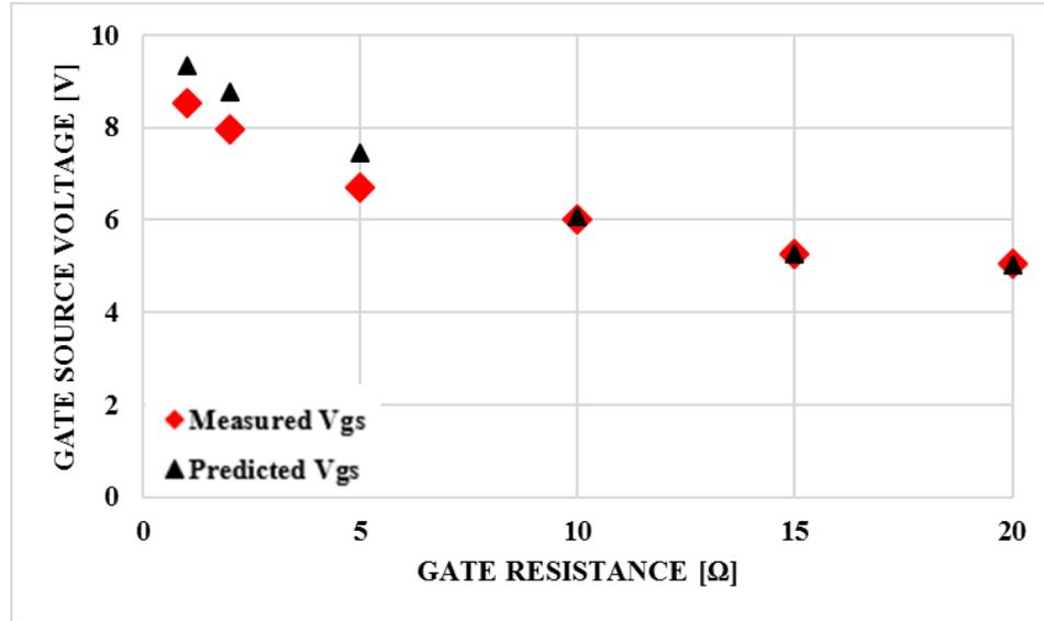
**Figure 20.** Predicted and measured values for  $v_{GS}$  vs  $R_G$
