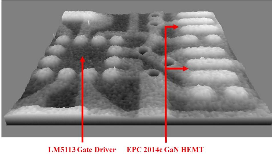
**Figure 59.** X-Ray Image of LM5113 Gate Driver and EPC2014c GaN HEMTs
