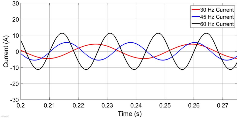
**Figure 46.** Motor input current from the DC-AC MMC variable speed drive
