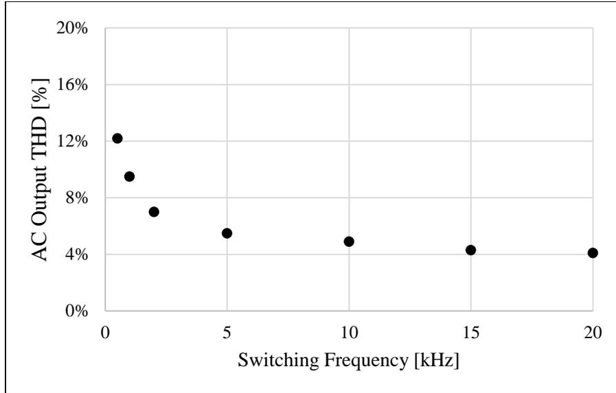
**Figure 40.** AC output THD as a function of switching frequency
