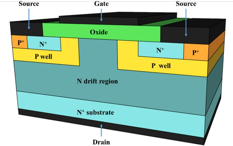
**Figure 5.** Device structure for a vertical SiC MOSFET
