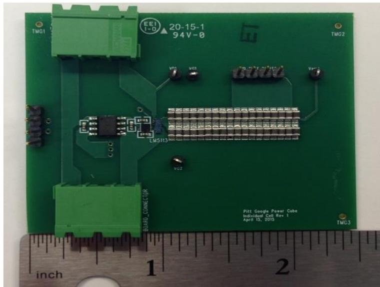
**Figure 50.** PCB design of a single half-bridge submodule
