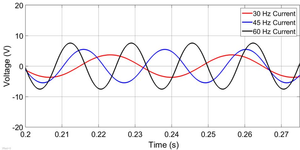
**Figure 47.** Motor load current from the DC-AC MMC variable speed drive
