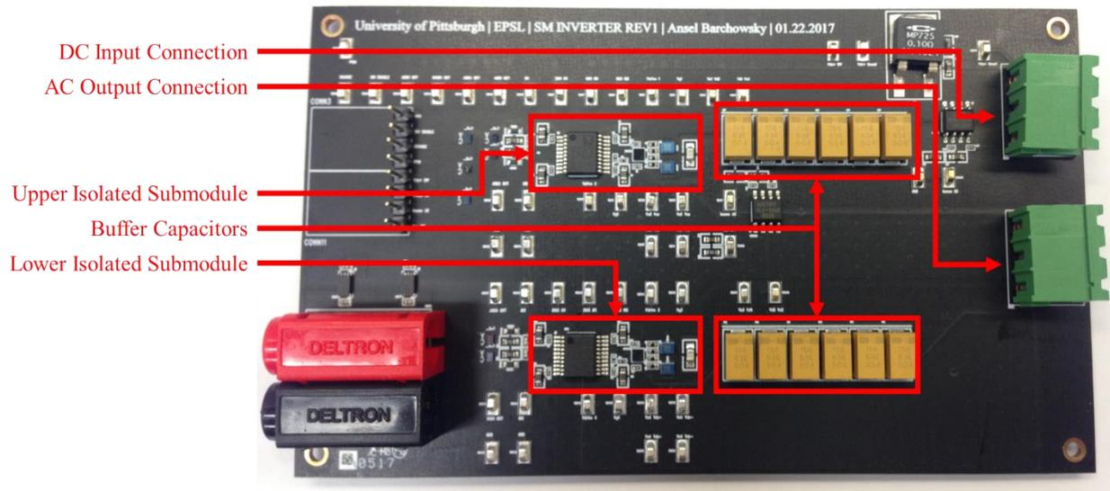
**Figure 80.** Annotated PCB layout of two-level isolated test system
