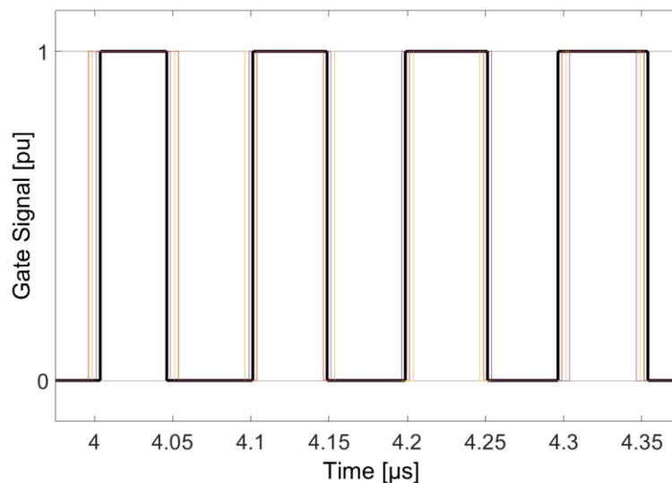
**Figure 66.** Progressive insertion method for voltage balancing between submodules
