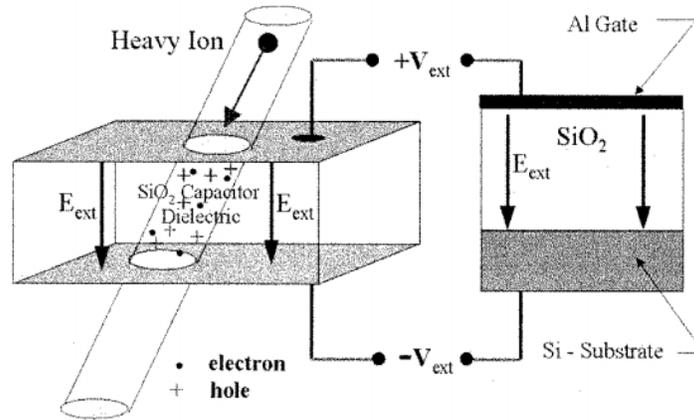
Figure 75. Generation of electron-hole pairs in an oxide following heavy-Ion strike
