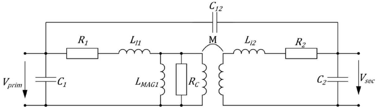
**Figure 35.** Equivalent circuit model for planar transformer
