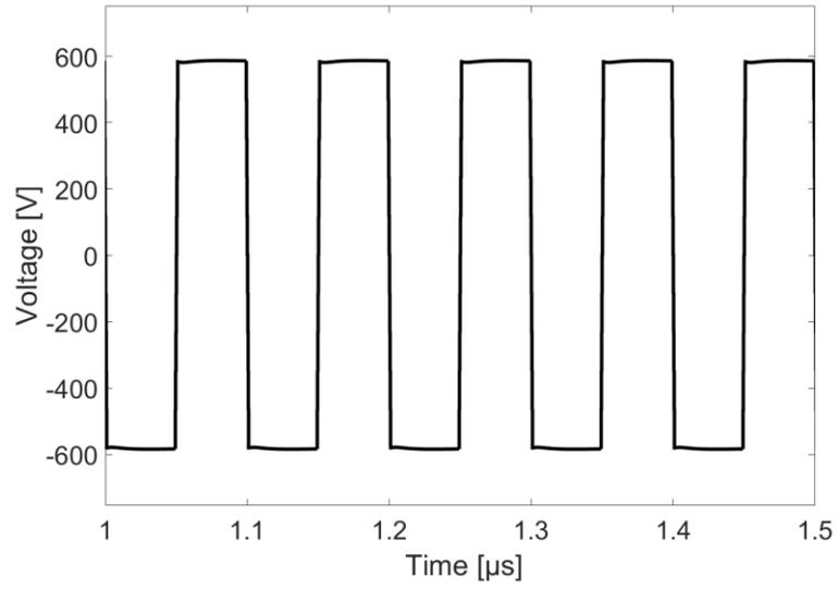
**Figure 69.** Voltage on secondary side of DC-DC MMC AC link
