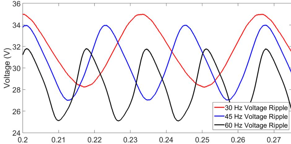
**Figure 48.** Voltage ripple on the SM capacitors of the DC-AC MMC variable speed drive
