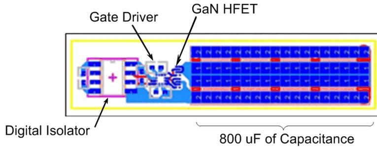
**Figure 49.** Printed circuit board design for one half-bridge submodule
