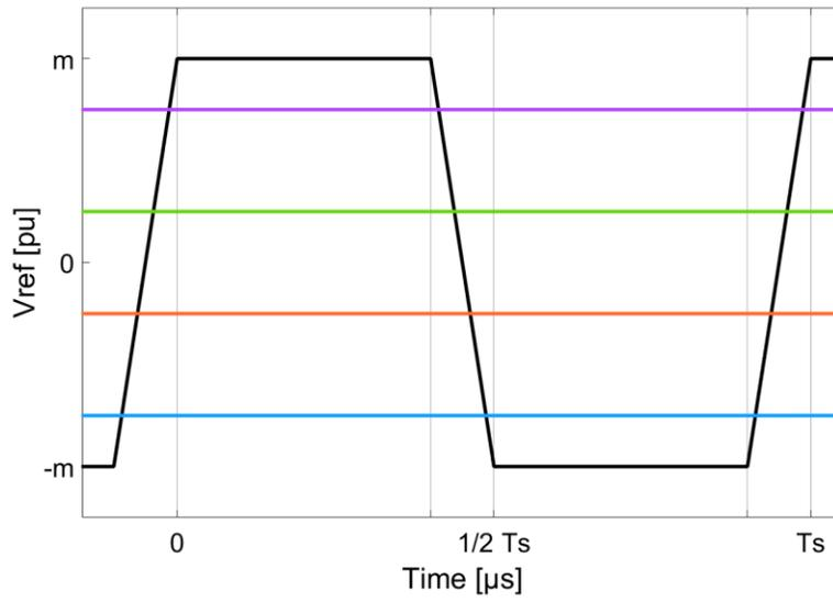
**Figure 64.** QSW reference and NLM carrier waveforms
