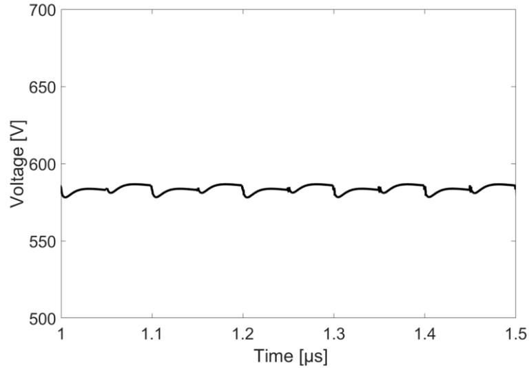
**Figure 71.** Voltage on DC-DC MMC output
