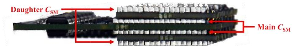
**Figure 57.** Side view of prototype MMC arm board
