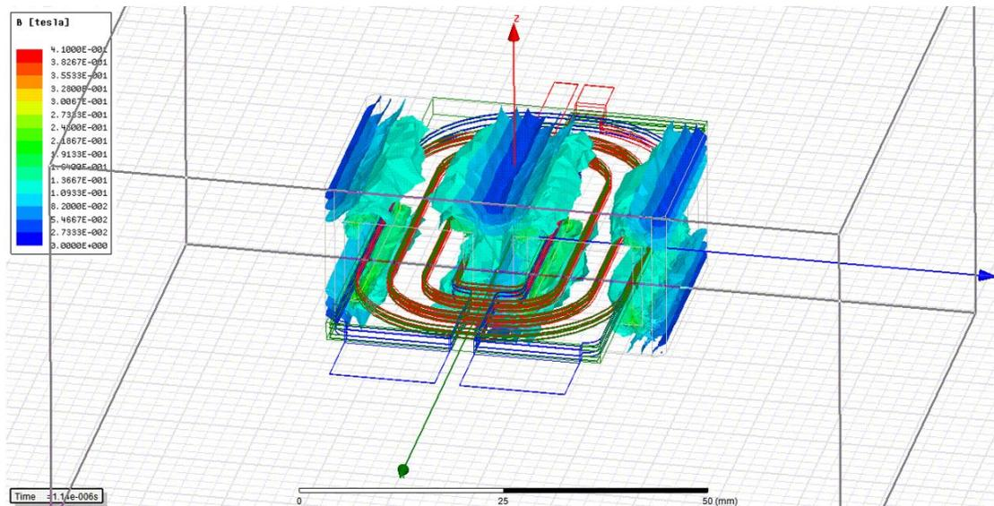
**Figure 33.** Lowest flux point in the core when excited by 200 V square wave
