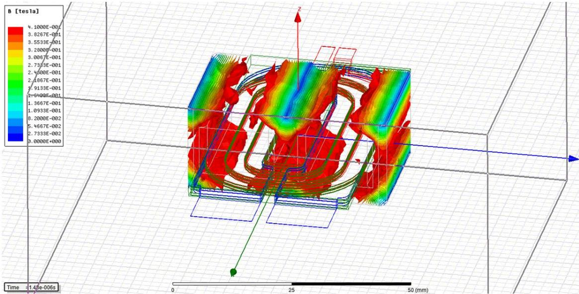
**Figure 32.** Highest flux point in the core when excited by 200 V square wave
