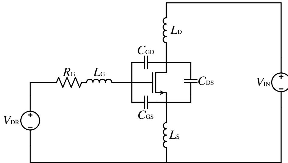
**Figure 9.** Circuit layout of a resistor-protected GaN HEMT illustrating device parasitics
