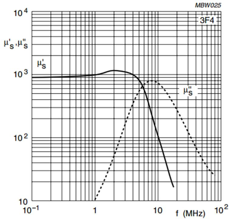
**Figure 8.** Complex permeability of Ferrocube 3F4 MnZn ferrite
