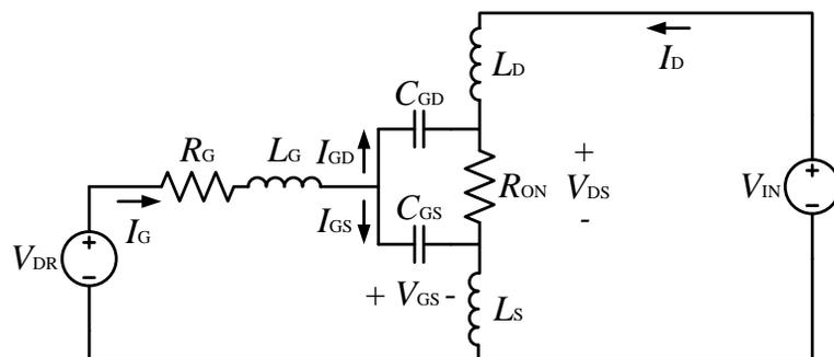
**Figure 13.** Equivalent circuit for sub-stage 3 of device turn on
