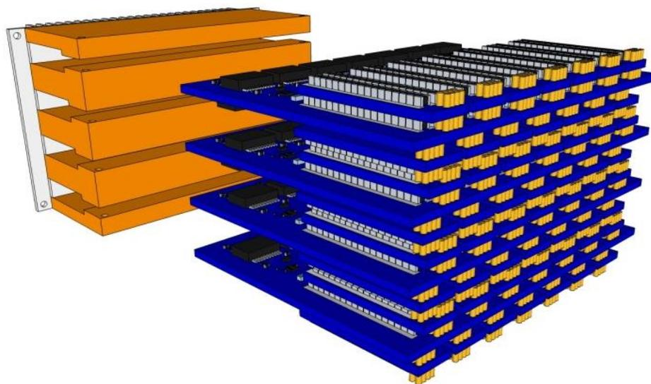
**Figure 58.** CAD Layout of full MMC Inverter with Heat Sink Design
