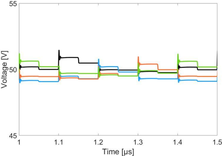
**Figure 73.** Capacitor voltage balancing in primary converter branch
