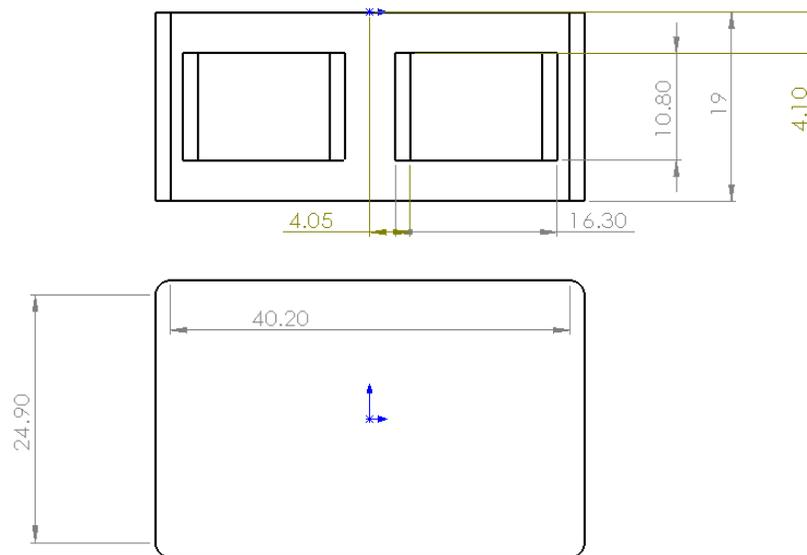
**Figure 26.** Solidworks drawing of paired E43/10/28 cores
