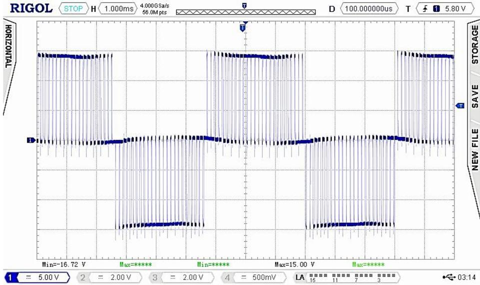
Figure 60. AC voltage output of prototype DC-AC MMC inverter
