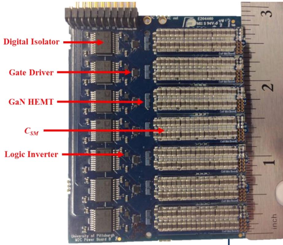
**Figure 56.** Top view of prototype MMC arm board
