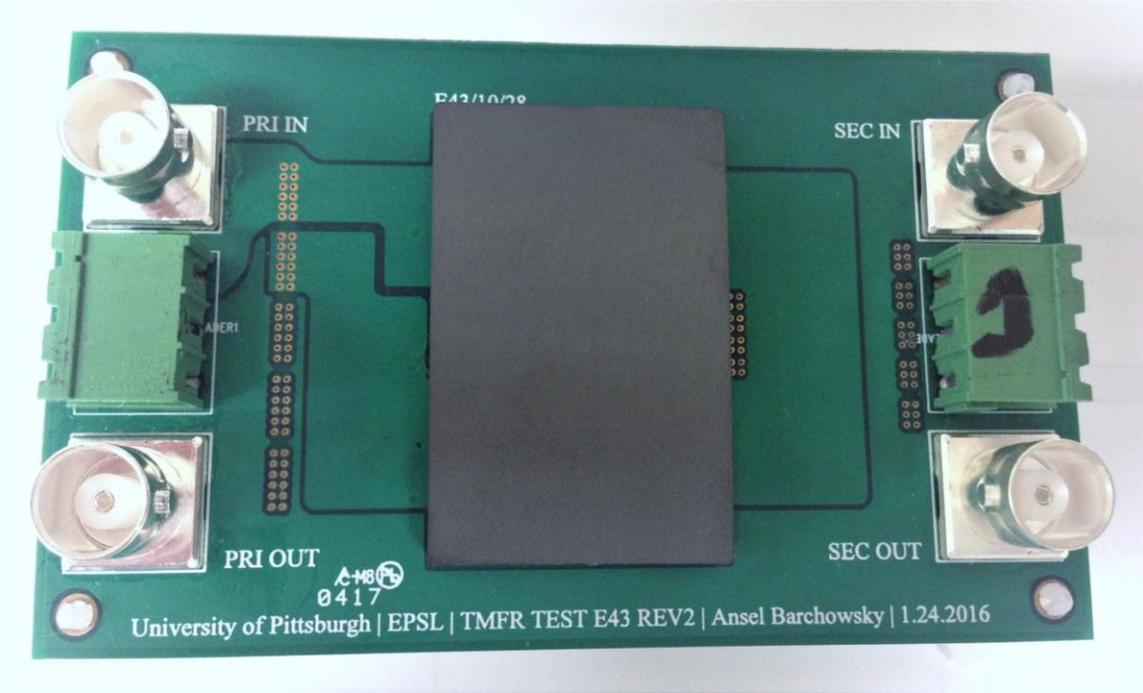
**Figure 36.** Prototype transformer PCB with layer-integrated windings
