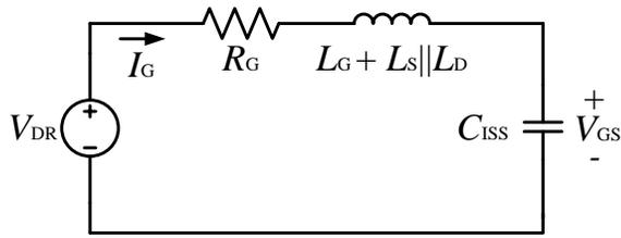
**Figure 11.** Equivalent circuit for sub-stage 1 of device turn on
