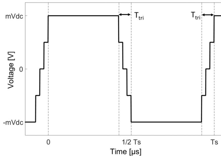
**Figure 65.** AC output from QSW NLM modulation
