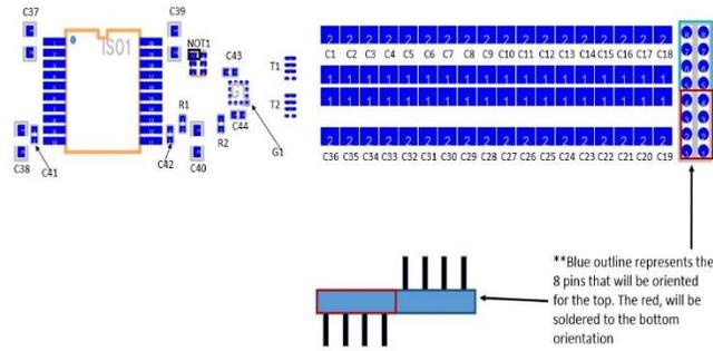
**Figure 55.** MMC full power board submodule with added standoffs for mezzanine capacitor boards
