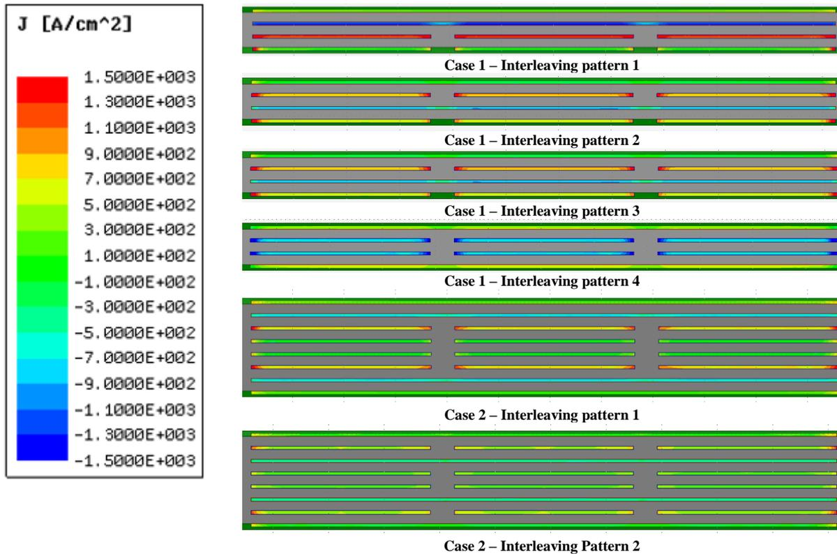
**Figure 23.** Current densities for various winding cases and interleaving patterns in  $A/cm^3$
