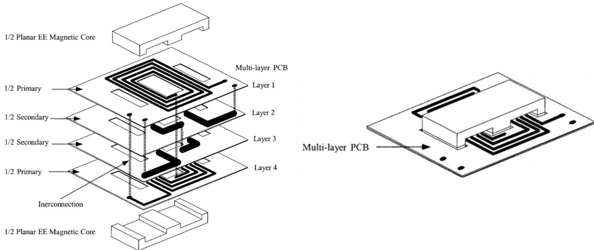
**Figure 21.** PCB integrated planar transformer [25]
