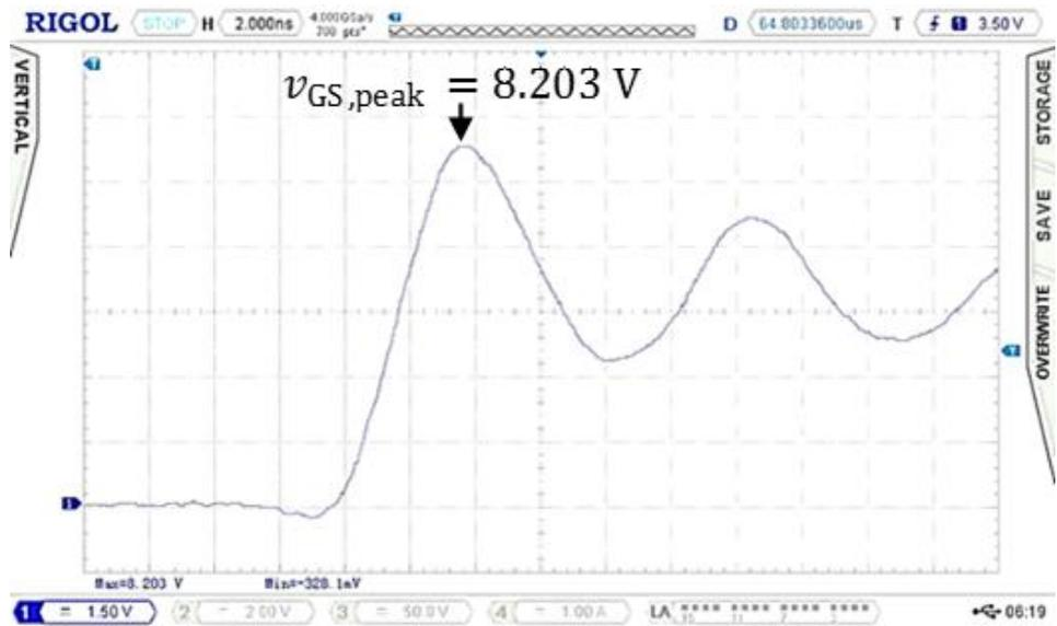
Figure 19. Turn-on of EPC8010 with  $R_G = 1 \Omega$
