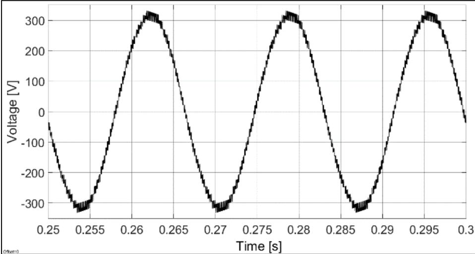
**Figure 42.** Simulated AC output voltage of 2 kW DC-AC MMC
