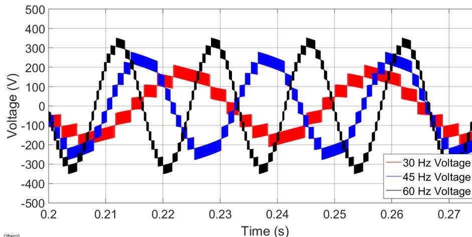
**Figure 45.** Line-to-line voltage output from the DC-AC MMC variable speed drive
