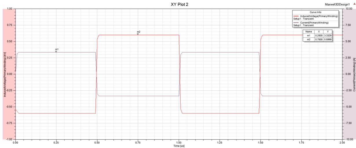
**Figure 31.** Secondary (high-voltage) voltage and current waveforms with 200 V square excitation and 2 kW resistive load
