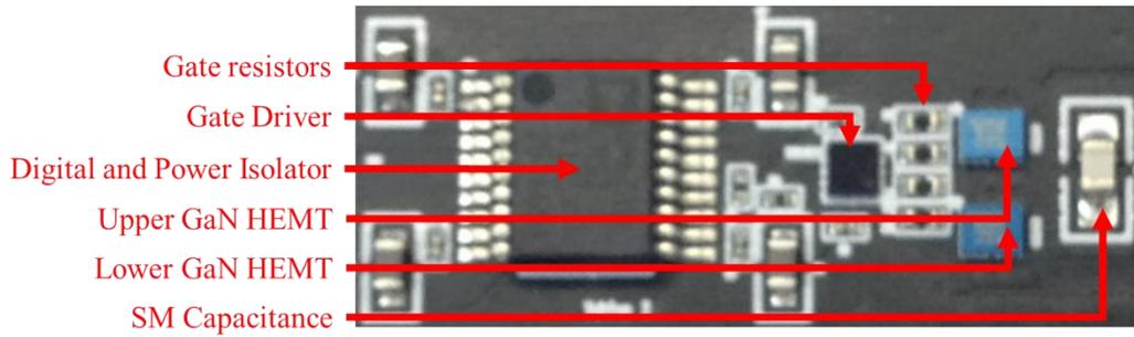
**Figure 79.** Isolated half-bridge PCB submodule layout
