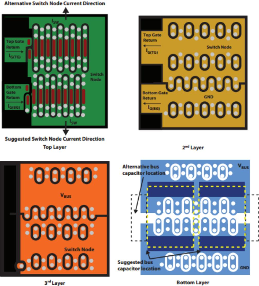
Figure 78. Recommended gate layout for GaN HEMT half-bridge from EPC
