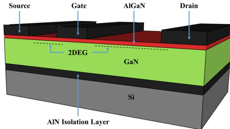
**Figure 6.** Device structure for a lateral GaN HEMT
