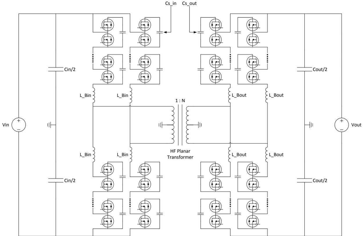
**Figure 63.** Proposed schematic of DC-DC MMC
