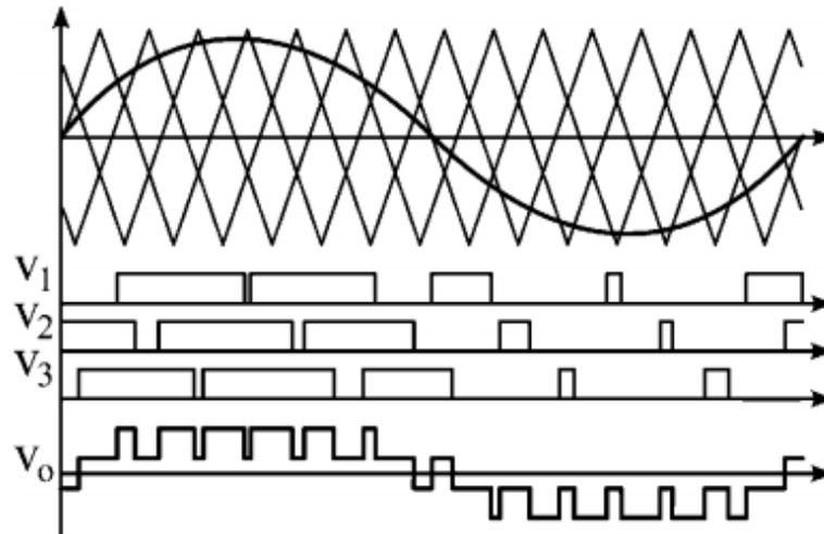
**Figure 38.** Phase shifted pulse width modulation signal generation and output
