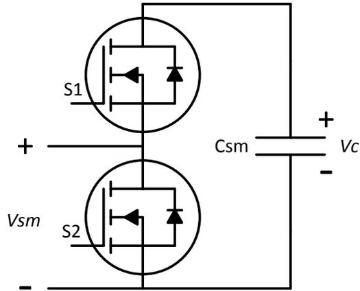
**Figure 1.** Half-bridge submodule for modular multilevel converter design
