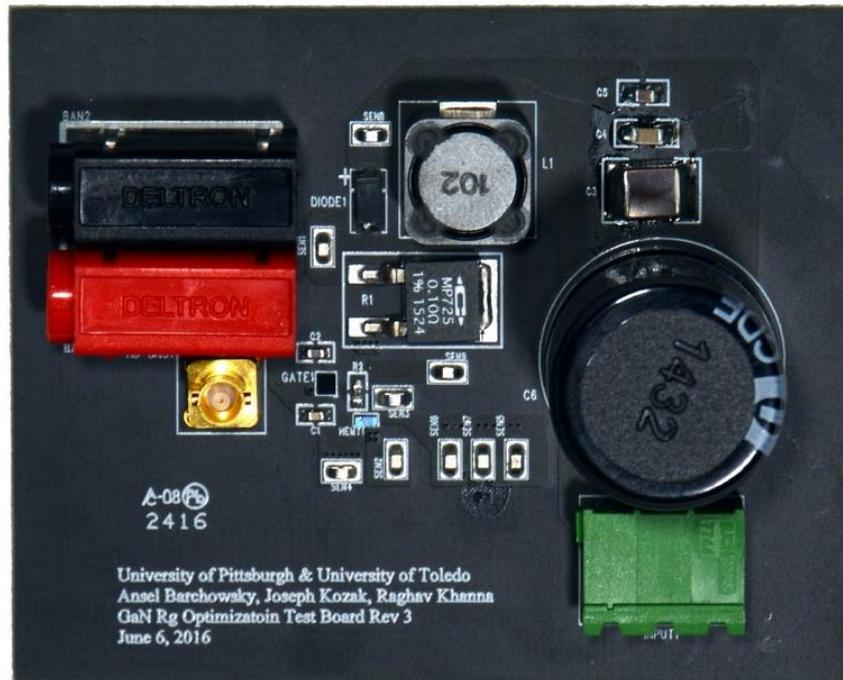
Figure 15. Double pulse test PCB for verification of  $R_G$  selection
