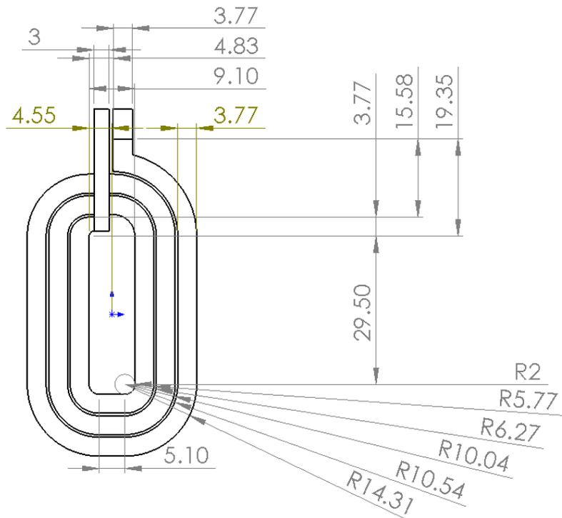
**Figure 25.** Solidworks drawing of transformer secondary winding
