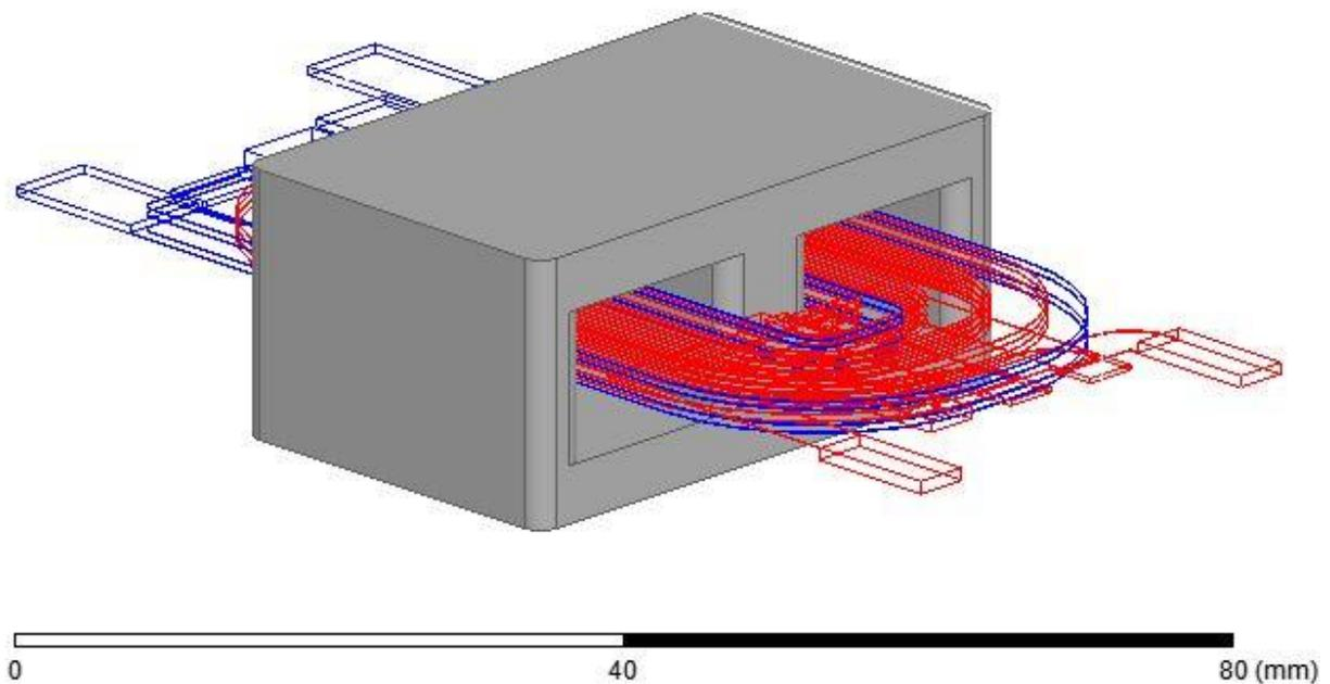
**Figure 34.** 3D model of planar transformer core with PCB integrated series windings
