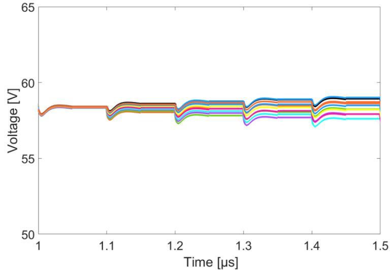
**Figure 74.** Capacitor voltage balancing in secondary converter branches
