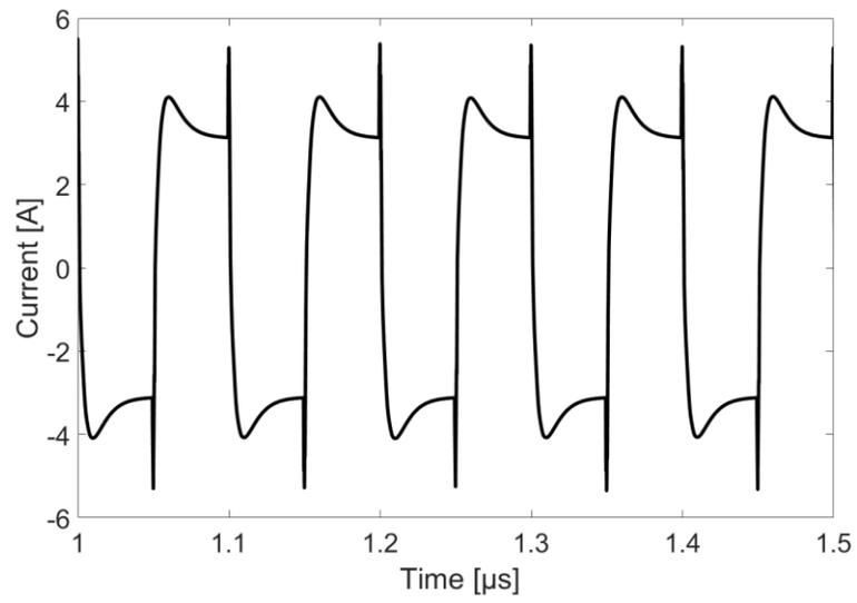
**Figure 70.** Current on secondary side of DC-DC MMC AC link
