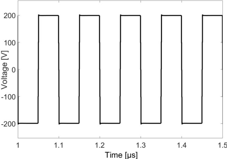
**Figure 67.** Voltage on primary side of DC-DC MMC AC link
