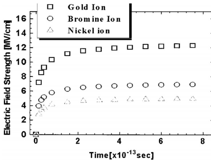
Figure 76. Buildup of the electric field strength versus time for the passage of an ion
