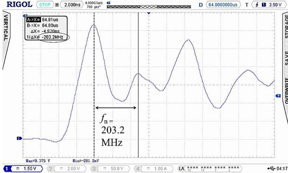
**Figure 16.** Un-damped measurement of  $v_{GS}$  vs  $t$  for calculation of  $L_{eq}$
