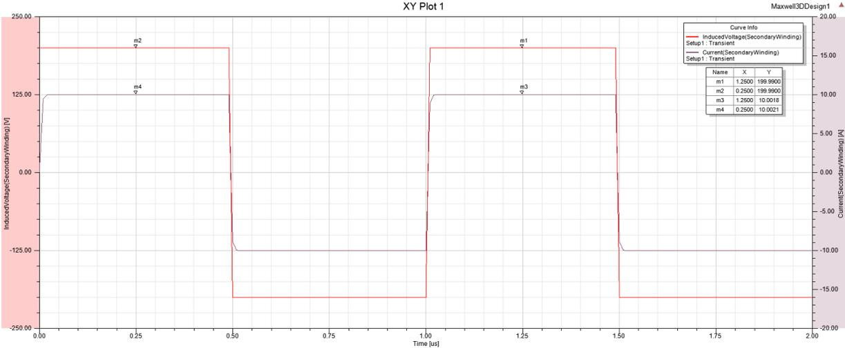
**Figure 30.** Primary (low-voltage) voltage and current waveforms with 200 V square excitation and 2 kW resistive load
