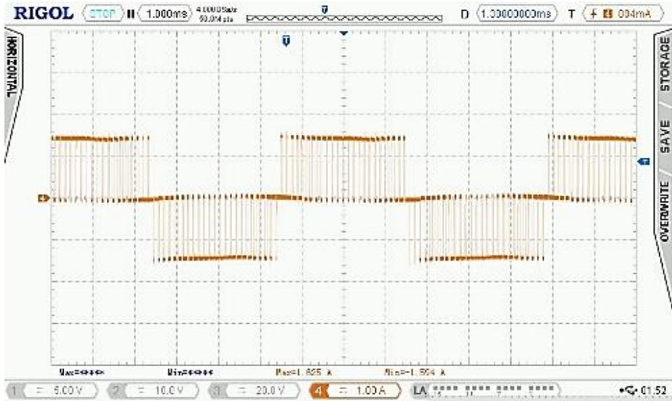
Figure 61. AC current output of prototype DC-AC MMC inverter
