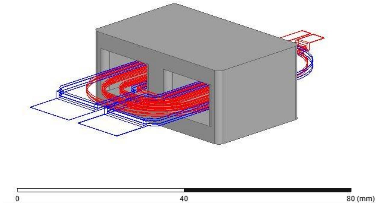
**Figure 27.** 3D model of planar transformer core with PCB integrated parallel windings
