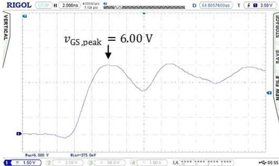
**Figure 17.** Turn on of EPC8010 with  $R_G = 10 \Omega$
