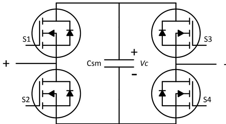
**Figure 2.** Full bridge submodule for modular multilevel converter design
