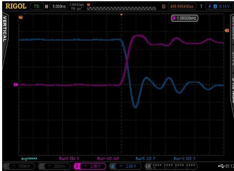
**Figure 53.** Measured turn OFF (ON) characteristic of upper (lower) transistors
