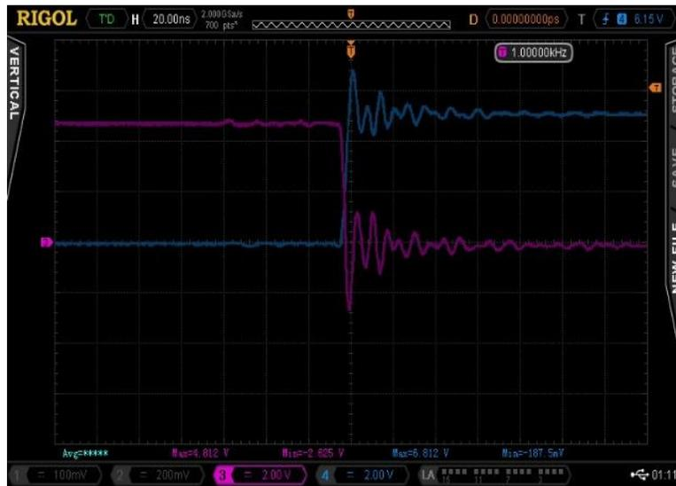
**Figure 52.** Measured turn ON (OFF) characteristics of upper (lower) transistors
