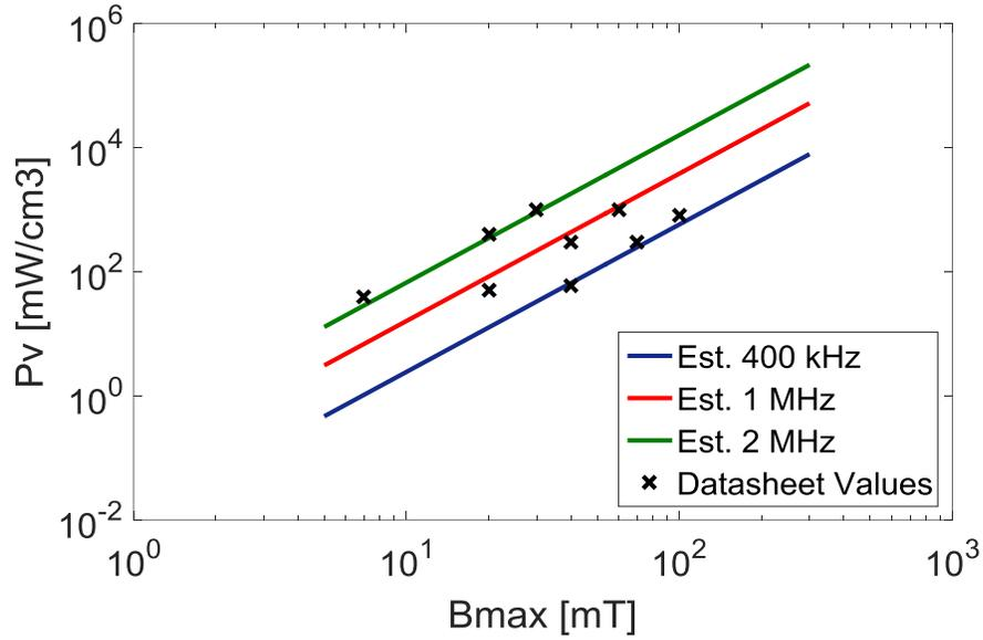
**Figure 22.** Matched core loss data for Ferroxcube 3F4 MnZn ferrite
