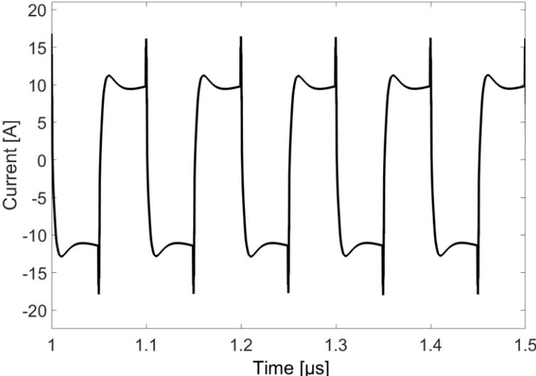
**Figure 68.** Current on primary side of DC-DC MMC AC link
