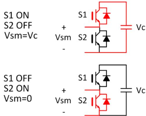
**Figure 3.** Switching states of a half-bridge modular multilevel converter submodule
