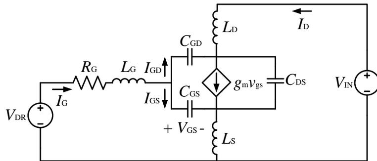
**Figure 12.** Equivalent circuit for sub-stage 2 of device turn on
