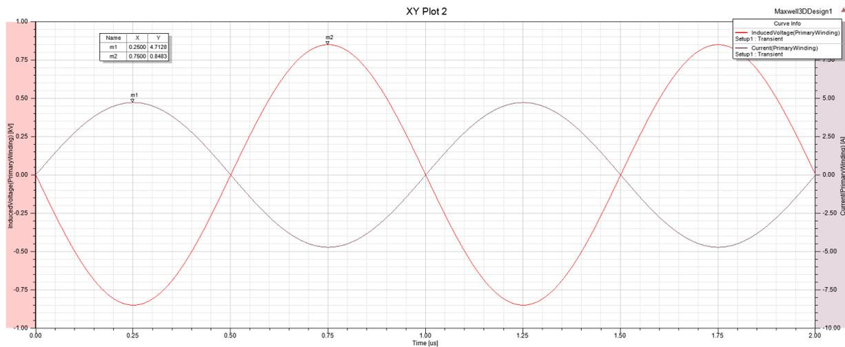
**Figure 29.** Secondary (high-voltage) voltage and current waveforms with 200 V sinusoidal excitation and 2 kW resistive load
