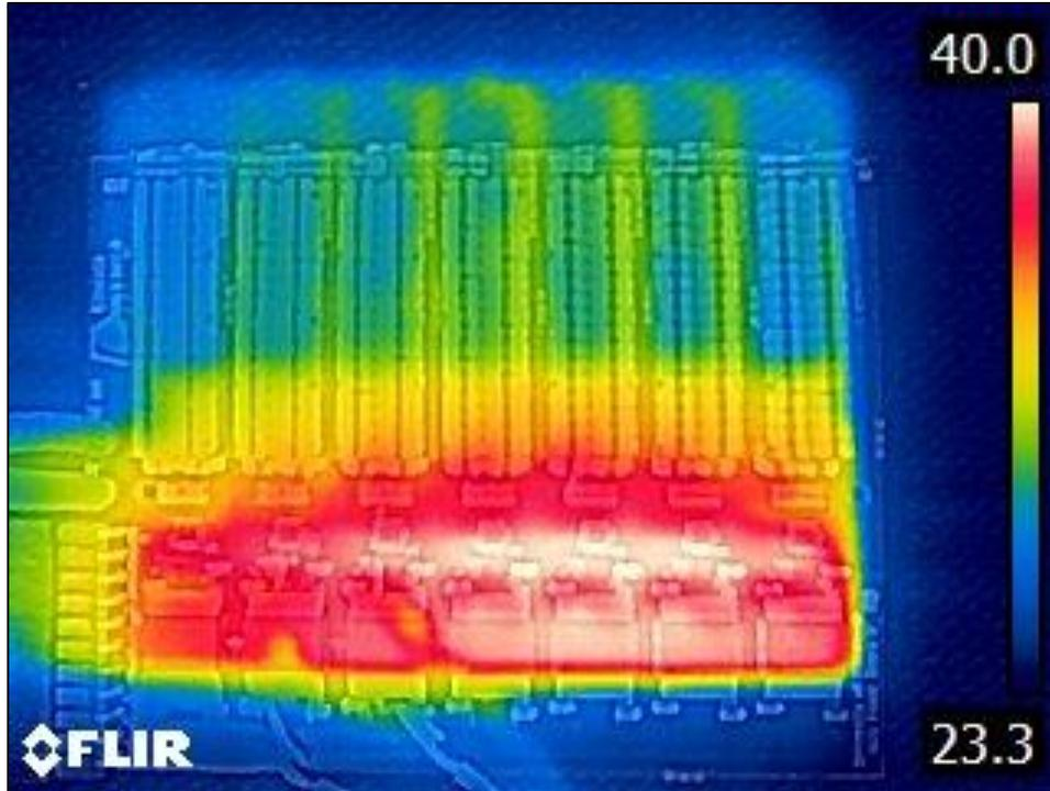
**Figure 62.** Thermal image of DC-AC MMC under loaded conditions
