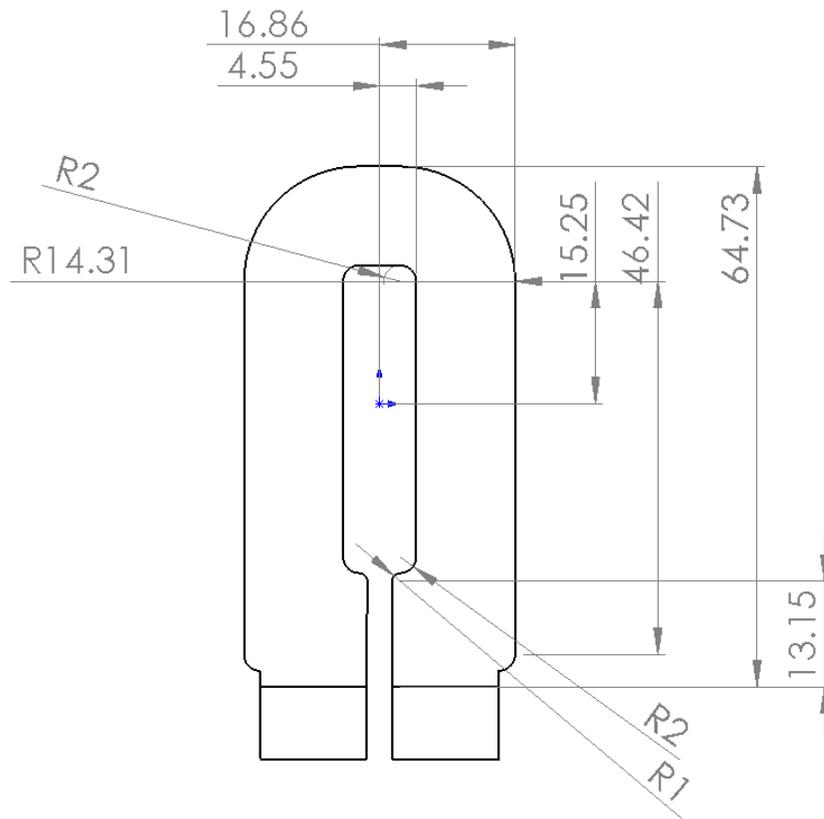
**Figure 24.** Solidworks drawing of transformer primary winding
