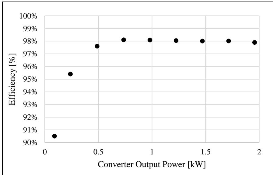
**Figure 44.** Simulated efficiency of DC-AC MMC
