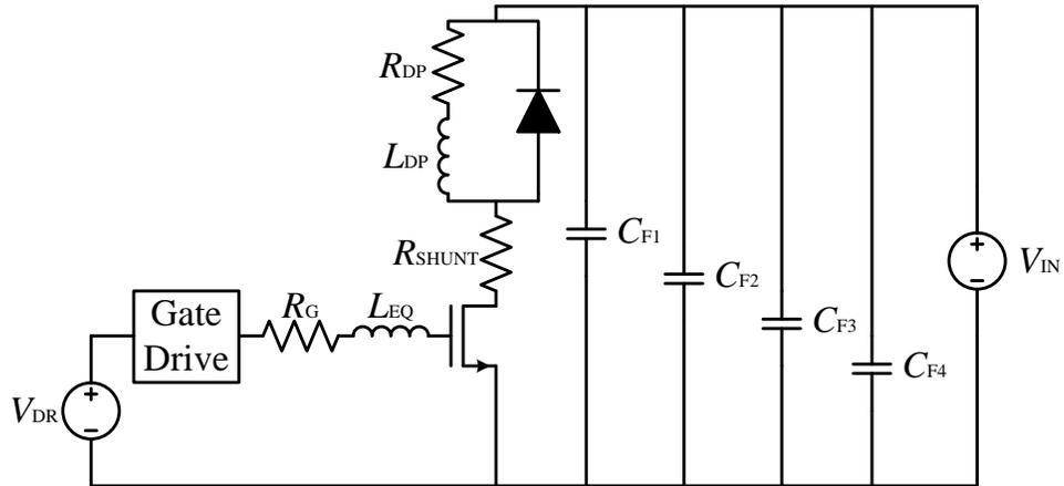
**Figure 14.** Double pulse test circuit for turn on measurements
