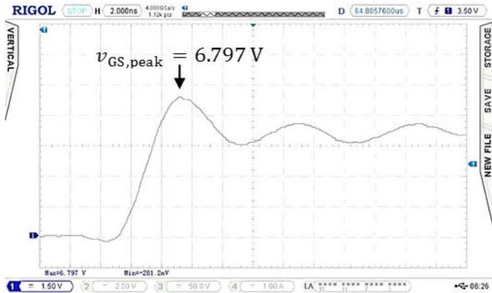
Figure 18. Turn-on of EPC8010 with  $R_G = 5 \Omega$
