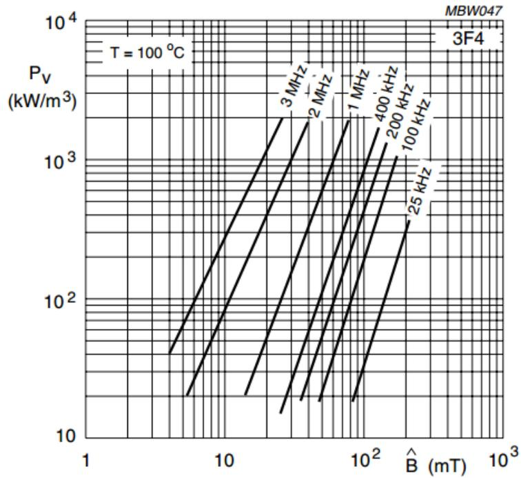
**Figure 7.** Specific power loss of Ferrocube 3F4 MnZn ferrite
