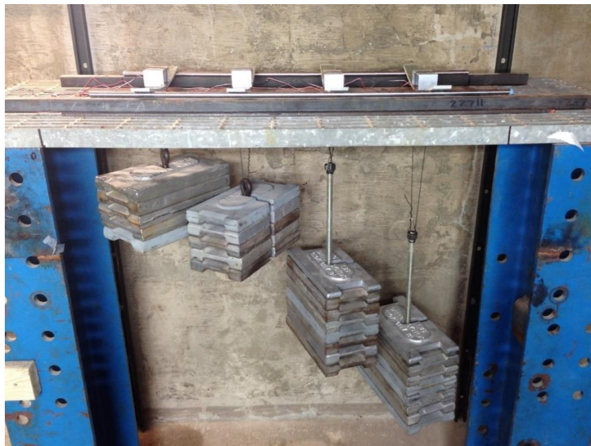
Figure 3.4 Creep test configuration showing four specimens under loads of 445 and 667 N
