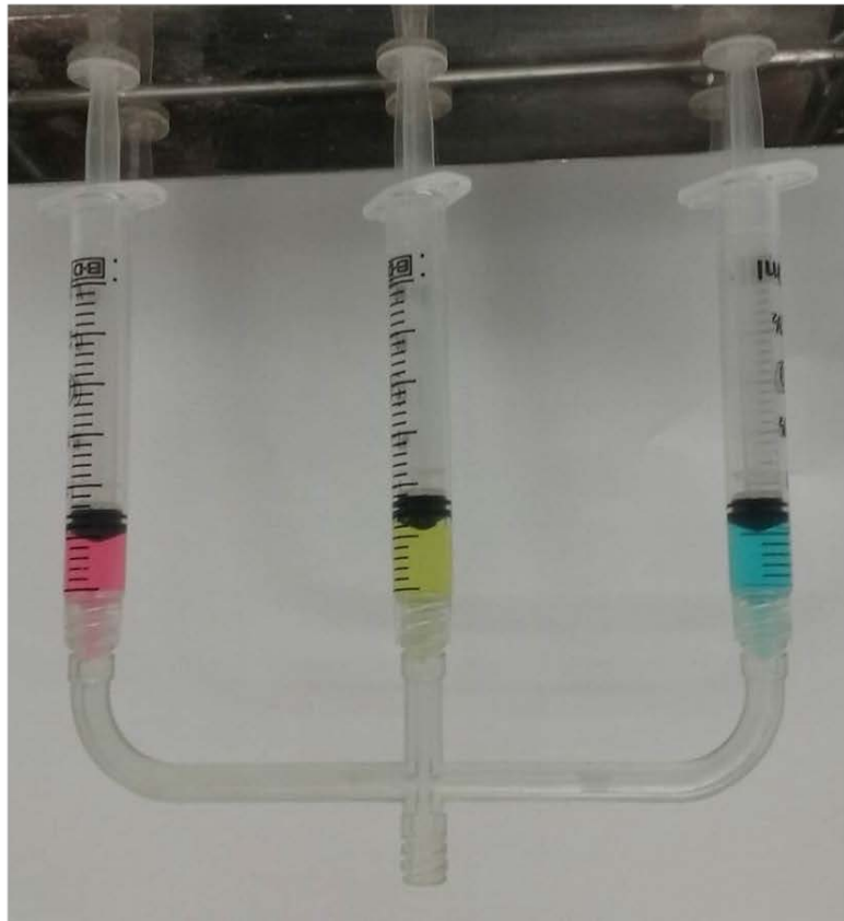
Figure 31. Cell delivery mixer designed to ensure gels are mixed only while injecting. A) The three inputs (top) were designed to accommodate a “Luer-Lok” syringe. Equal volumes of the fibrinogen, thrombin, and iron nanoparticle loaded ADMSCs will be loaded into three separate syringes and dispensed at the same time through the single output (bottom). B) Fibrin gel constituent components loaded into a syringe and locked in the fibrin gel mixer. From left to right, the constituents are fibrinogen solution (pink), cell suspension (yellow), and thrombin solution (blue).
