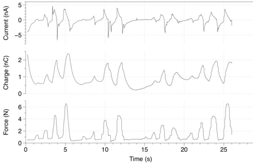
**Appendix Figure 10.** Measured current, charge (integrated current), and measured force over time during sample testing.
