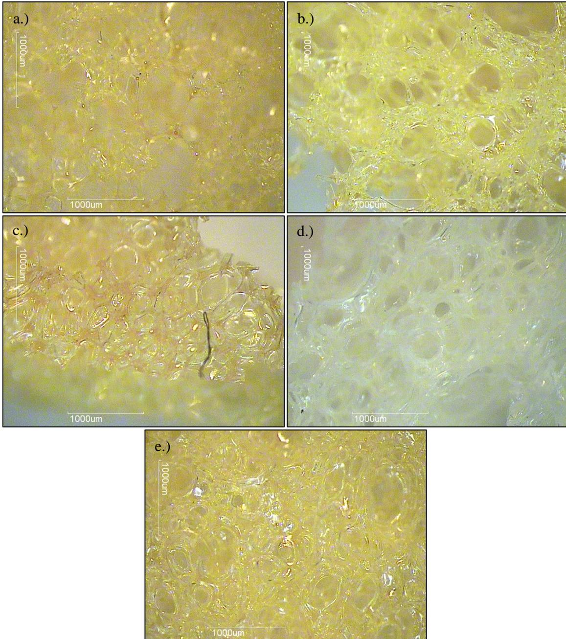
**Appendix Figure 14.** Micrographs of a.) non-poled sample, b.) 150 V, c.) 500 V, d.) 1051 V, and 2000 V poled samples.
