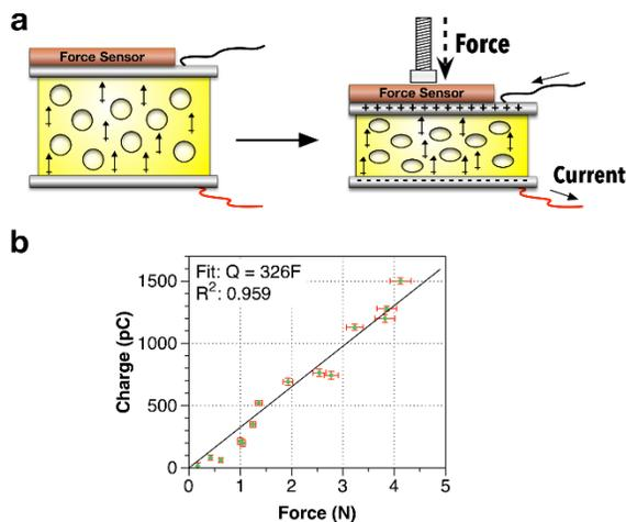
**Figure 6.1.** a) Schematic of foam material b) Net charge transferred as a function of applied force.
