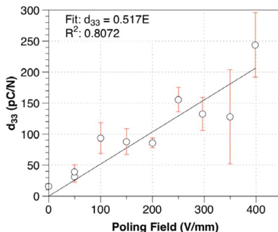
**Figure 6.3.** Piezoefficient as a function of poling field for samples doped with 0.2 M 2-chloro-4-nitroaniline.
