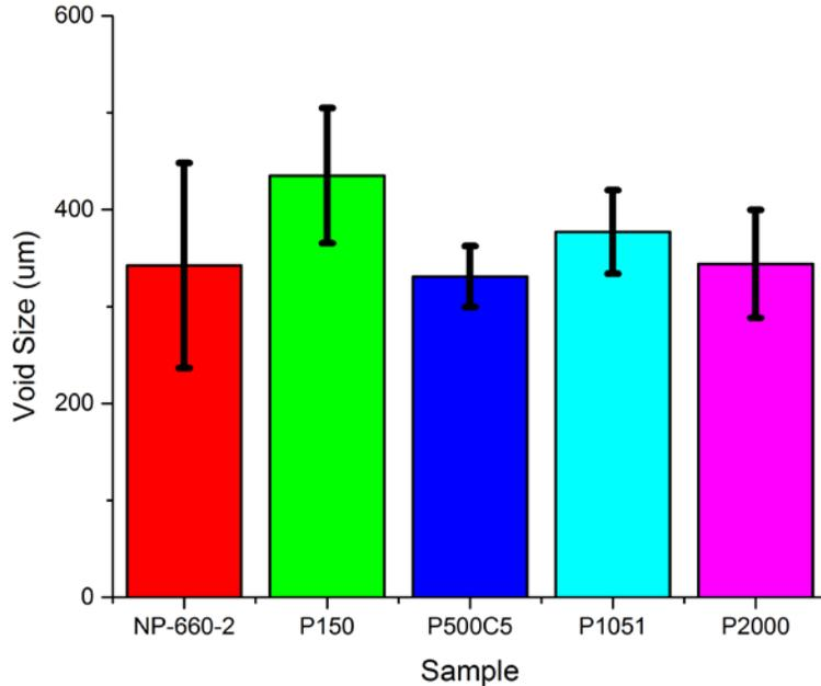
**Appendix Figure 15.** Average void size with error of samples above. NP – non-poled and P is poled.
