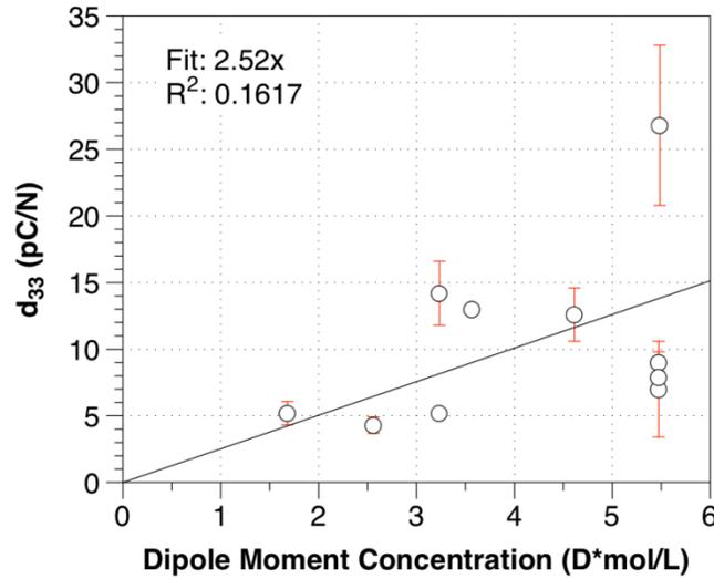
**Appendix Figure 11.** Piezoelectric coefficient as a function of dipole moment concentration for samples prepared with added acetone.
