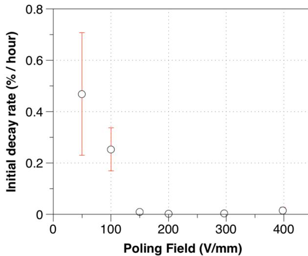
**Appendix Figure 12.** Initial decay rate of piezoresponse as a function of poling field.
