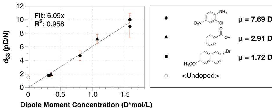
**Figure 6.2.** Piezocoefficient as a function of the product of dopant dipole and concentration when poled at  $40 \text{ V mm}^{-1}$ .
