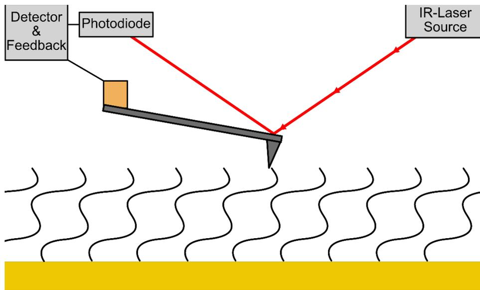
**Figure 1.3.** Working principle of an atomic force microscope. An IR-laser is placed on a cantilever probe which interacts with the surface of a sample and the IR reflection is measured by a photodiode. Any deformation of this signal is indicative of a change in topography of the surface of the sample.
