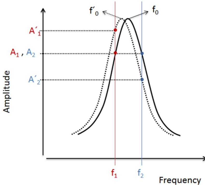
**Figure 1.4.** Adapted from ref.<sup>35</sup>, the working principle of DART-PFM allowing for the frequency tracking technique to be applied.
