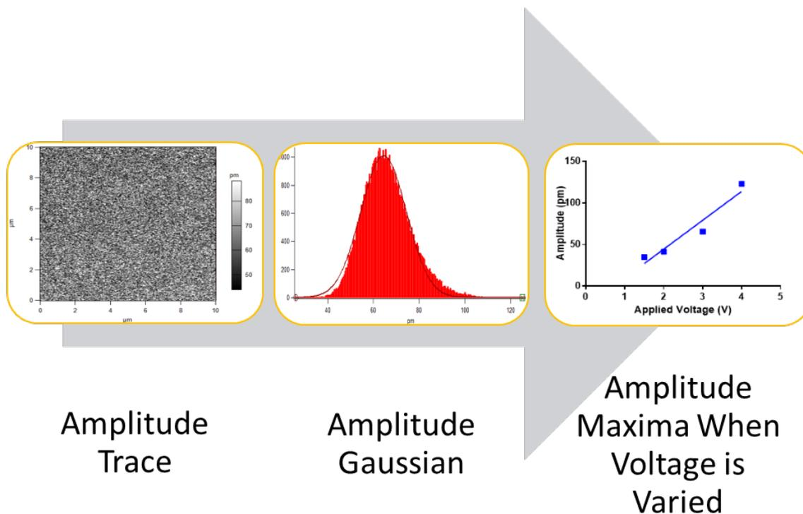
**Figure 5.7.** Process for acquiring semi-quantitative piezoresponse response of the peptides.
