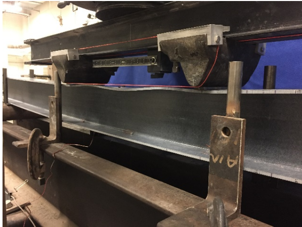
a) Buckling in constant moment region showing 3 half sine buckles over the 800 mm constant moment region
