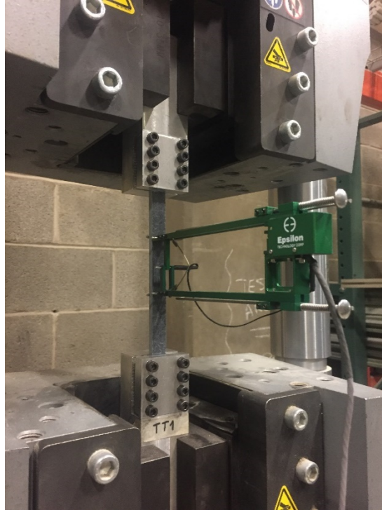
Figure 3.2 Tensile test set-up
