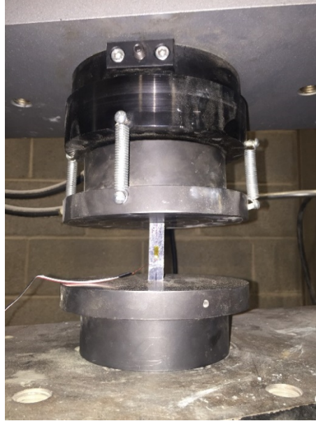
Figure 3.8 Compressive test set-up
