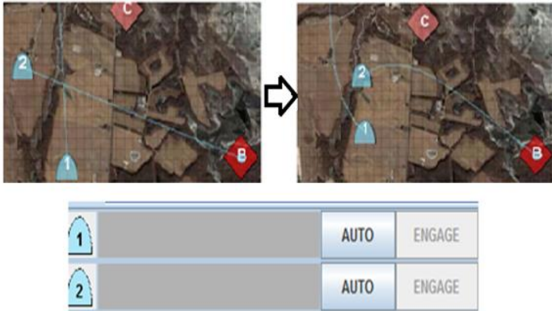
Figure 9. By clicking the auto button, new paths are applied to divert UAVs from a collision course
