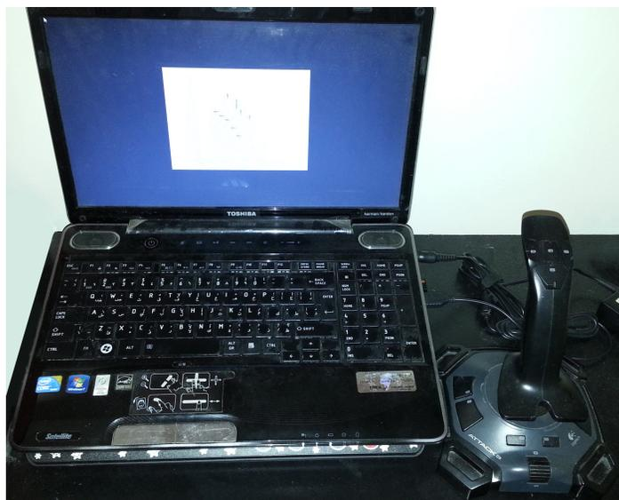
Figure 33: Computer simulation framework for aircraft conflict resolution HRC system. Human can cooperate with the computer controller by using joystick to control the acceleration of the lateral maneuver.
