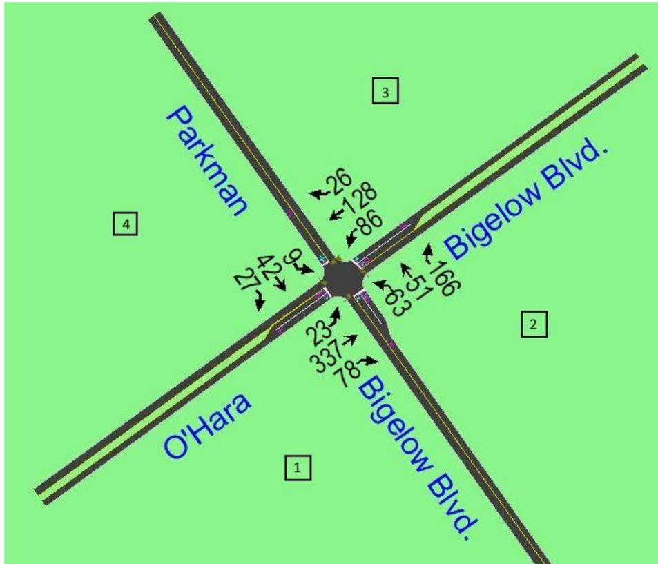
**Figure 4-20.** Bigelow Blvd.-Parkman Ave.-O'Hara St. intersection diagram
