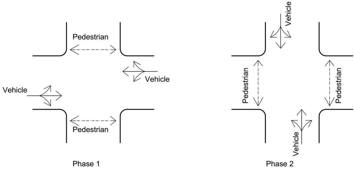
**Figure 2-1** Simple two-phase intersection with Concurrent Pedestrian Phasing
