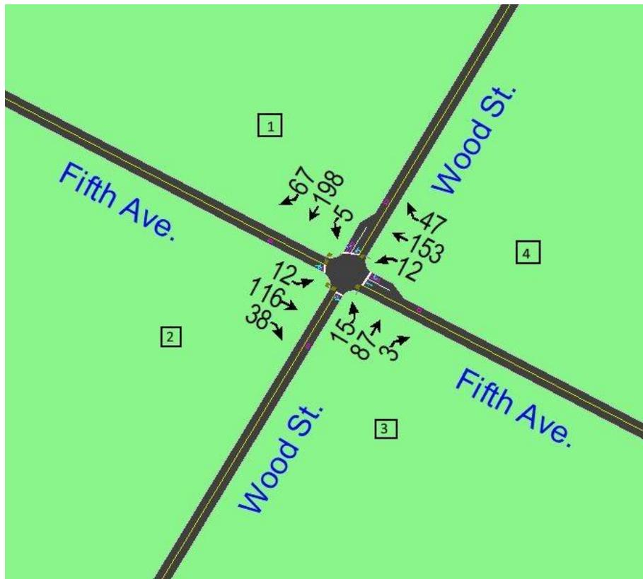
**Figure 4-19.** Fifth Ave. and Wood St. intersection diagram
