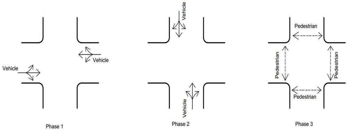
**Figure 2-2** Simple three-phase intersection with Exclusive Pedestrian Phasing
