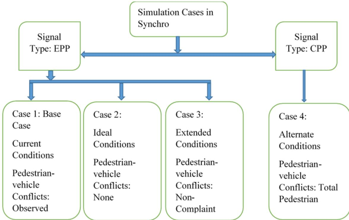
**Figure 3-2.** Different cases to analyze in traffic simulation tool Synchro
