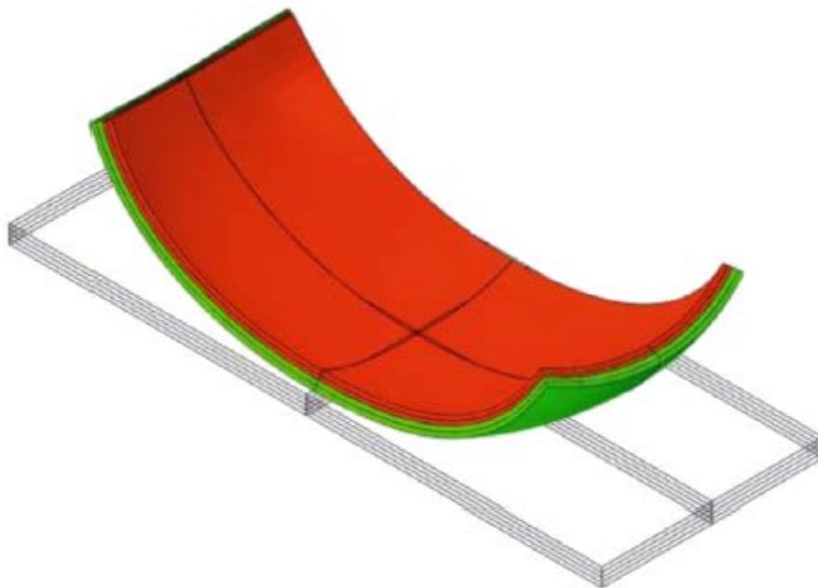
Figure 20. Simulated free sintering response of a bi-layer laminate presented by Van et al [6].
