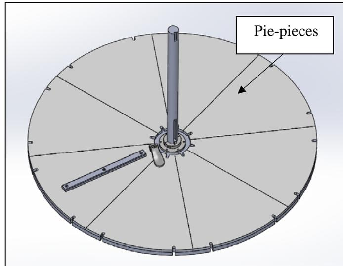
**Figure B 5.** Turntable Assembly with pie-pieces (only one slat mounted to pie-piece)
