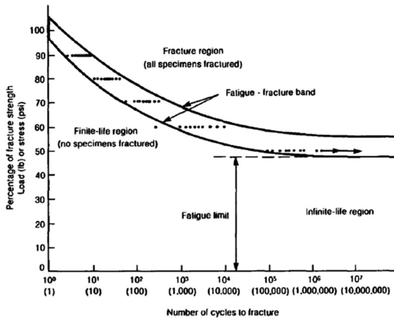
Figure E 3. Fatigue curve for typical medium strength steels[142]
