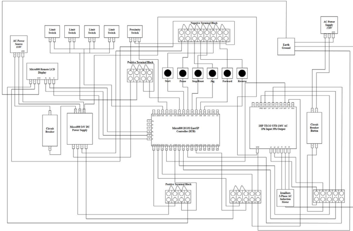
**Figure 7.** Electrical wiring for the caster test
