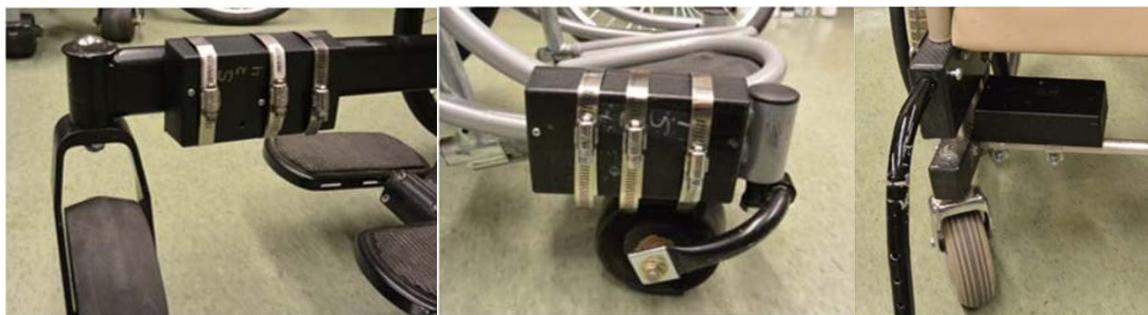
**Figure 18.** Accelerometers on MRT (left), WRR (center) and HKC (right) wheelchairs
