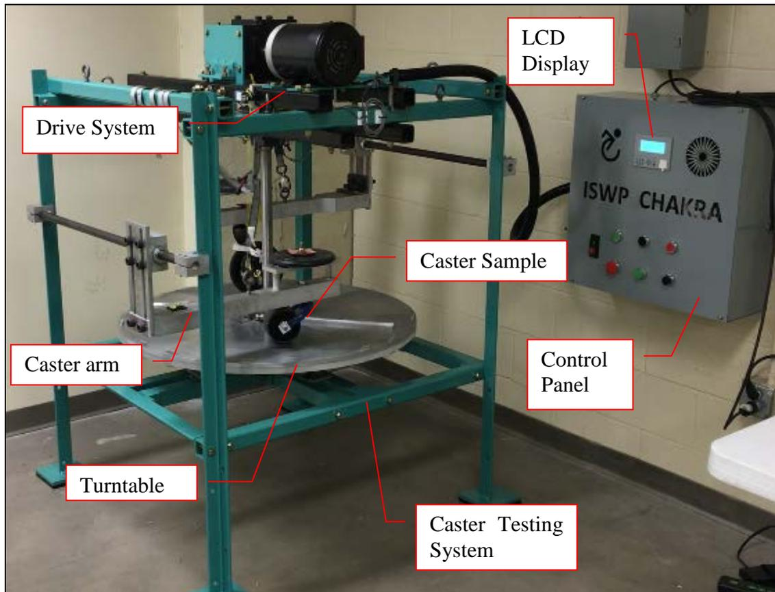
**Figure 9.** ISWP Caster Assembly Test
