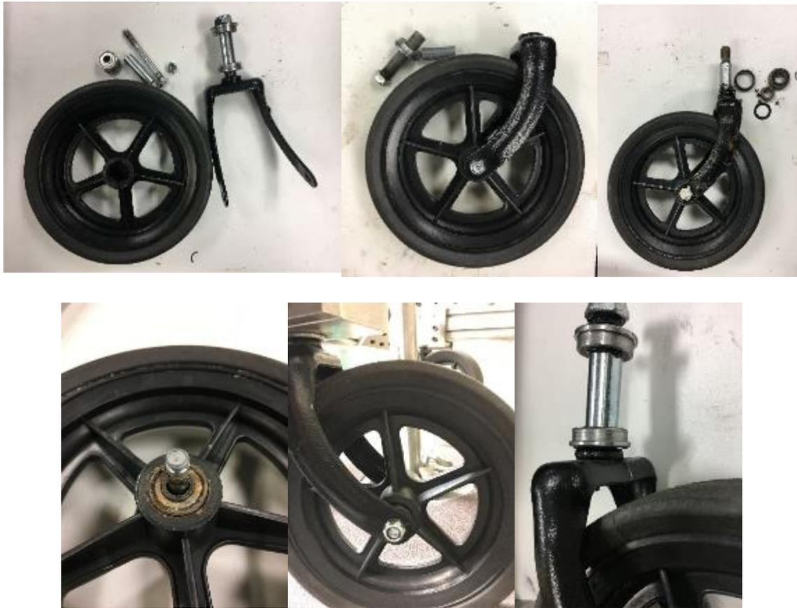
**Figure 35.** Failures with model C
