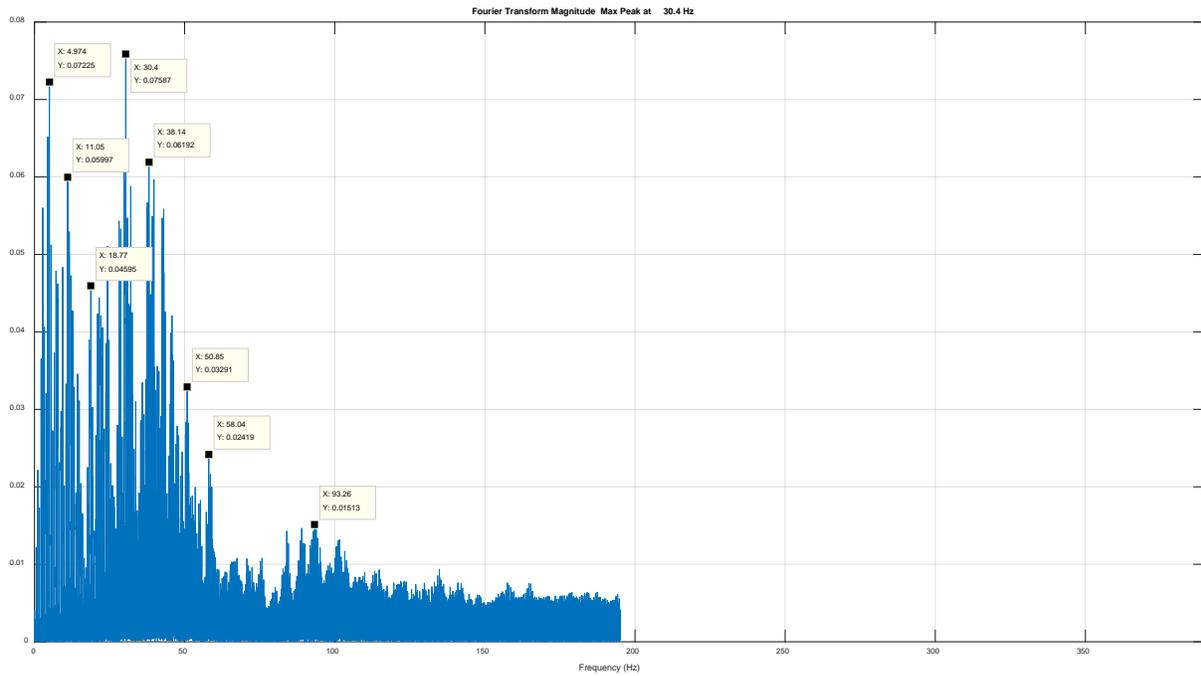
**Figure D 7.** FFT for vibrations seen on Whirlwind Roughrider caster fork in forward direction
