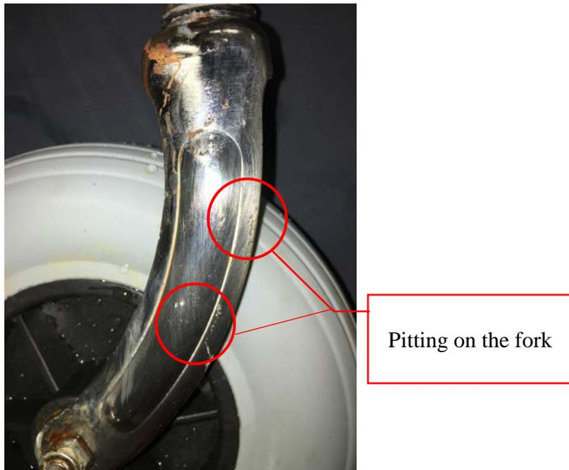
**Figure 38.** Corrosion effects on a chrome plated castor fork
