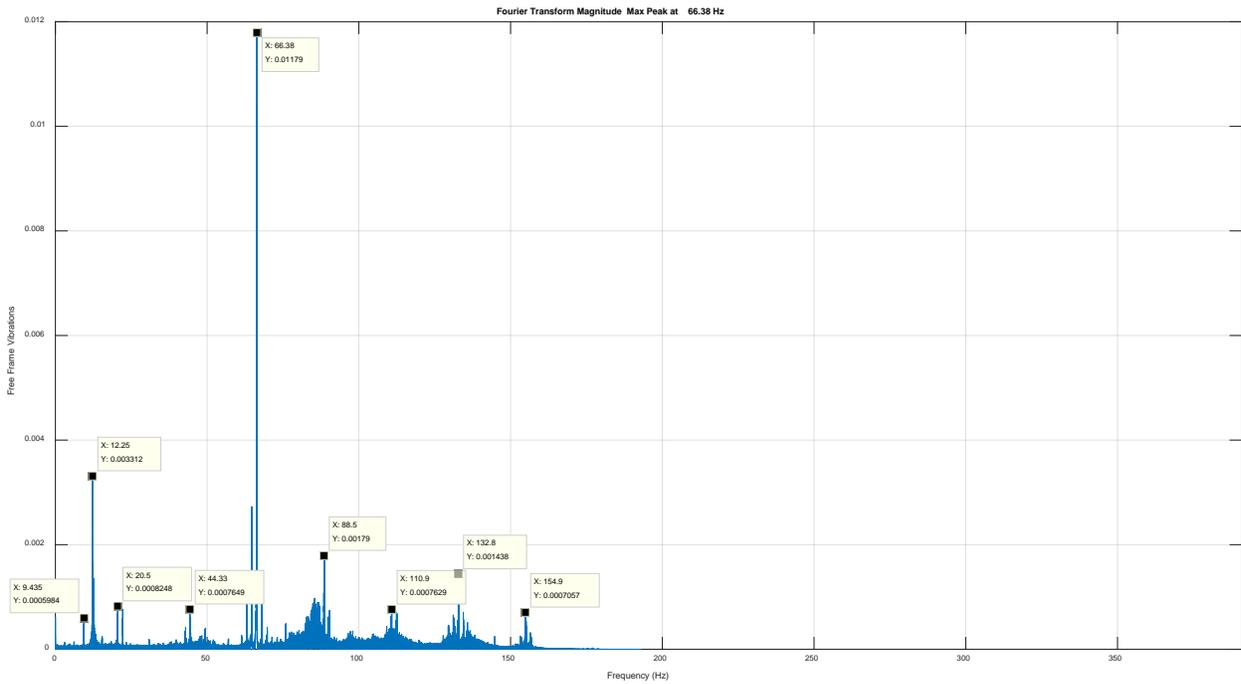
**Figure D 5.** FFT for vibrations seen on caster test frame in lateral direction
