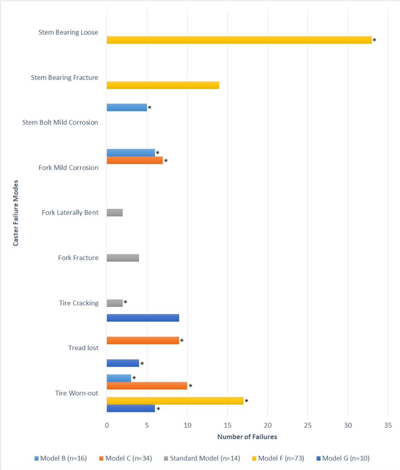
**Figure 31.** The three most common field failure modes for five caster models, \* indicates that the same mode was found during in-lab testing
