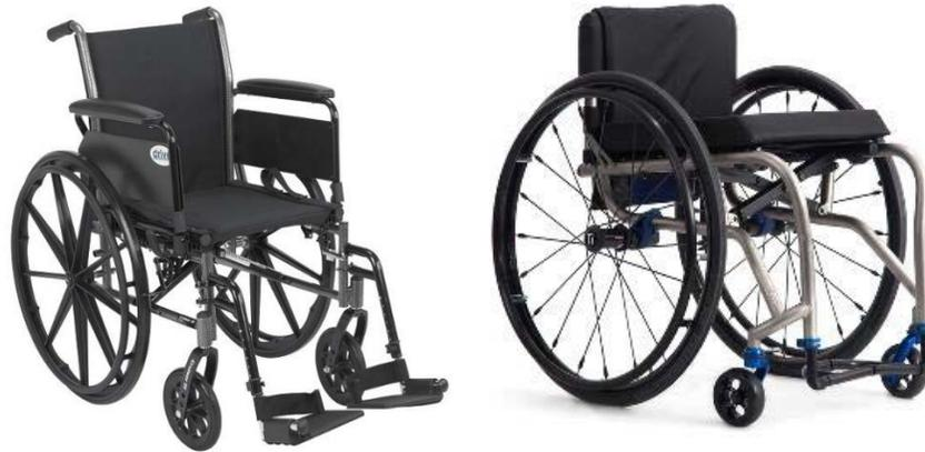
**Figure 3.** Lightweight wheelchair (left) and Ultra-lightweight wheelchair (right)[81]
