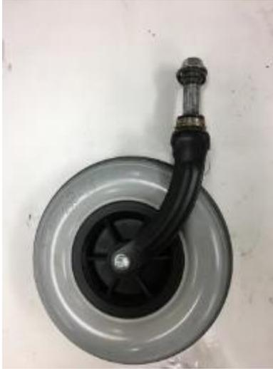
5.1a Review failure item - stem bearings corrosion
