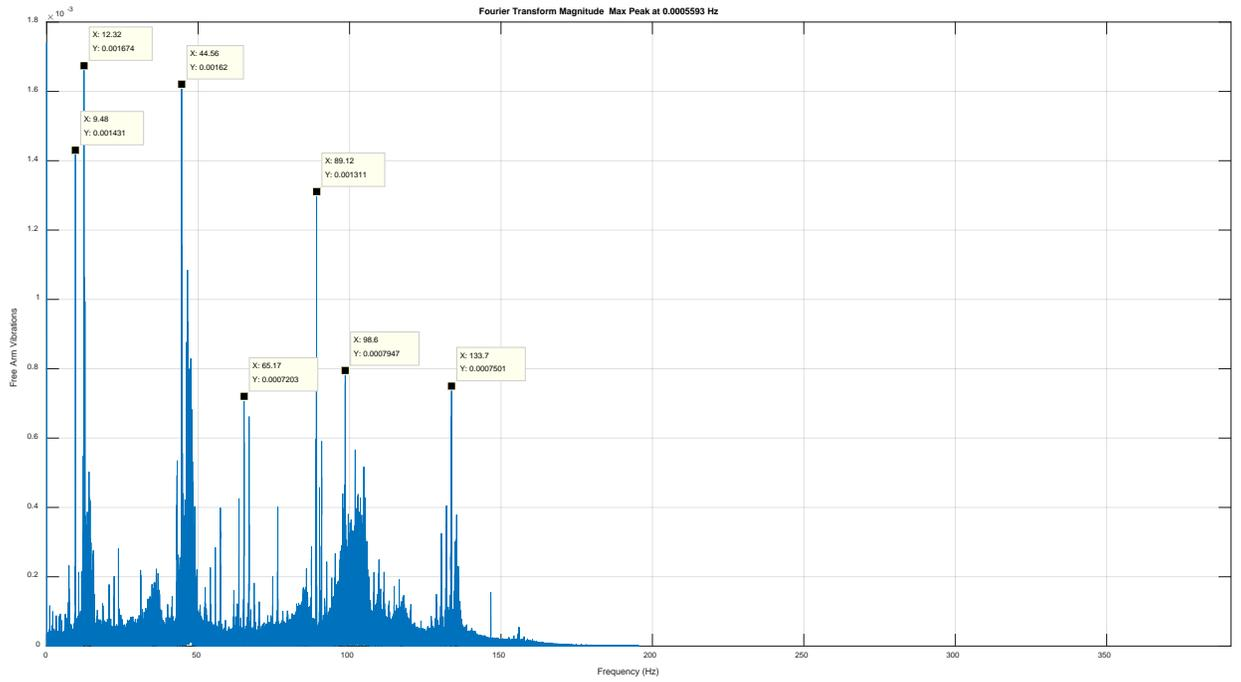
**Figure D 3.** FFT for vibrations seen on caster arm in vertical direction
