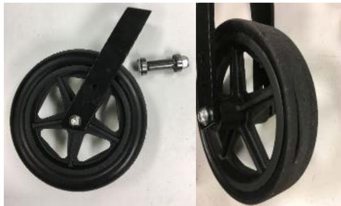
**Figure 37.** Model E failures. Shock tested sample (left) and abrasion + shock tested sample (right)
