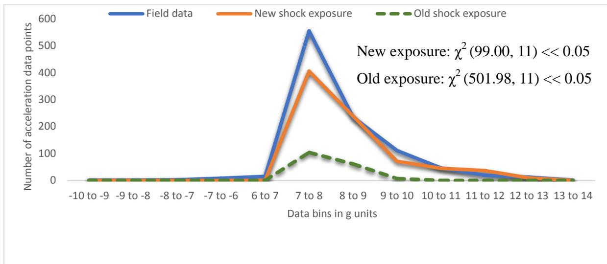
**Figure 25.** Field and caster test shock exposure histograms for HKC caster
