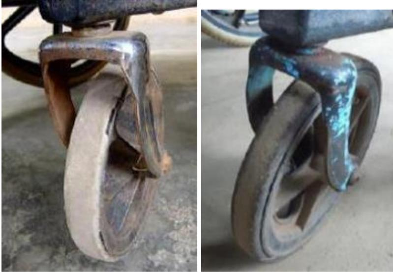
7.3a Review failure item - fork corrosion
