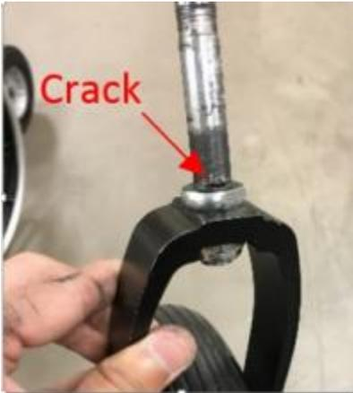
6.1a Review failure item - stem bolt fracture
