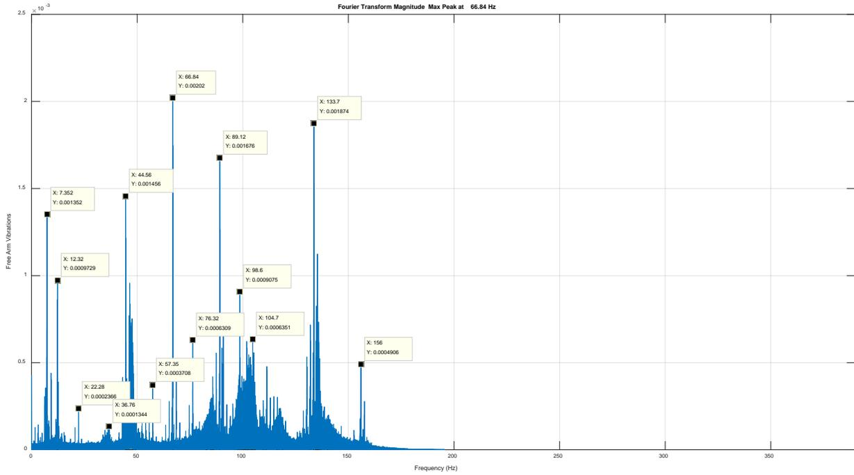
**Figure D 2.** FFT for vibrations seen on caster arm in lateral direction
