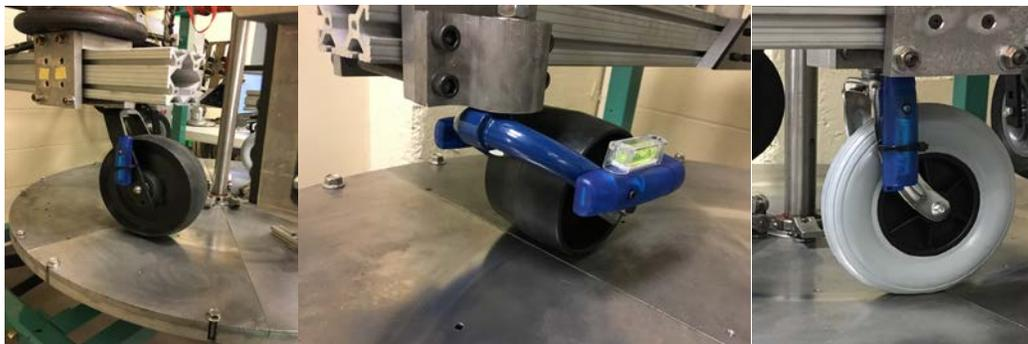
**Figure 19.** Accelerometers installed on MRT (left), WRR (center) and HKC (right) casters
