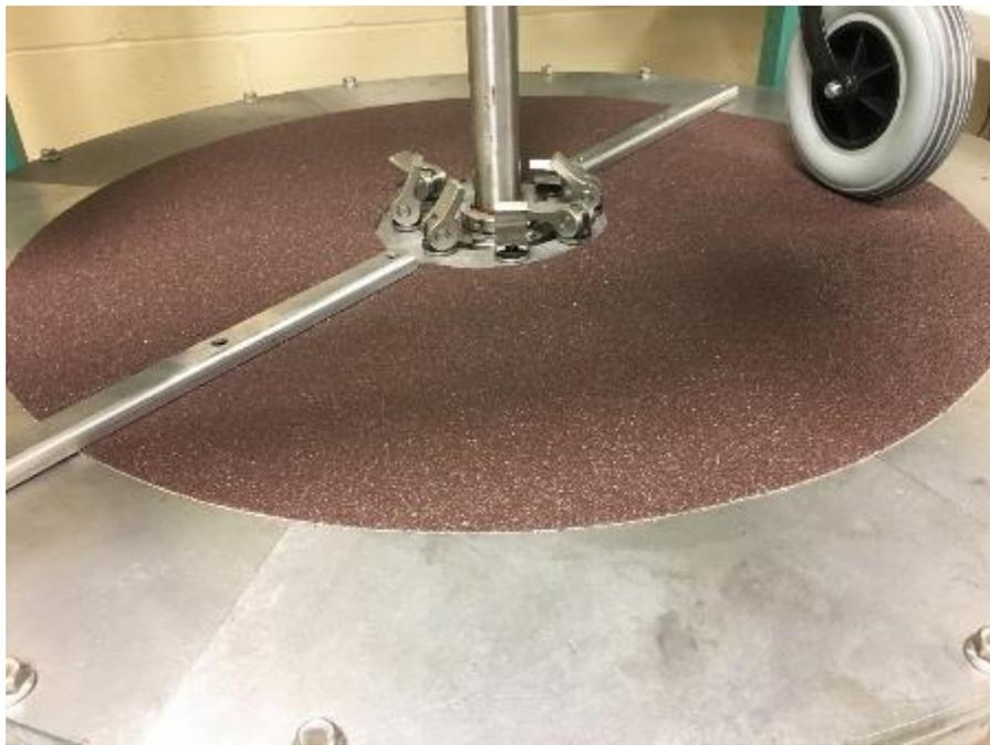
**Figure 27.** Sanding disc attached to the turntable to simulate abrasion
