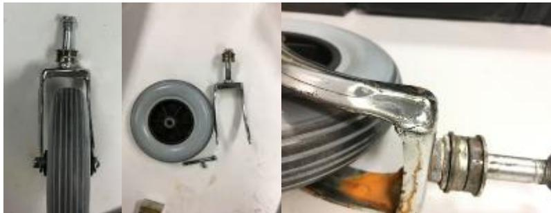
**Figure 39.** Model F failures. Shock tested sample (left and center) and corrosion + shock tested sample (right)
