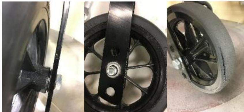
**Figure 36.** Model D failures. Shock tested samples (left and center) and abrasion + shock tested sample (right)
