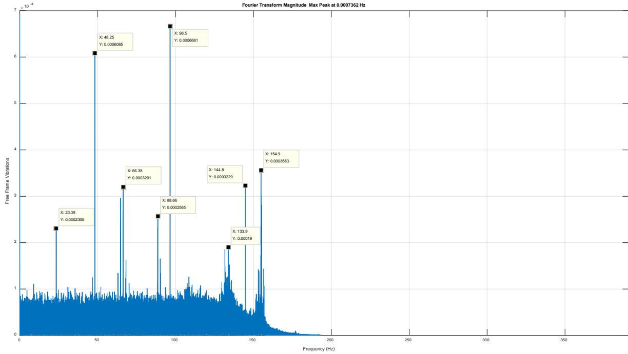
Figure D 6. FFT for vibrations seen on caster test frame in lateral direction
