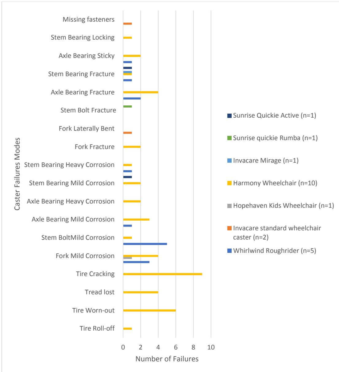
**Figure 14.** Field failures collected using caster failure checklist
