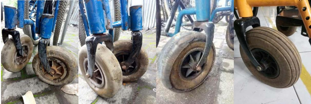
**Figure 15.** Caster failures with Harmony wheelchairs.
