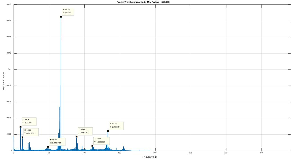
**Figure D 4.** FFT for vibrations seen on caster test frame in forward direction
