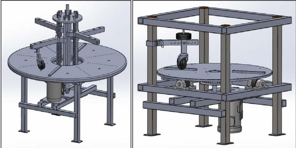
**Figure B 2.** Caster assembly test design concepts #4 (left) and #5 (right)
