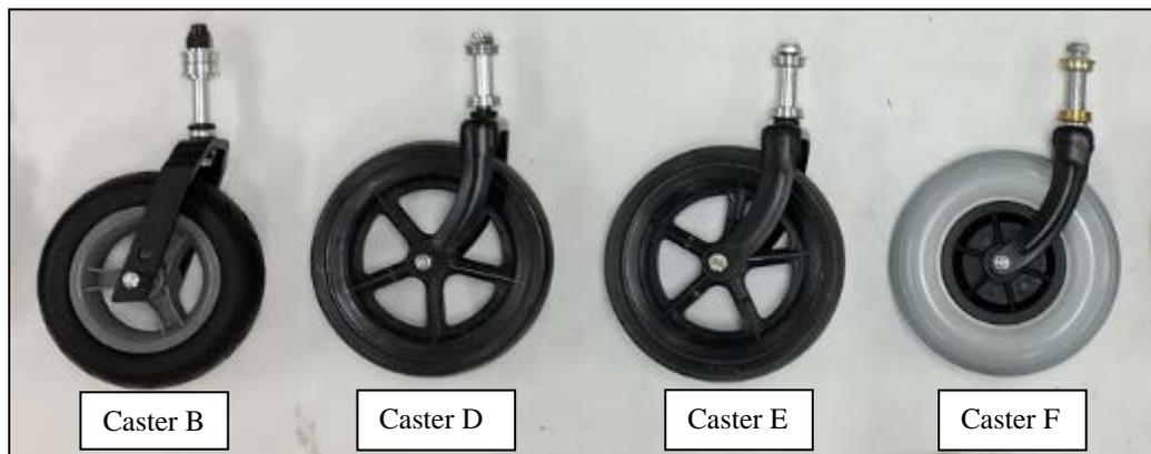
**Figure 11.** Caster assemblies tested in preliminary testing study (Model A and C are not shown)
