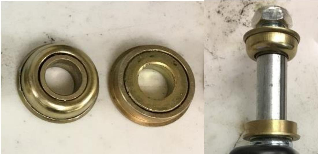
**Figure 43.** Stem bearings supplied with model G for testing
