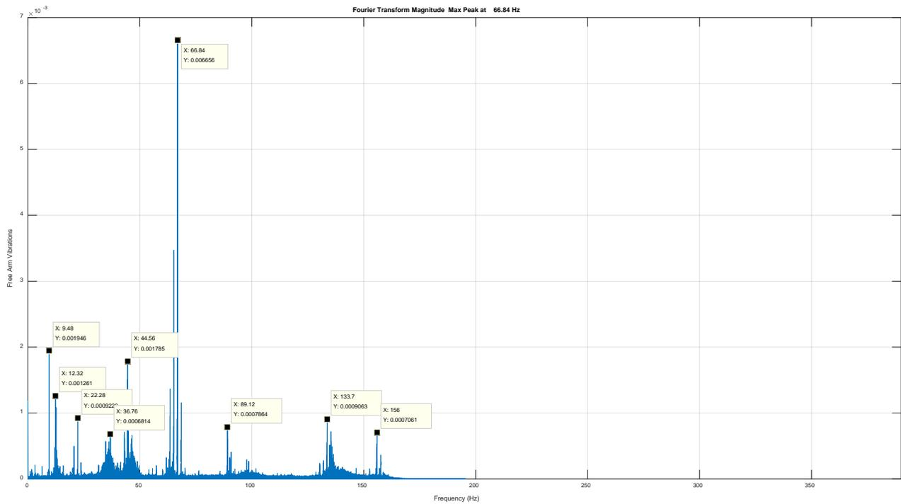
Figure D 1. FFT for vibrations seen on caster arm in forward direction
