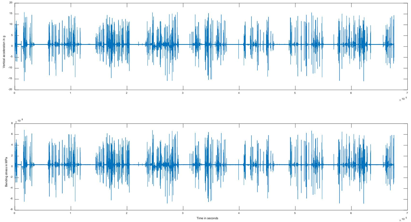
**Figure E 1.** Vertical accelerations and bending stresses seen by the WRR caster stem bolt.
