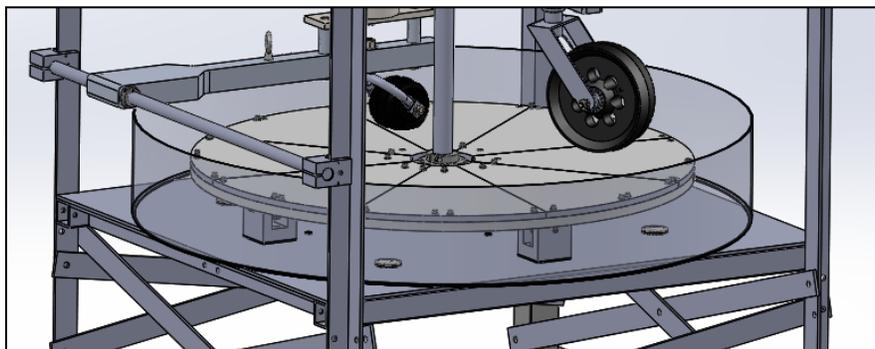
**Figure 12.** Incorporating water tank around the turntable
