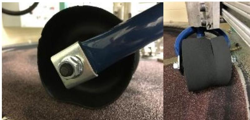
**Figure 33.** Worn out tires of abraded model B samples. Tire cracking failure (right).
