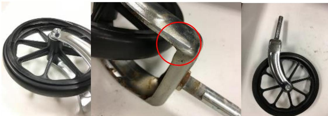
**Figure 45.** Model H testing failures. Wheel fracture (left), fork crack (center) and bent stem bolt (right)
