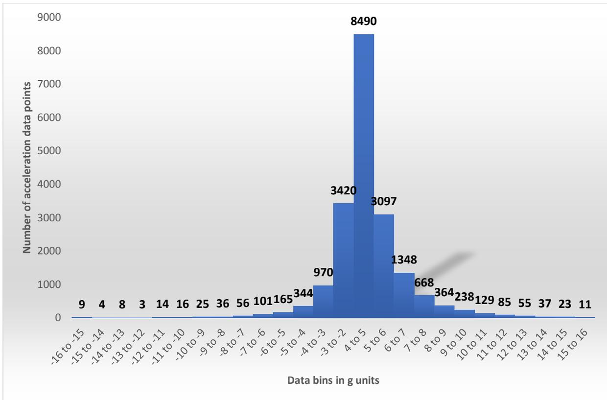
**Figure 21.** Accelerations seen by the WRR caster in the field (only one user)
