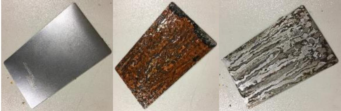
**Figure 26.** Mass loss test panel before corrosion (left), corroded panel after 100hrs of salt fog exposure (center) and cleaned panel before weighing (right)
