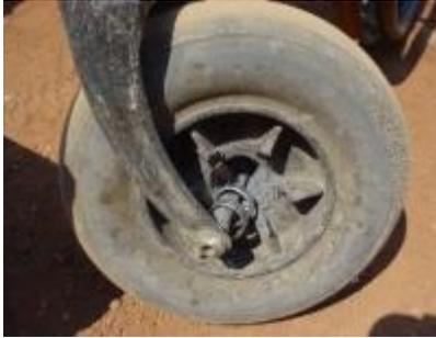
2.3a Review failure item - axle bearing fracture
