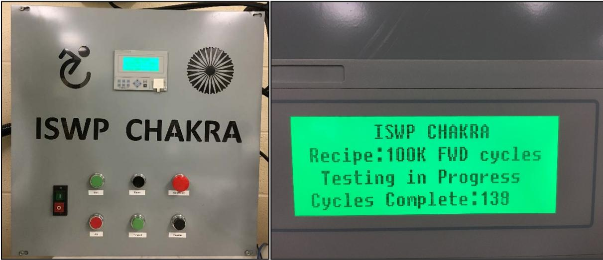
**Figure B 4.** Controller box of the caster test system (left) and LCD display (right)
