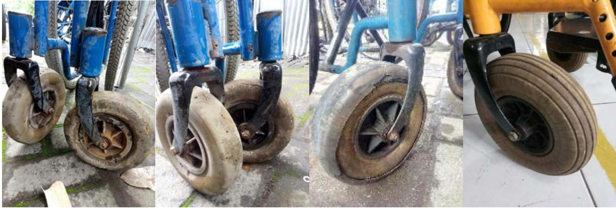
**Figure 15.** Caster failures with Harmony wheelchairs.
