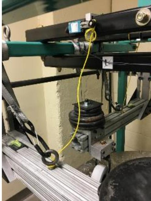
**Figure 8.** Limit switch for detecting caster arm fall.
