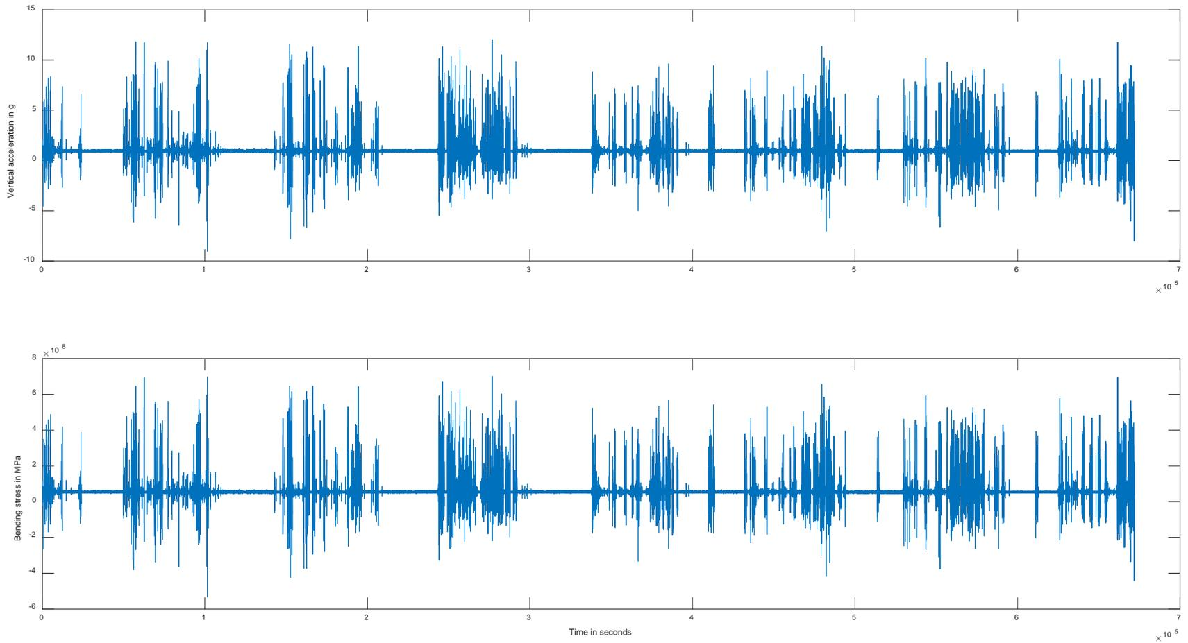
**Figure E 2.** Vertical accelerations and bending stresses seen by the HKC caster stem bolt.
