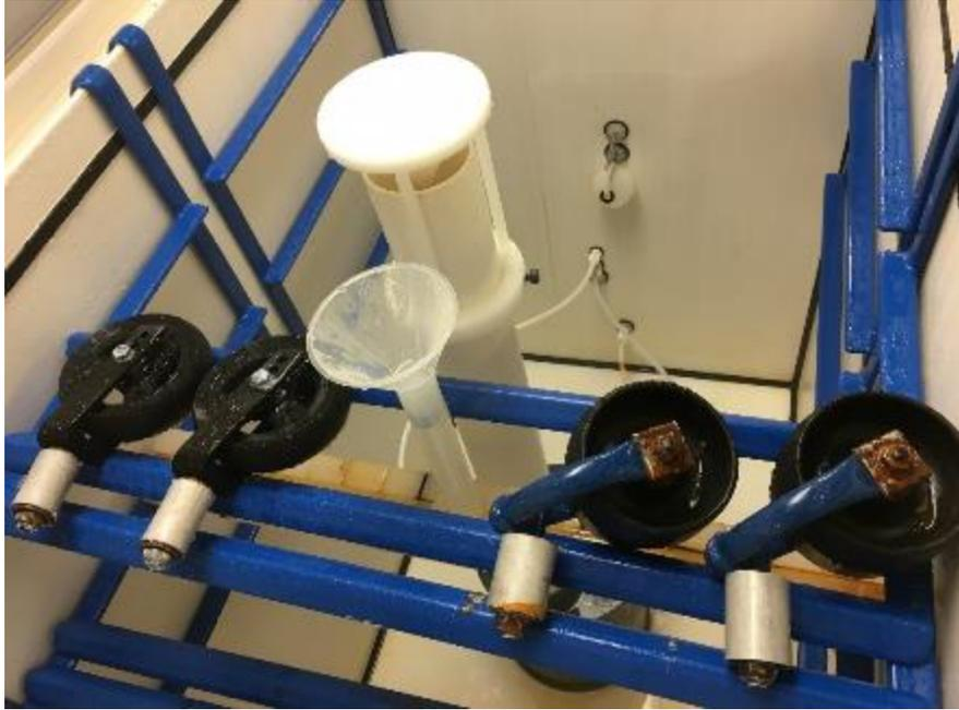
**Figure 29.** Casters exposed to corrosion in the salt fog chamber
