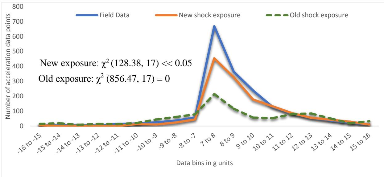
**Figure 24.** Field and caster test shock exposure histograms for WRR caster
