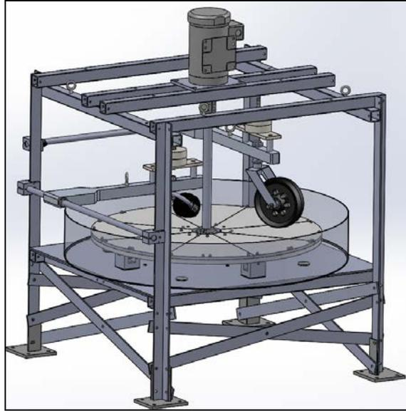
**Figure B 3.** Turntable design concept
