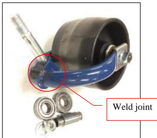
**Figure 13.** Fork weld joint on model C
