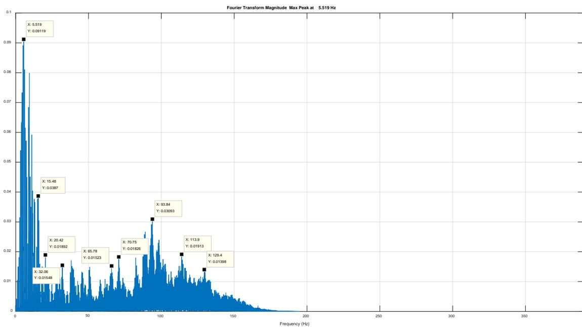
**Figure D 9.** FFT for vibrations seen on Whirlwind Roughrider caster fork in vertical direction
