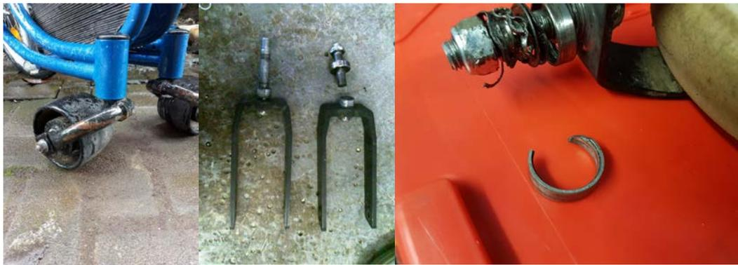
**Figure 16.** Caster failures with Whirlwind Roughrider (left), Sunrise Quickie Rumba (center) and Invacare Mirage (right)
