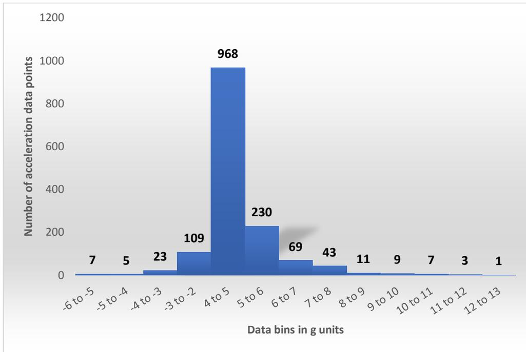
**Figure 23.** Accelerations seen by the HKC caster in the field (User 2)
