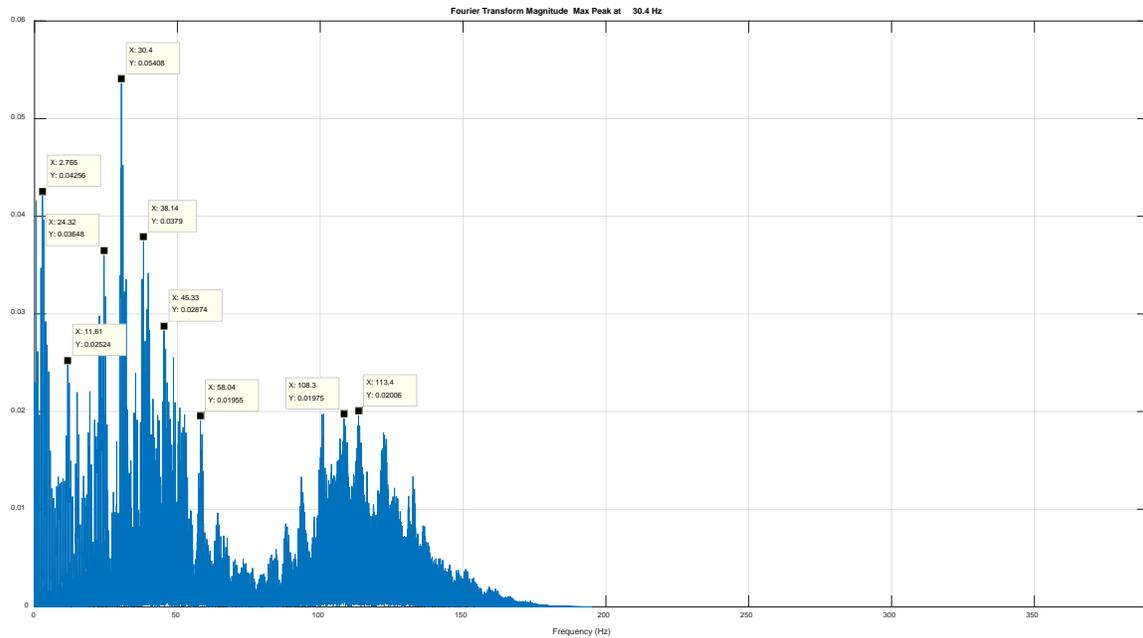
**Figure D 8.** FFT for vibrations seen on Whirlwind Roughrider caster fork in lateral direction
