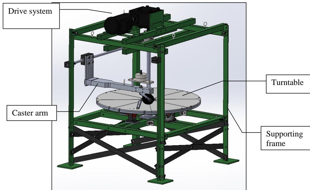
**Figure 6.** Final caster test equipment drawing for fabrication (includes only one caster support arm)
