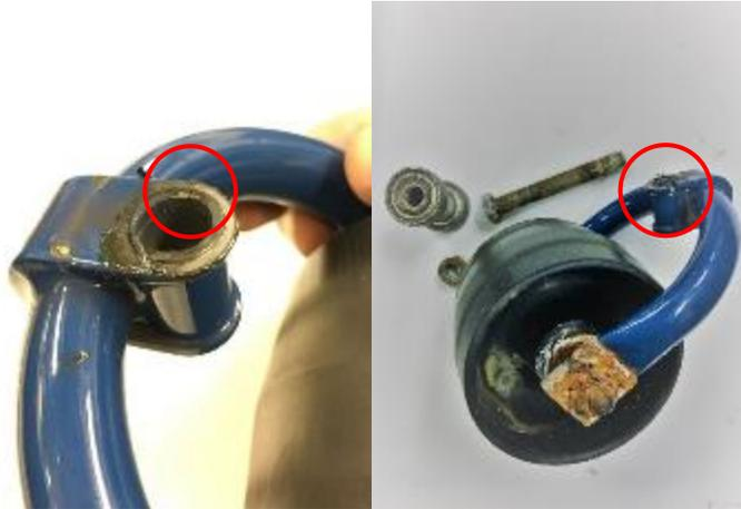
**Figure 34.** Fork cracks in model B samples.
