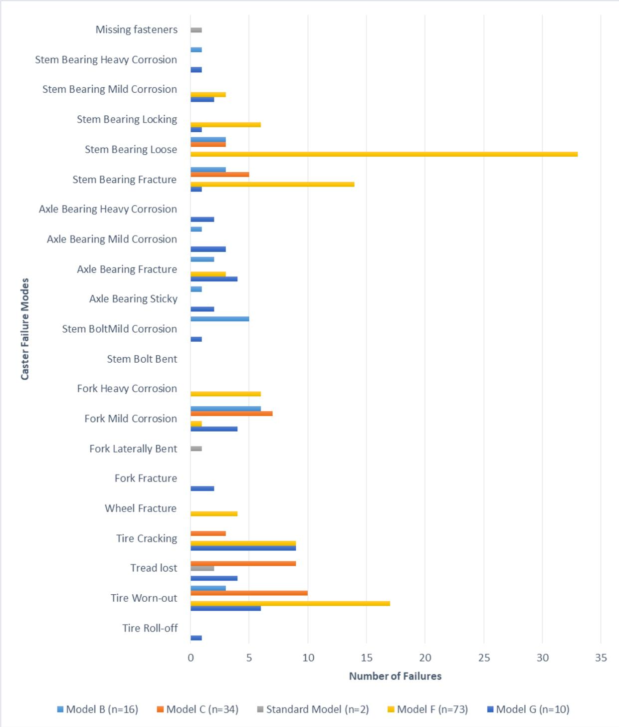
**Figure 30.** Field failures collected using the caster failure checklist and WCQ-C tool
