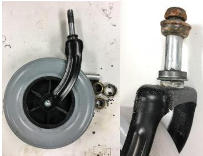
**Figure 44.** Failure mode seen with model G, bearing fractures (left) and fork crack (right)
