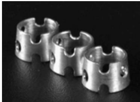
Figure 14: Mg ring implants manufactured with single crystal Mg
