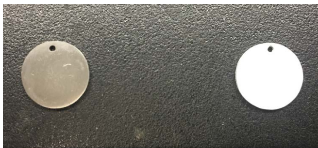
Figure 22: Photograph of Mg disk sample before and after MAO coating
