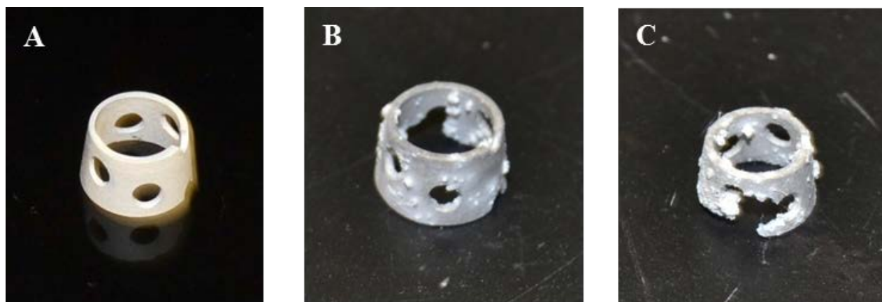
Figure 19: Photographs of the MAO coated Mg ring implants from the previous "healing study" before hydrogen evolution measurements (A) and after immersion in HBSS (B&C)
