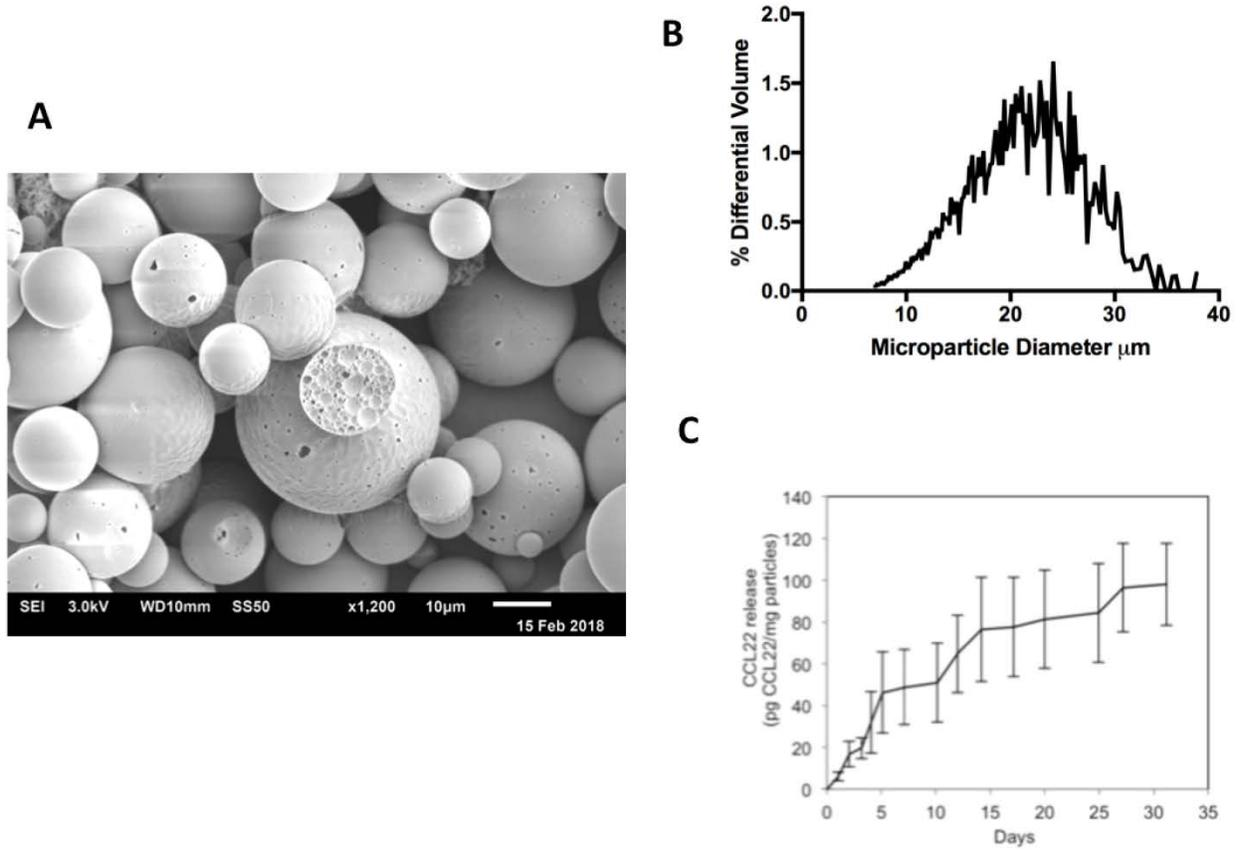
**Figure 10. The characterization of Recruitment-MP.** Recruitment-MP is spherical in shape and slightly porous (A) with an average particle diameter of 18.3µm (B). Release kinetics demonstrate that Recruitment-MP release CCL22 in a linear fashion for 30 days (C).
