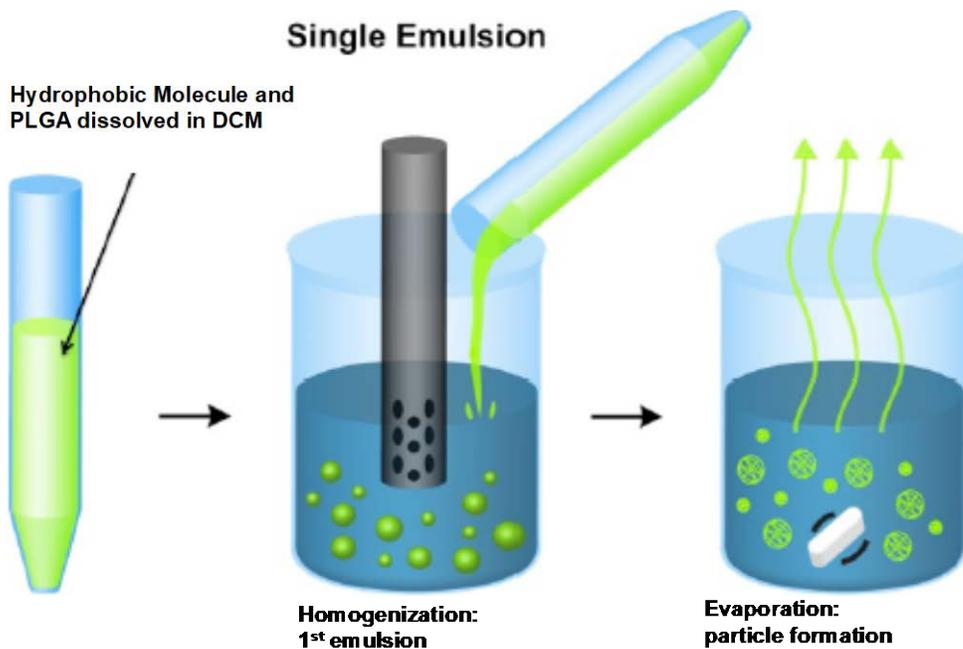
**Figure 17. Illustration of the water-in-oil single emulsion technique used to fabricate Rapamycin microparticles (Rapa-MP, a component of TRI-MP).**
