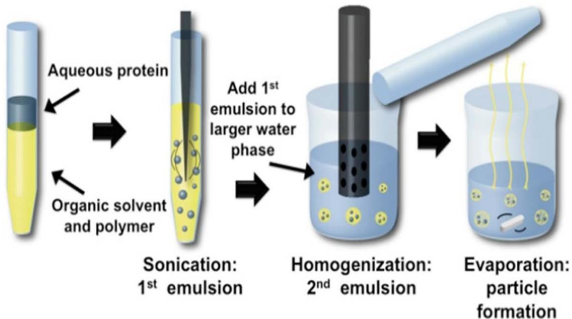
Figure 5. Recruitment-MP were fabricated using a water in oil in water (W/O/W) double emulsion technique.
