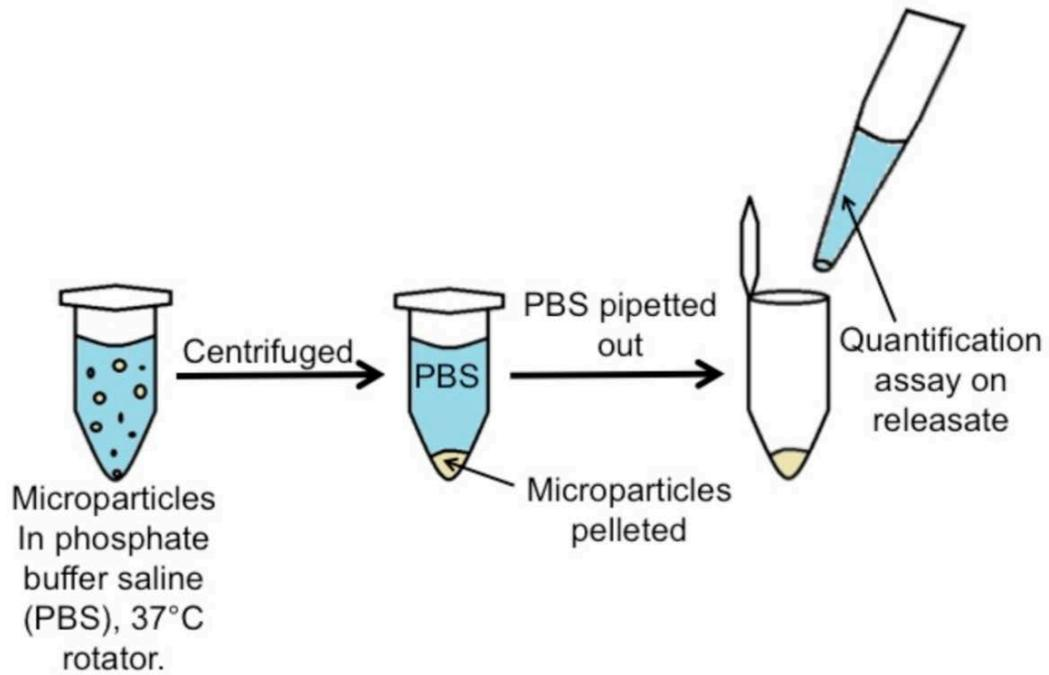
**Figure 6.** *In vitro* release of CCL22 from Recruitment-MP was measured for 40 days.
