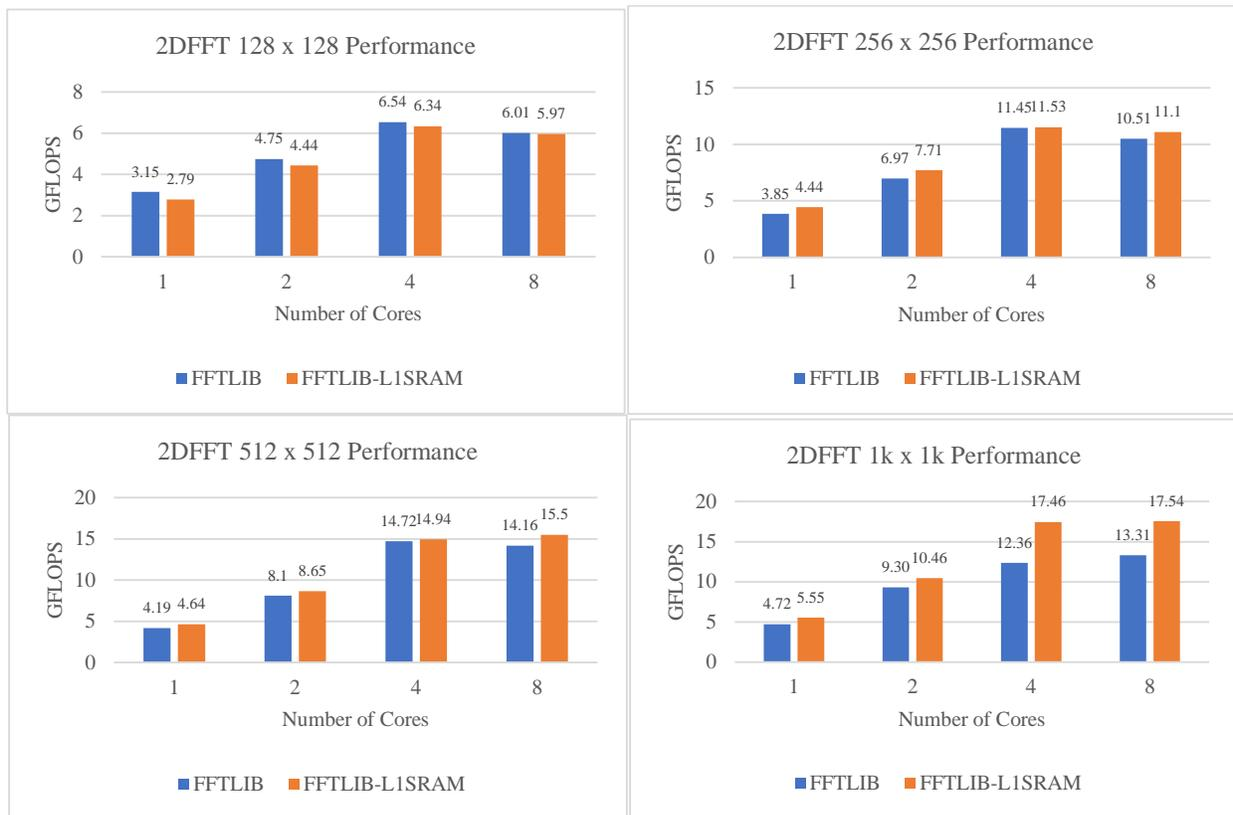
**Figure 12.** K2EVM-HK 2D-FFT performance with and without L1-SRAM in the DMA scheme
