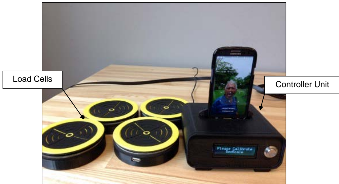
Figure 4: E-Scale system - four load cells and the bedside controller unit.
