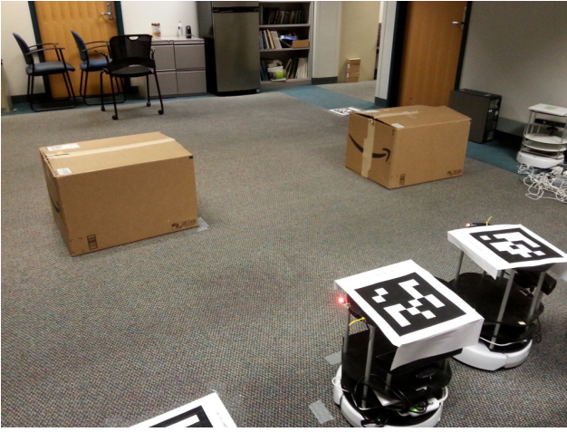
Figure 6. Actual environment used for trials with robots in their initial locations. The large boxes are obstacles.
