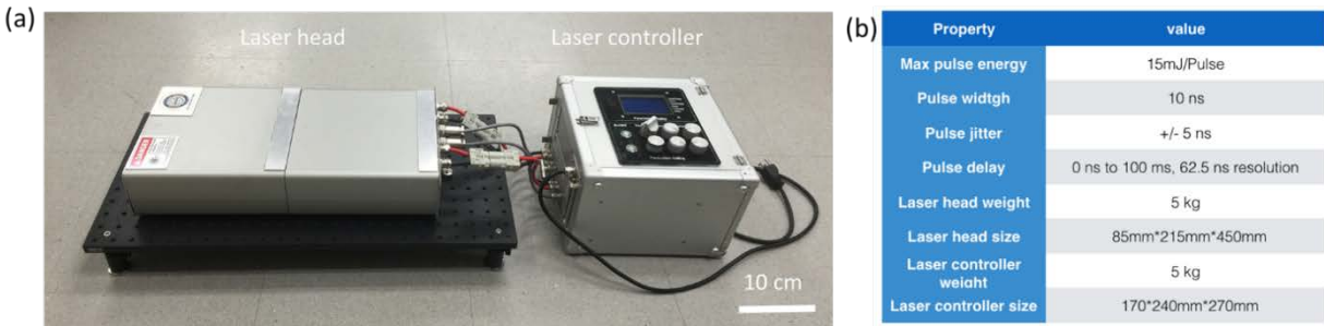
Figure 3.1 (a) Photo of the double-pulse laser system that consists of a laser head and a laser controller and (b) the laser system's key parameters.
