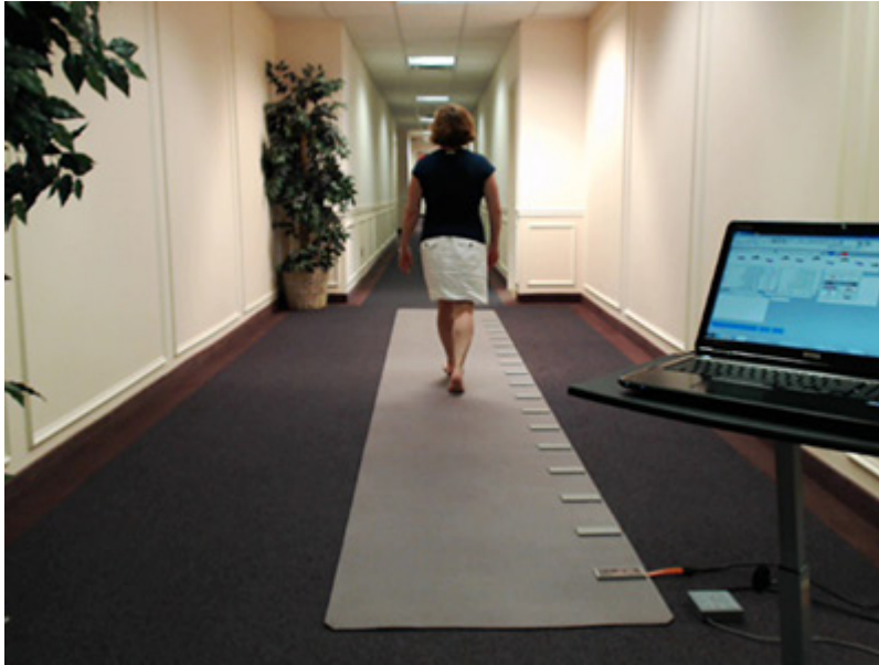
Figure 9 Participant walking on portable GAITRite® Walkway System
