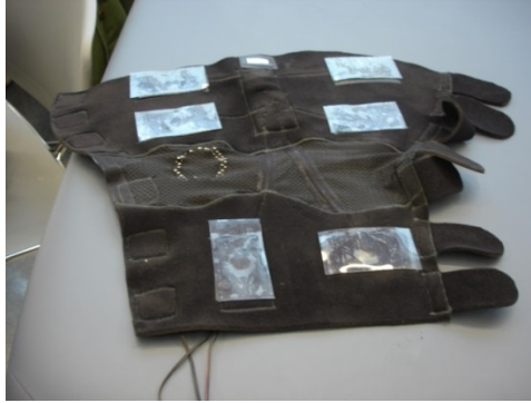
Figure 5 Final garment with electrodes in place, inside view
