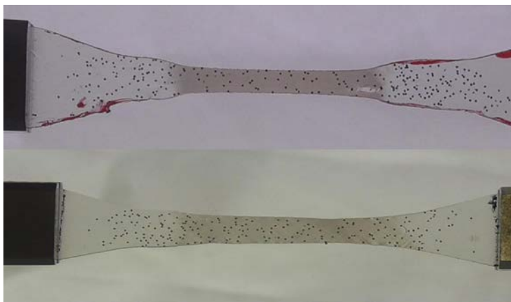
Figure 12 Snapshots at 900 mm/min showing differences in drawing. The rubber:plastic ratio of upper is roughly 1:1 and roughly 4:1 of the bottom one.
