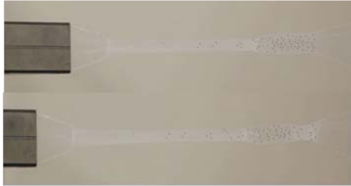
Figure 16 The images of multiple necking happened.
