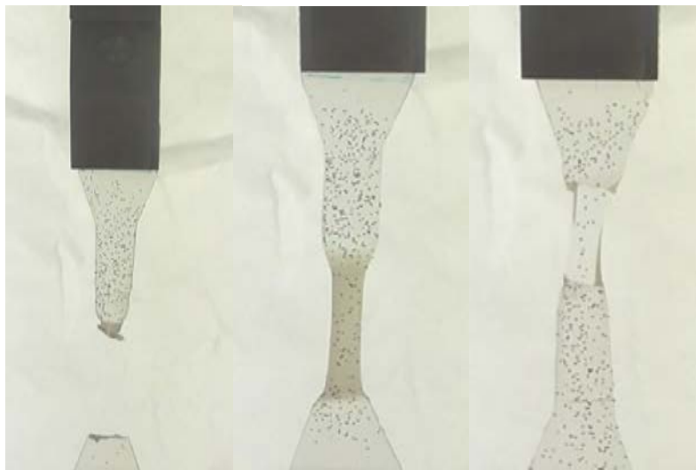
Figure 3 (a) Cracked HDPE-Rubber composites (b) Drawing HDPE-Rubber composites (c)Delaminated HDPE-Rubber composites
