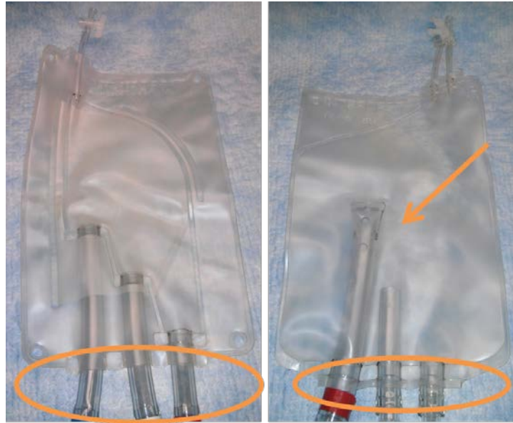
Figure 10. Commercially available, pediatric ( left ) and adult ( right ) soft-shell reservoirs used in previous benchtop blood biocompatibility experiments highlighting the deficient extraneous and fenestrated ports.
