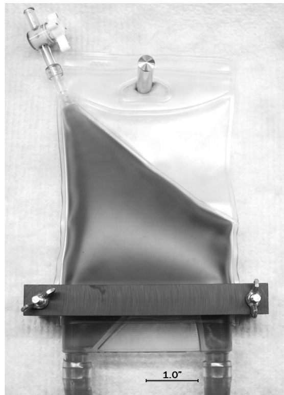
Figure 13. The vertically hung, ½”-port blood reservoir assembly after clamping, filling and de-airing.
