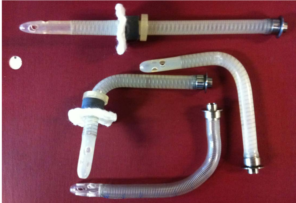
Figure 21. Representative inflow cannula used for PF1-PF3 in vivo implants with custom sewing rings and pump connectors.
