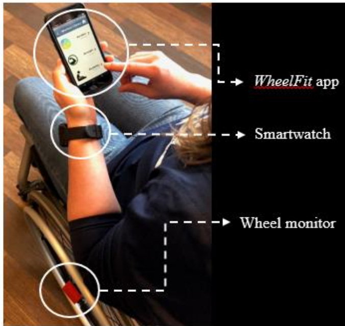
Figure 8. WheelFit consists of 3 components: 1) WheelFit app, 2) smartwatch, and 3) and the wheel monitor
