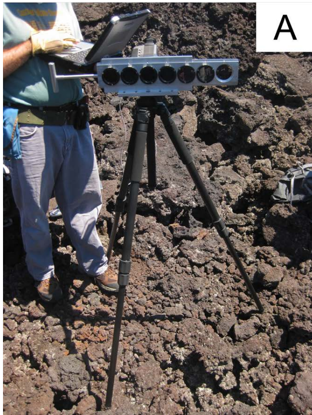
Figure 4-2 Photographs of the slider filter system (courtesy of R. Lee, SUNY Oswego).
