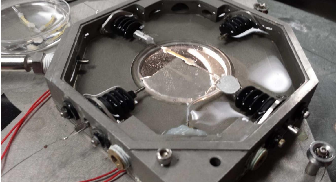
Figure 7. Gelatin/fibrinogen tubular construct loaded into the bath of the microbiaxial optomechanical device.
