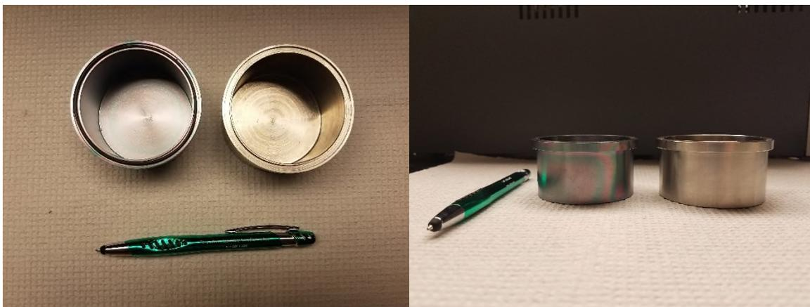
**Figure 2: Micro-chamber (114 ml) used in studying SPF SVOC emissions (top and side view)**
