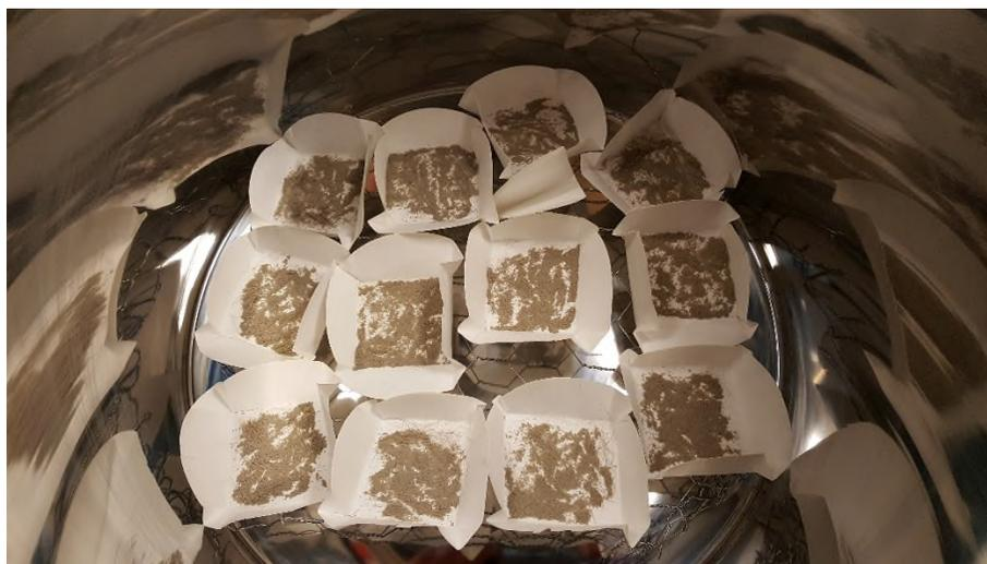
**Figure 30: Dust samples and blank filter placed in the small chamber**
