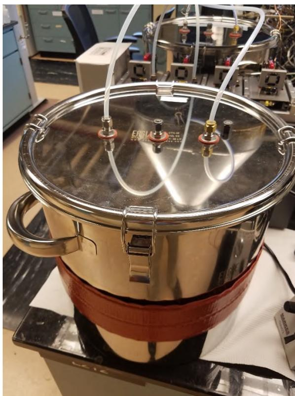
**Figure 3: Small chamber (36 liters) used in studying SPF SVOC emissions**
