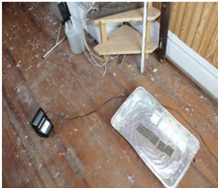
**Figure 17: TCPF accumulation samplers**
