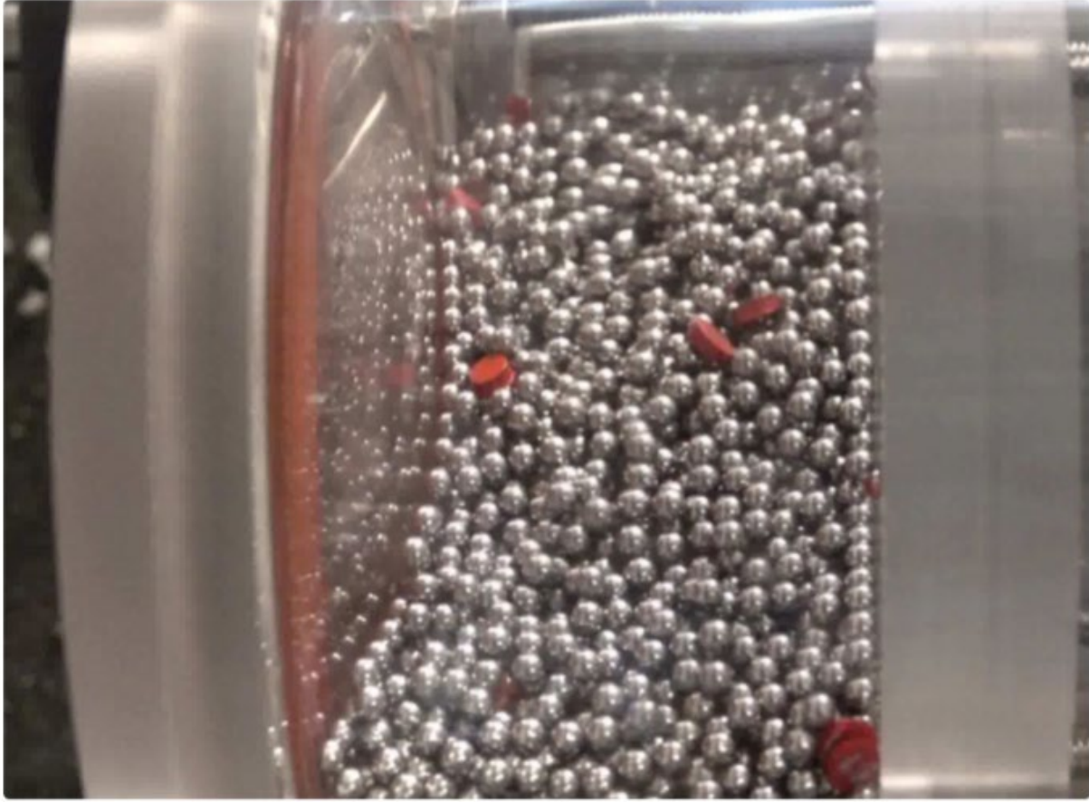
Figure 8.6: Experimental results for #7 tracer disks (as shown in Table 1) with 4.5 mm bulk spheres inside a 3-D cylinder container running at 3 RPM.
