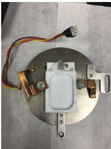
**Figure E.3.** The completely assembled stage including the Teflon cell is shown here.
