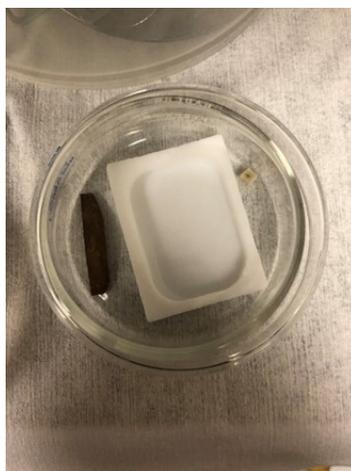
**Figure E.1.** The image shows the Teflon cell, which holds the substrates used for the break junction experiments.
