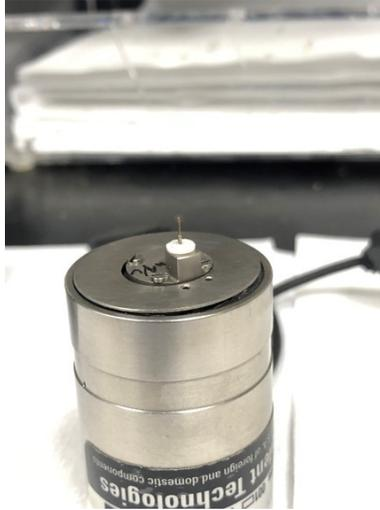
**Figure E.4.** The scanner with a gold tip inserted into the preamplifier tube is shown here.
