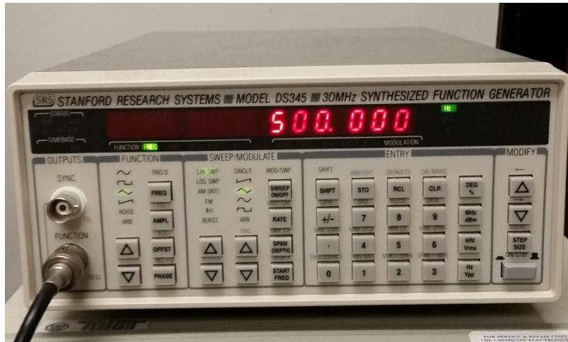
**Figure E.5.** The function generator (SRS Model DS345) used to apply the externally modulated bias is shown.
