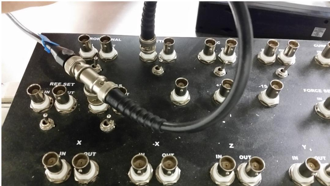
**Figure E.6.** The breakout box for the Agilent 5500 SPM system is shown. The incoming coaxial cable from the function generator is split and enters the breakout box in the “Bias In” port and the “Friction” port. For each port, there is an on/off switch; the position of the switch shown here corresponds to “off” position for both ports.
