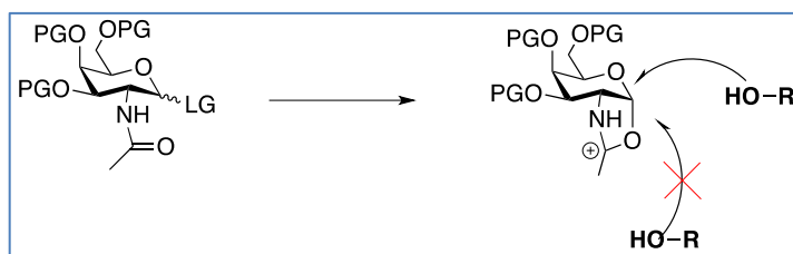
Figure 2-13 Acetyl group acting to inhibit alpha selectivity in glycosylation reaction
