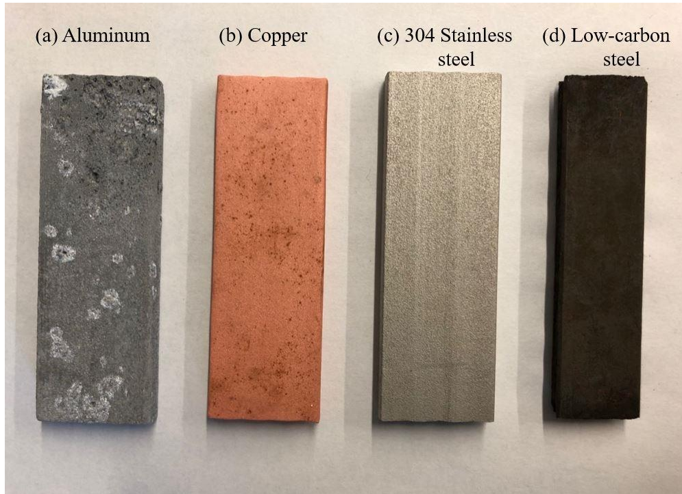
Figure 17. Corroded samples for 25 days after cleaning
