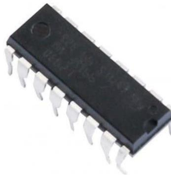
**Figure 3.4 The L293D IC chip**
