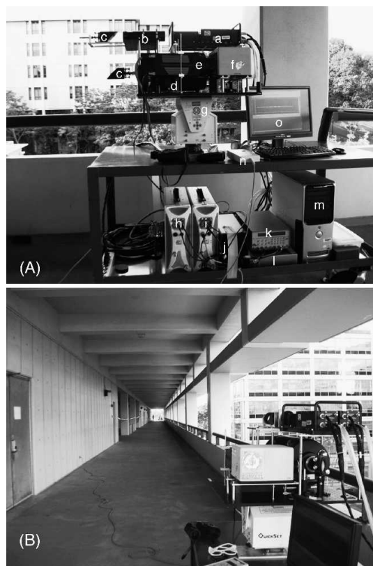
Figure 1.18 – Standoff visible Raman spectrometer constructed by Misra et al. pointed at samples 120 m away. Figure adapted from Misra et al. 24
