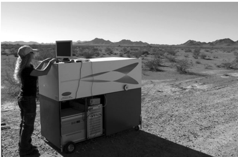
Figure 1.14 – Cart mounted standoff LIBS instrument utilized for explosive detection. A Nd:YAG laser produced 350 mJ pulses of 1064 nm light to excite samples including TNT, RDX, and C-4 placed on a car door at 30 m standoff. Figure adapted from Lopez-Moreno et al. 171
