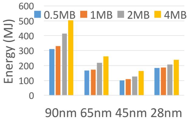
Figure 9: Manufacturing energy for four-core systems with varying LLC capacities across technology nodes.
