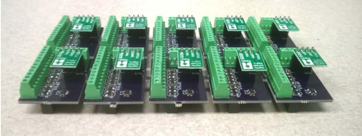
**Figure 2.2 - Custom sensor boards for TelosB motes**
