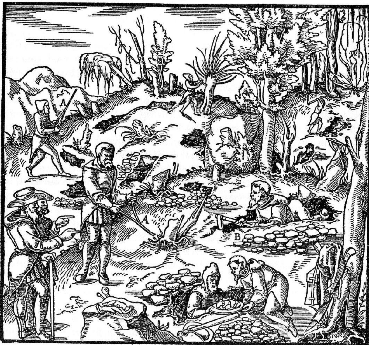
Figure 7.4 Illustration from De Re Metallica Book 2, Georgius Agricola, Erzsucher - The Prospectors. The image shows various techniques used for mining and prospecting during the XVI century, such as test pitting, recognition of areas of flora impacted with metals, and dowsing (Reproduced from Agricola 1556, Book II, page 1).
