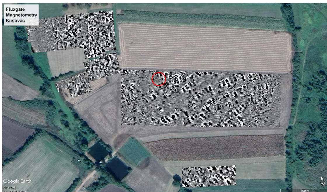
Figure 5.6 Fluxgate gradiometer surveys at the Kusovac settlement revealing enclosure ditches and other magnetic features .
