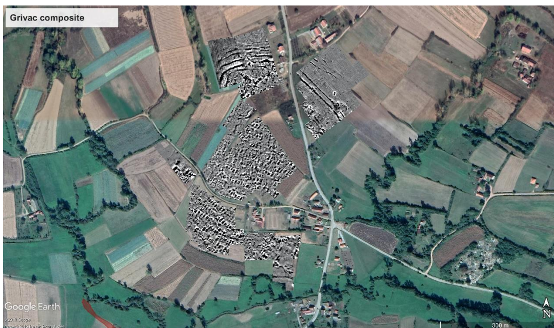
Figure 5.4 Fluxgate gradiometry surveys showing enclosure ditches and other magnetic anomalies at the Grivac settlement.
