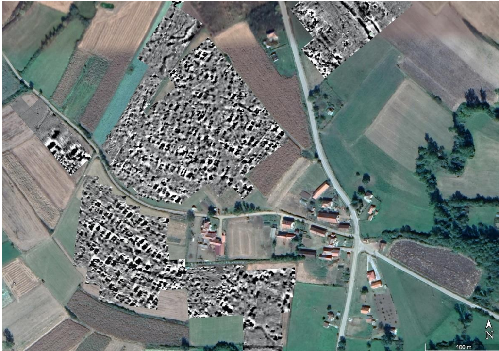
Figure 5.3 The central area of the Grivac settlement showing greyscale plots of fluxgate gradiometry surveys placed on Google Earth Satellite imagery.
