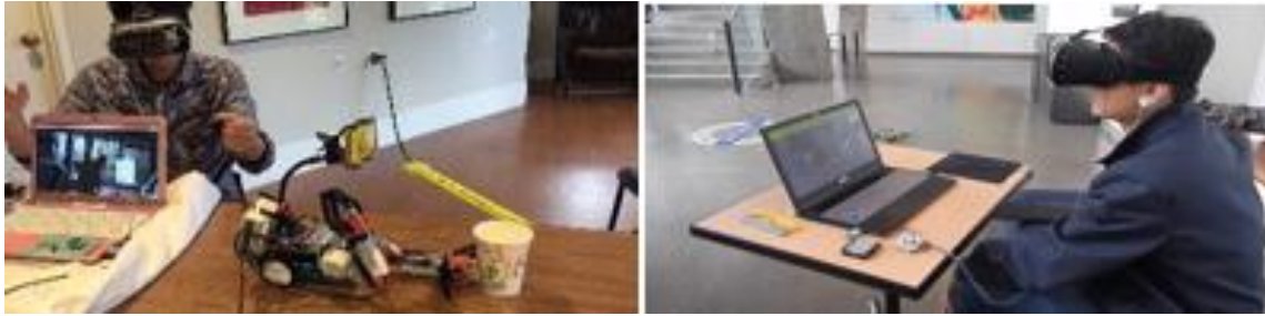
Figure 4.16. Concept of telepresence robot control by using physiological gestures. (Left) First-person's view control of a telepresence robot. The person can use hand-eye coordination to grasp a cup of water; (Right) First Person's View control of VR telepresence drone. The user can see through the drone's camera and simply use eye movement and facial gestures to navigate around.
