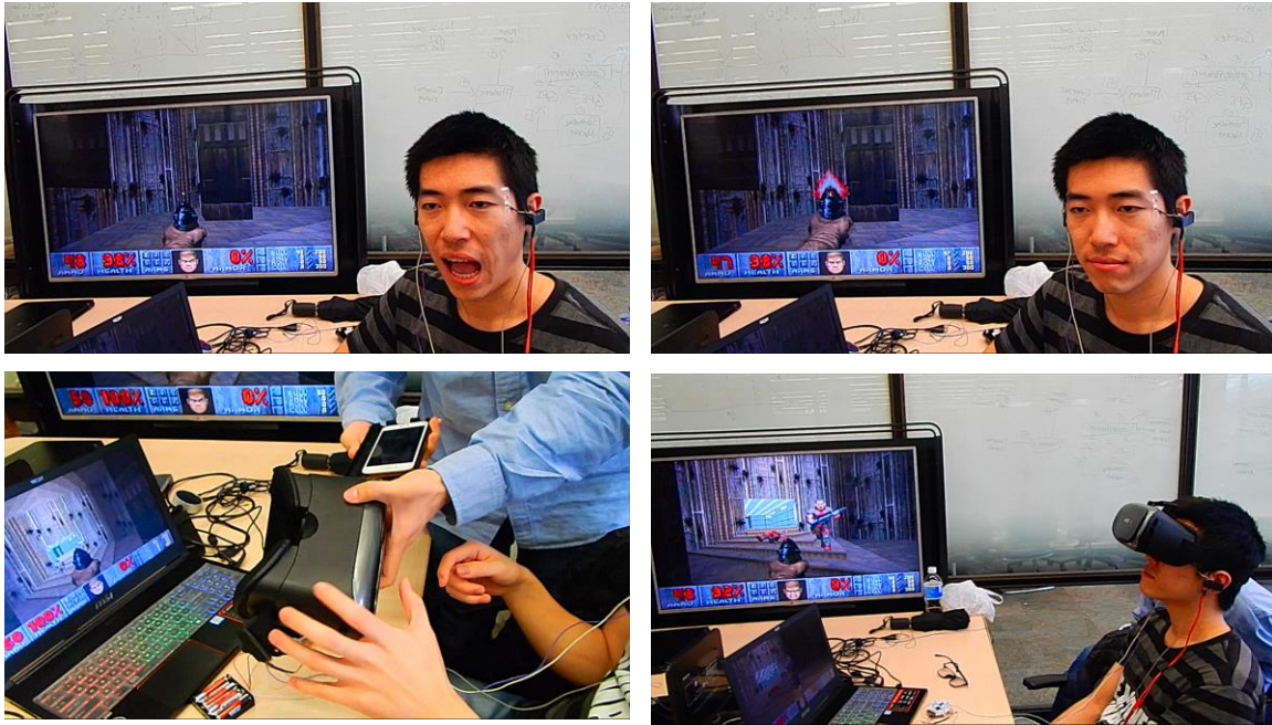
Figure 4.19. Control of 3D game for engaging and emersive experience. (Upper-left & right) Illustration of the strategy of firing a gun by open and close the mouth. (Lower-left) Our device can easily integrate with the off-the-shelf, phone-insertion-type VR headset to increase the controllability and functionality. (Lower-right) User can wear our X-interface device and VR headset seamlessly to control the VR game without conflict.
