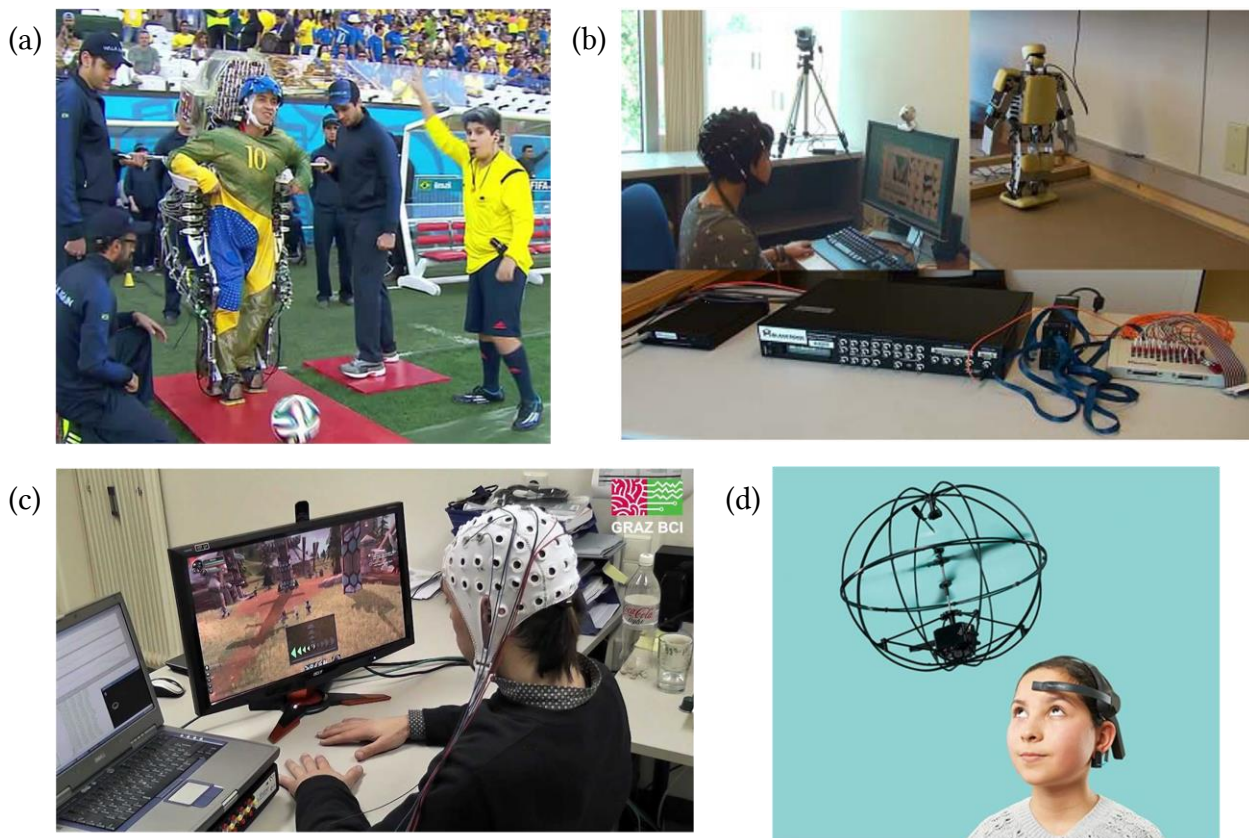
Figure 4.1. Non-invasive EEG and its state-of-the-art applications. (a) 2014 World Cup kick off by a paraplegic man with the help of a full body robotic EEG-signal-controlled exoskeleton (Developed by Duke university) [115]. (b) BCI-based humanoid robot control system [116]. (c) Graz-BCI Game Controller controlling World of Warcraft (Blizzard Inc.) just using EEG [117]. (d) Puzzlebox Orbit, a brain-controlled helicopter with the help of NeuroSky MindWave EEG headset [118].
