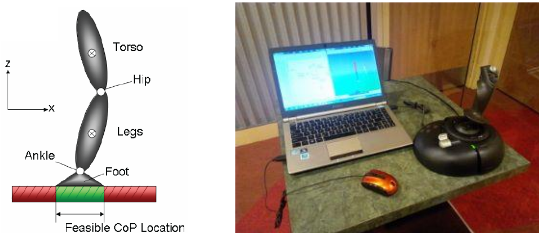
Figure 3.6. Matlab Simulink platform of double-inverted pendulum. Human can cooperate with the robot by using joystick to control the hip joint, while robot will be responsible for controlling the ankle joint.
