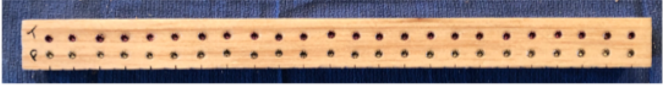
Figure 12: Balsa wood with Tapered and Parallel walled implants placed
