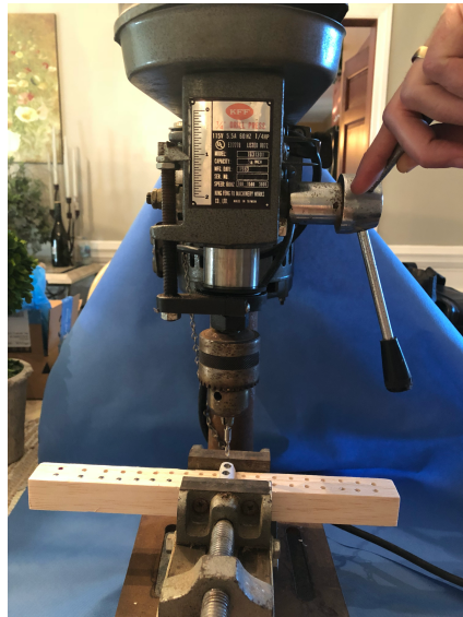
Figure 11: KFF 1/4" Drill Press with Osteotomy bur (King Feng FU Machinery, Taiwan)
