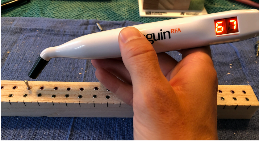
Figure 13: RFA recording using Penguin RFA Analyzer (Aseptic, Woodinville, WA)
