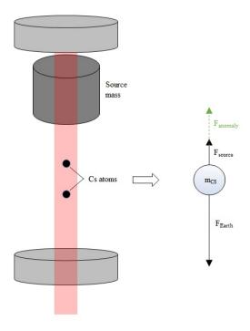
Figure 3.2: The basic set-up for a light-pulse atom interferometry experiment using Cs atoms with mass  $m_{Cs}$ . The atoms are launched into free fall, in the vicinity of a source mass mass  $m_{source}$ . While in free-fall they experience the gravitational force from the source mass  $(F_{source})$ , the gravitational force from the Earth  $(F_{Earth})$ , and potentially an anomalous fifth force  $(F_{anomaly})$ . Redrawn from Jaffe et al. 2017.
