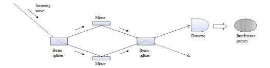
Figure 3.1: A schematic overview of the principle behind an interferometry experiment. An incoming wave is split, after which two waves follow two different paths. The waves along the two paths get reflected by mirrors, and recombined at a third point. The recombination gives rise to an interference pattern. Shifts in the interference pattern can hint at differences in path length, for example due to the stretching of spacetime by gravitational waves.
