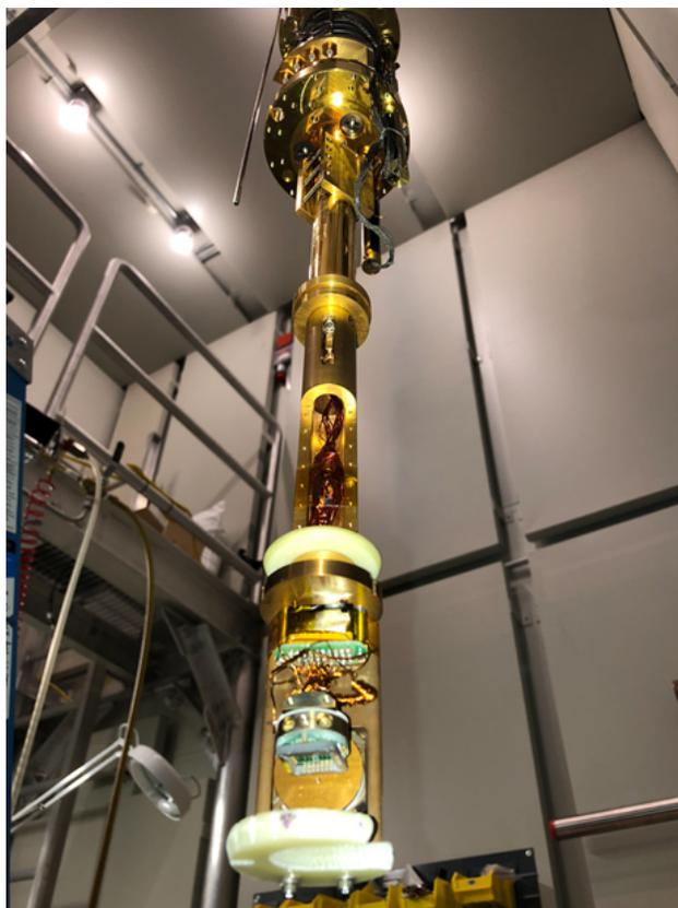
Figure 67: 2-axis rotator on Leiden MNK dilution insert. The 2-axis rotation allows the magnetic field of up to 20 T to be applied in any orientation relative to the sample.
