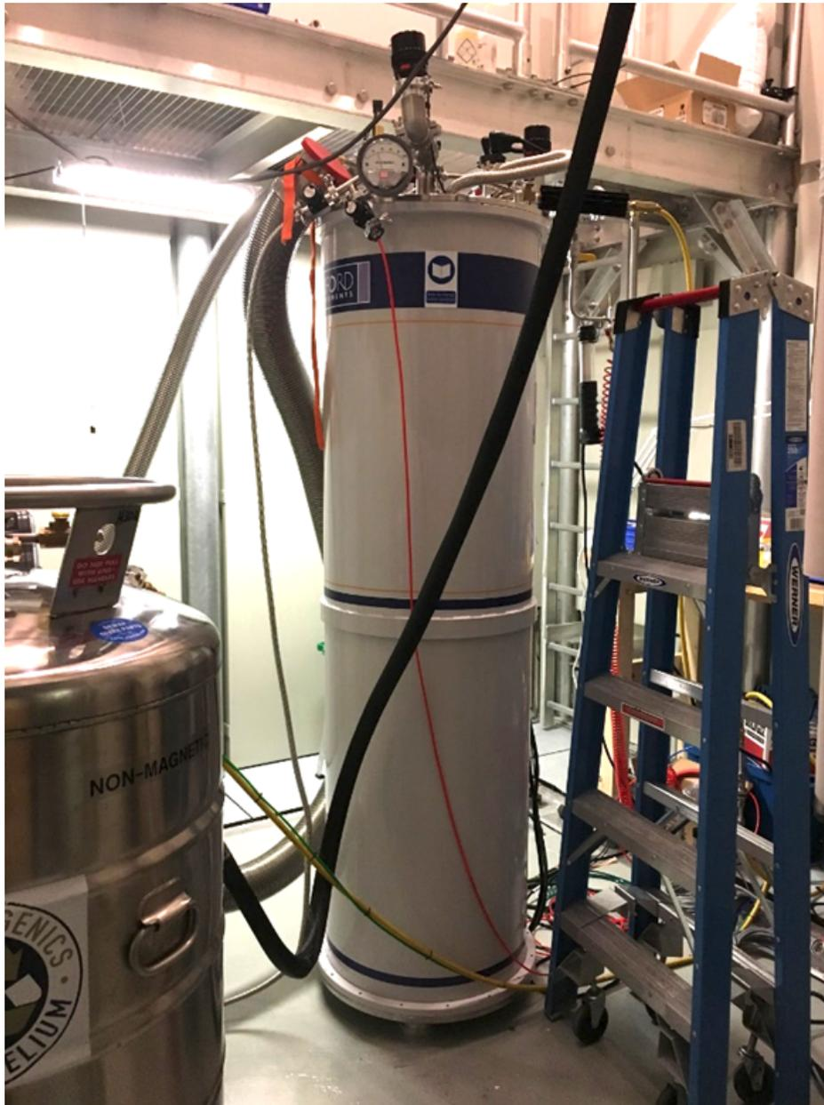
Figure 62:  $^4\text{He}$  cryostat with 18/20 T superconducting magnet for the Leiden MNK dilution refrigerator insert.
