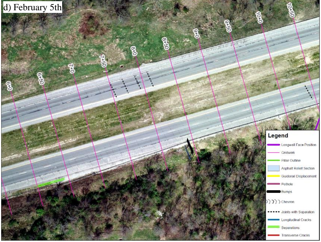
Appendix Figure 2 Damage observed on highway on February 5 th
