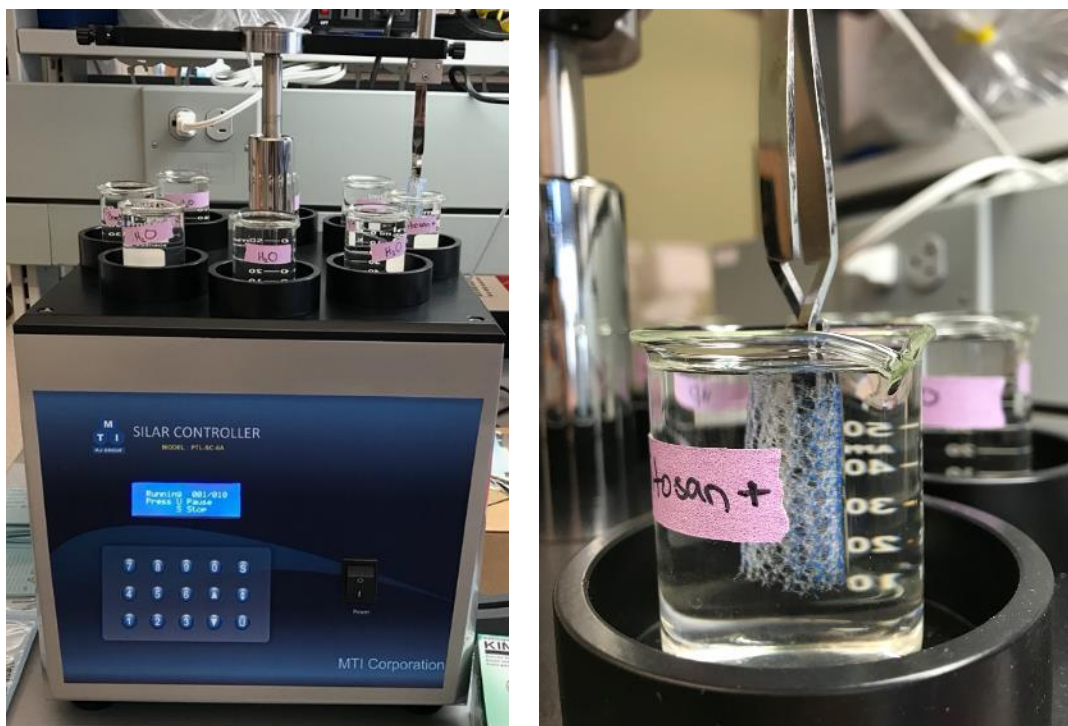
Figure 34: MTI SILAR Automated Dip Coating machine used for layer-by-layer coating
