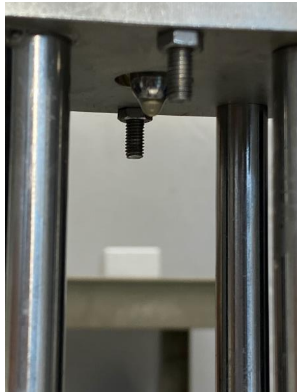
Figure 13: Instron Set up for Ball Burst Testing
