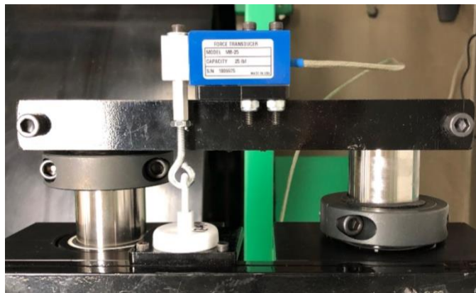
Appendix Figure 5 Load Cell Attached to Air Bushings with Magnet
