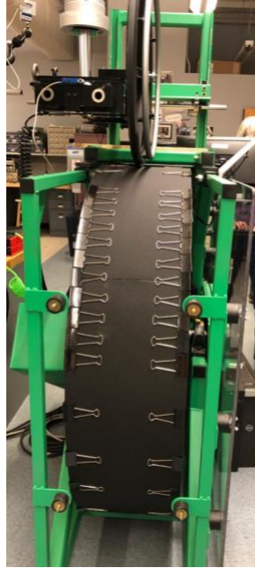
Appendix Figure 8 Treadmill Belt Material on the Drum
