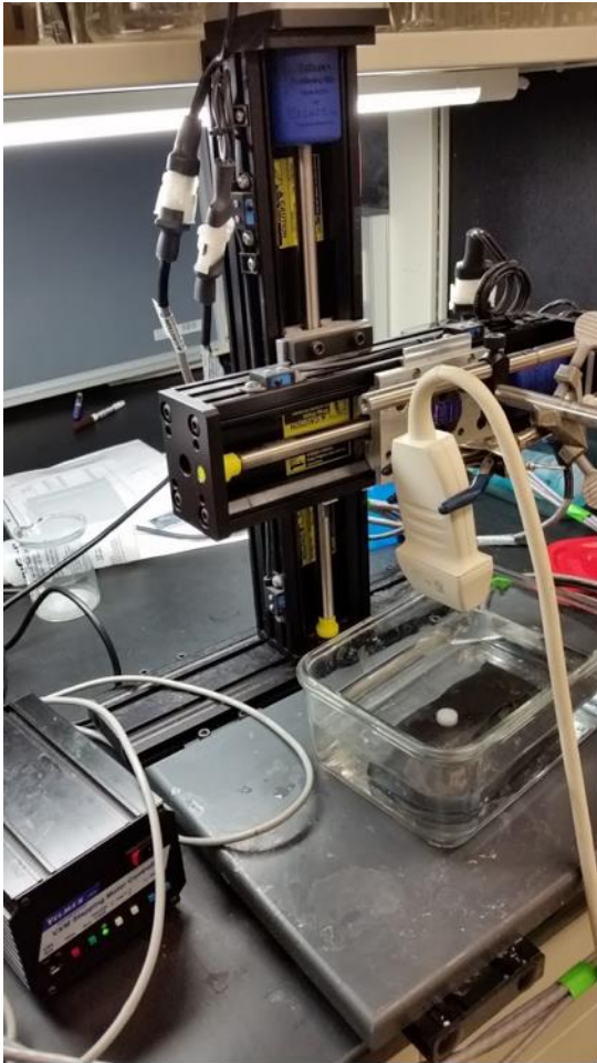
Appendix Figure 15 Ultrasound Elastography Experimental Setup
