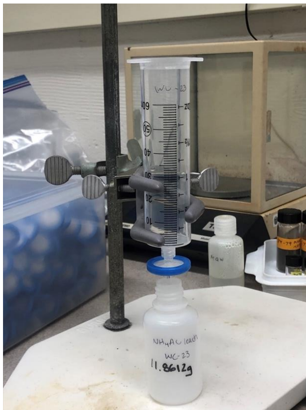
Figure 15. A 60 ml poly syringe with an attached filter held up with a ring stand above a 60 ml poly sample bottle of previously recorded mass (author's photo).
