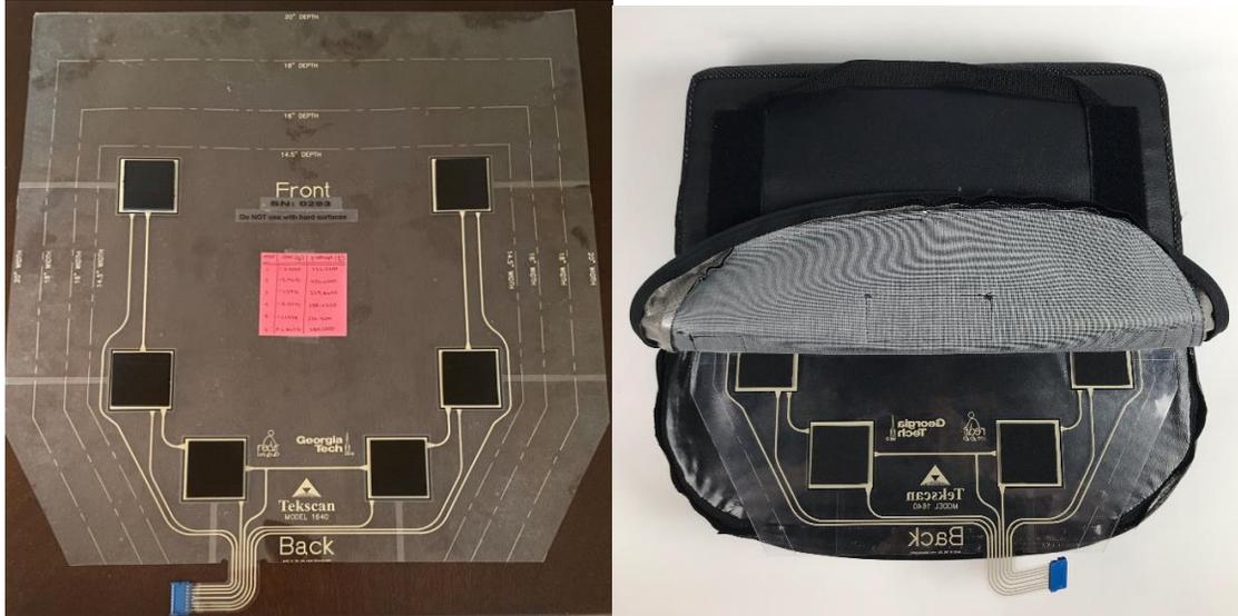
**Figure 1. Tekscan Mat Equipped with Force Sensors**
