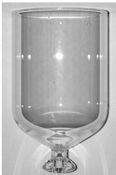
Figure 30. Electrochemical cell used for EIS measurements.
