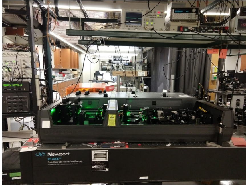
Figure 3 Photo of the regenerative Ti:sapphire laser system during maintenance, including the pump laser diode (back), oscillator (middle), and amplifier (front).
