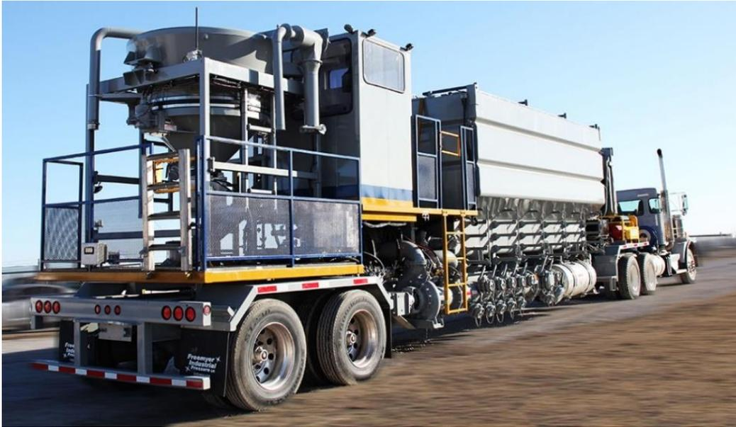
Figure 6 A trailer, engine, hydraulic system, open top hydration tank, image by: <http://indpress.com>.
