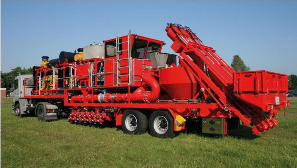
*Figure 8 Blender, image by: <https://www.goes-well.com/frac-equipment/>.*
