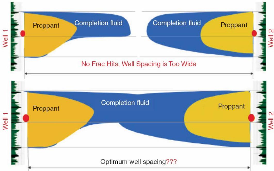
Figure 20 The top figure illustrates that if frac hits are not observed it may mean that an operator is leaving a portion of the reservoir untapped. A happy medium is shown in the bottom, in which a frac hit might take place but because it mainly involved fluids and not proppant, negative communication will be short-lived as any unpropped fractures close. Source: Shell (Jacobs 2017).
