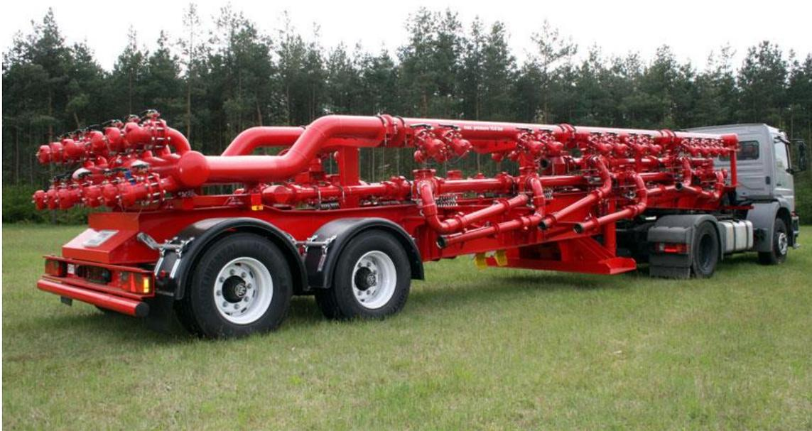
Figure 9 Manifold trailer, image by: [https://www.goes-well.com/frac-equipment/#Anker\\_Iron\\_Handling\\_Equipment](https://www.goes-well.com/frac-equipment/#Anker_Iron_Handling_Equipment).
