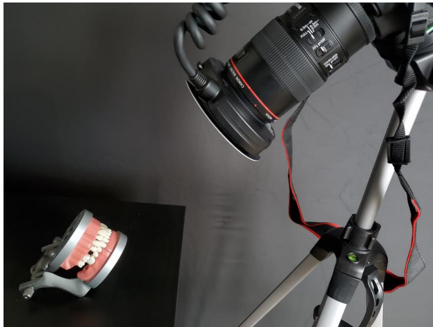
Figure 9: Camera Mounted on Tripod with a Fixed Lens-to-Object Distance
