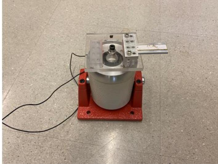
**Figure 3.5 Vibrator with the sensor installed**
