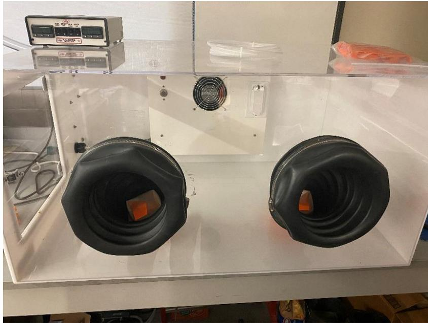
**Figure 3.4 Chamber with temperature control panel**
