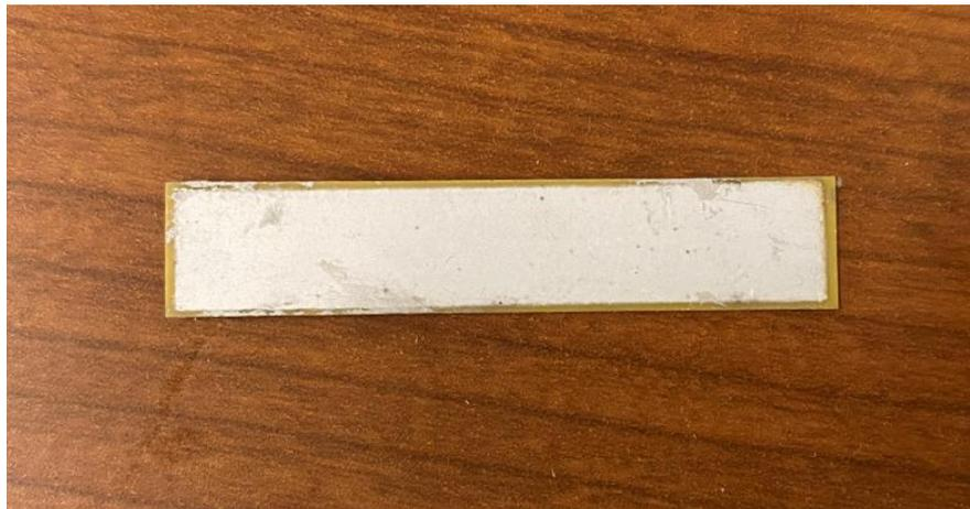
Figure 3.1 PZT element used in the sensor
